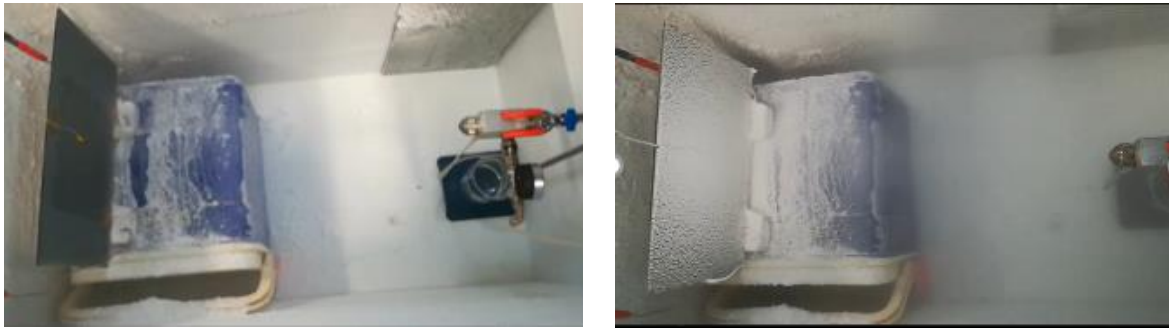
Figure 5.11: Ice accretion of the surface of the heating panel by a spray-gun system made by CNR-ISAC.
