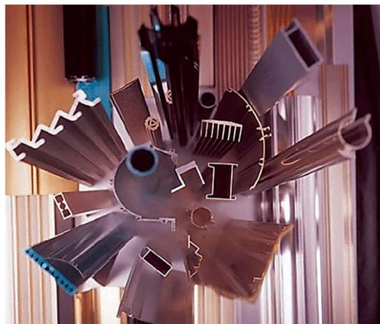
**Fig. 1.3:** Examples of profiles achievable with the hot extrusion process [3].
