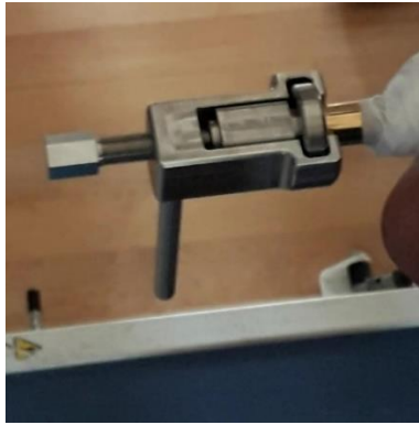
Figure 19 - Insert the extractor around the male connector
