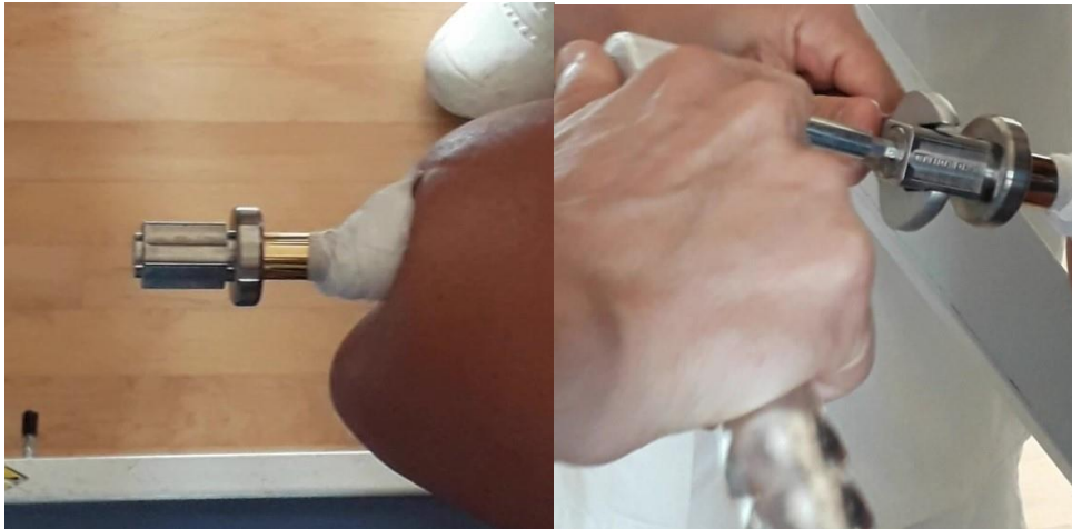
Figures 14 (a e b) – Screwing of the male connector
