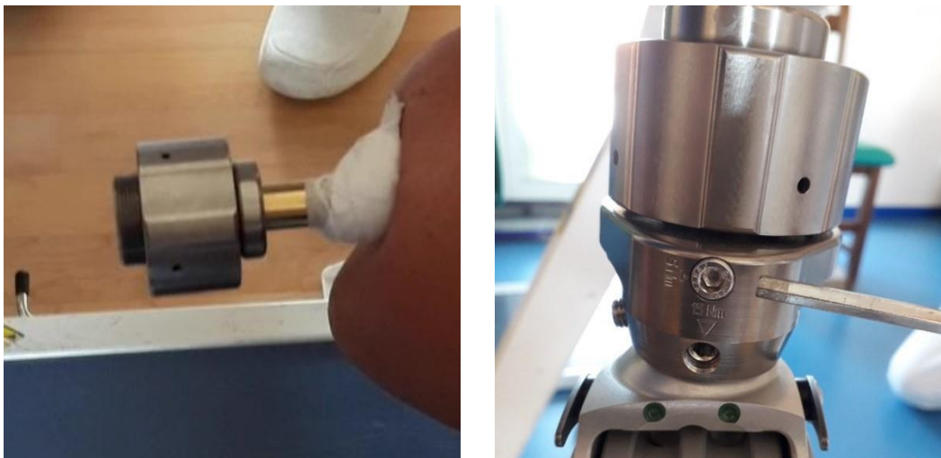
Figures 15 and 16 – Insert the female connector and M5 screw (right)
