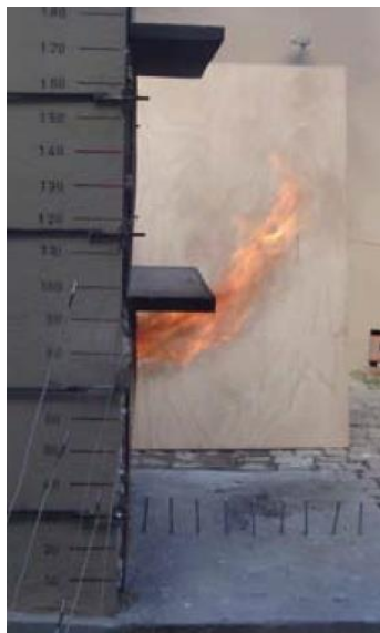
Picture 68: Laboratory test of the external vertical subdivision.
