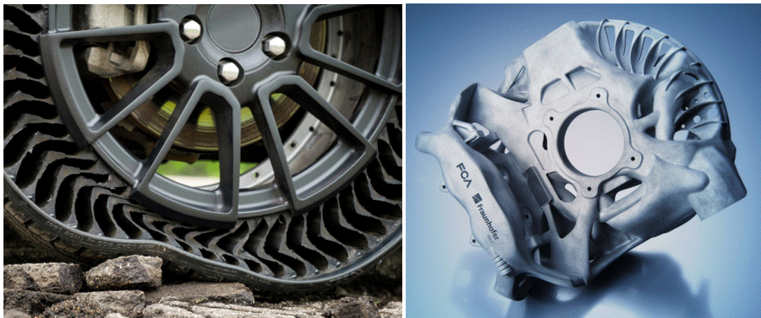
Figure 17: The Michelin's Uptis and the integrated wheel carrier from FCA
