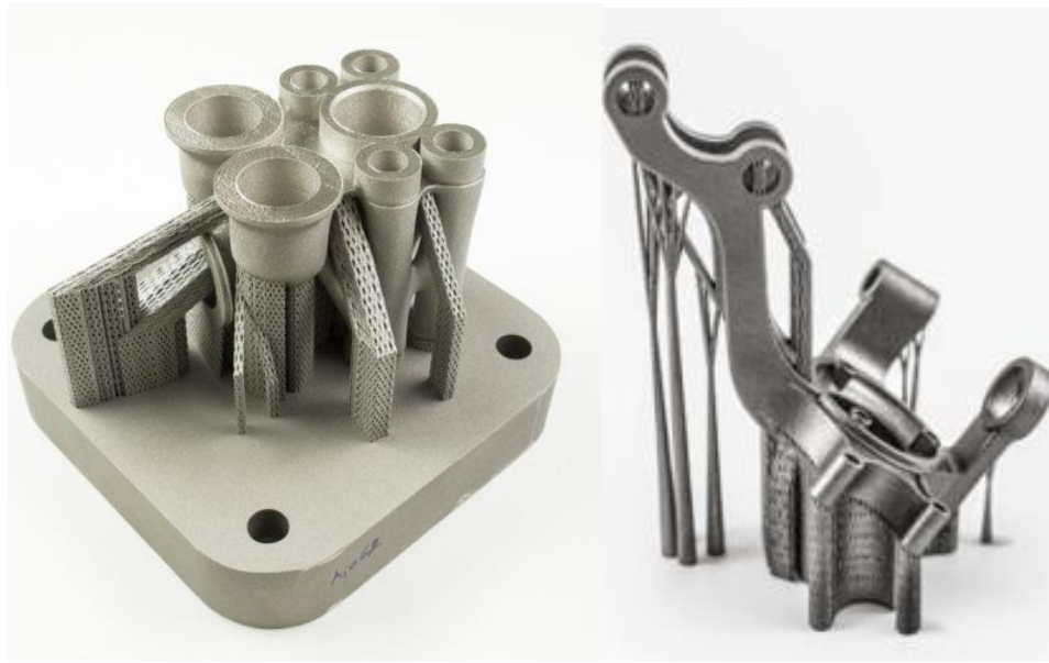
Figure 15: An industrialized build job for L-PBF process.
