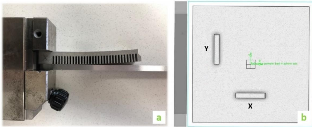
Figure 29: Deformed X specimen from 1 st test after removal (a) and 3D printing job layout from 2 nd test (b)
