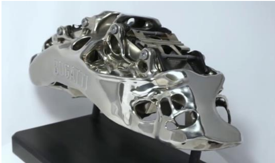
Figure 20: Bugatti's titanium brake caliper
