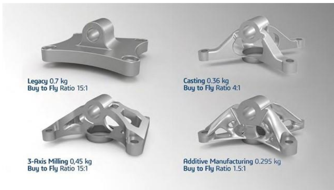
Figure 14: The effect of process constraints on topology optimization
