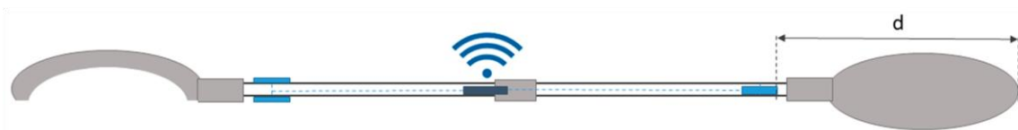
Figure 3. Block scheme of the paddle slave node (where d is the distance of the strain gauge sensor from the tip blade).
