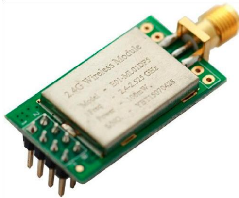
Figure 3. The nRF24L01P+PA+LNA module.
