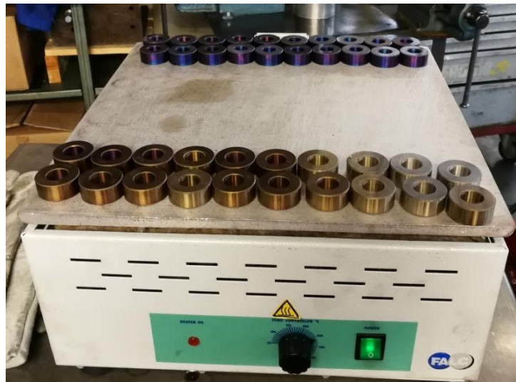
Figure 44: Heated plate used to heat shrink fitted hubs.
