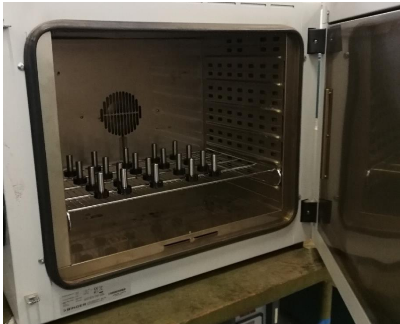
Figure 46: Oven used to heat samples for high temperature tests
