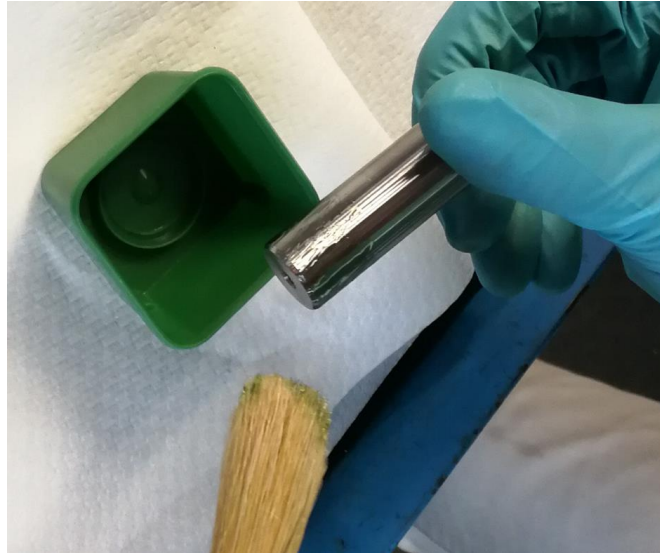
Figure 45: Adhesive applied to cleaned shafts with a little brush
