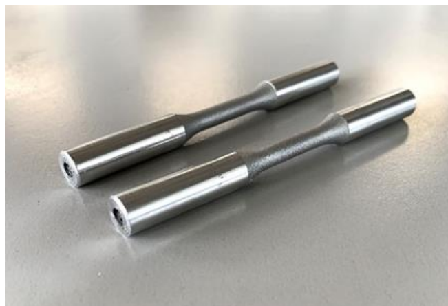
Figure 72: AlSi10Mg slanted oriented samples, after head machining
