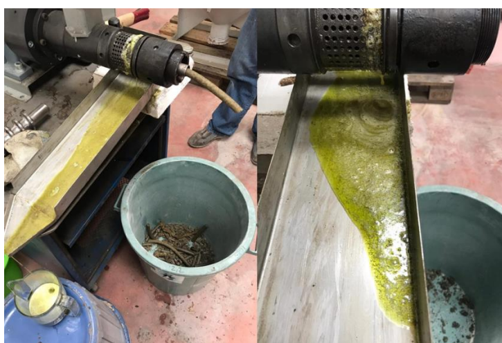
Figure 3.4.2.1.1 Extraction of hemp seed oil by cold-pressing.
