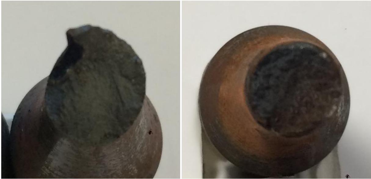
Fig. 3.2.18 Appearance of the fracture surface; a) specimen from ausformed 3229 alloy broken after LCF test; b) specimen from the same alloy broken after CF test (200s Hold Time)
