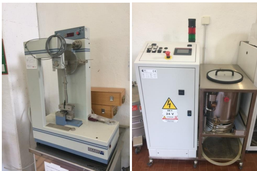
Figure 2.2.6. a) 60J capacity pendulum (CEAST) installed at ENEA Brasimone b) Conditioning device for the cryogenic temperatures
