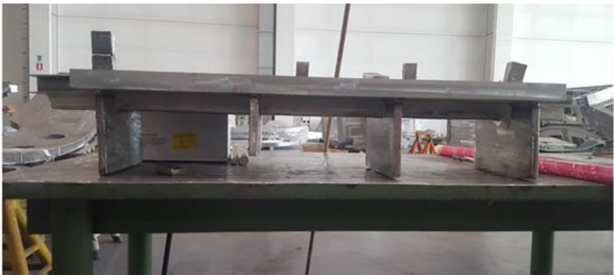
Figure 3.1.2. Additional welded plates added by the manufacturer to avoid distortion during the fabrication of the main weld
