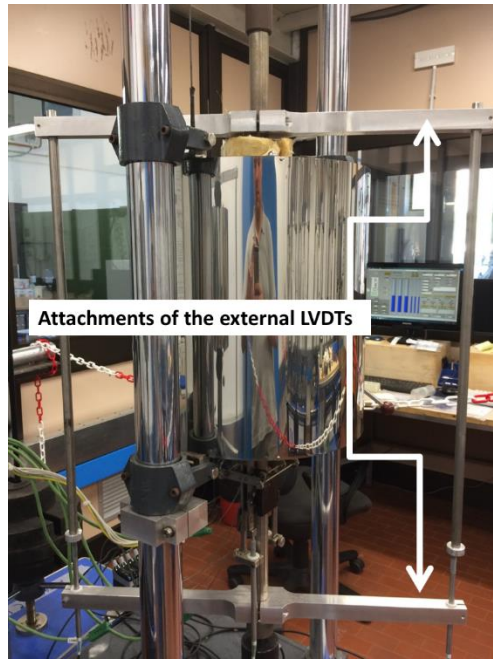
Figure 2.1.15. Detail of the assembling of the external LVDTs
