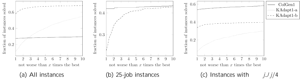
Figure 4.4: Performance profiles Dolan and Moré [2002] for different sets of instances. Each curve is associated with one method, and shows the fraction of instances it solves not slower than the value of the abscissa times the time required for the fastest approach
