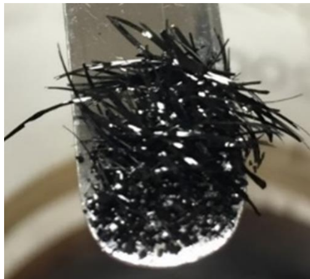
Figure 7: sample Heat24, obtained by heating after 24 hours from the melanin formation reaction in sample PDA-TiO 2 @Pluronic F-127.
