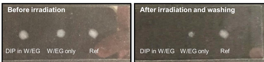
Figure 6: spots deposited on a glass slide before and after irradiation and washing. “DIP” and “W/EG” spots are covered respectively with 10 \mu\text{L} of DIP 0.04M solution in water/ethylene glycol 40:60 and with 10 \mu\text{L} of water/ethylene glycol 40:60. “Ref” spots aren’t covered with any solution during the irradiation and aren’t washed after irradiation.
