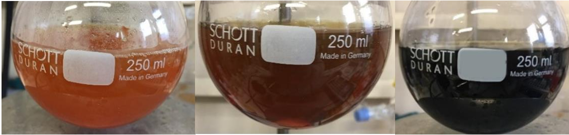
Figure 6: Melanin formation steps in PDA-TiO 2 @Pluronic F-127
