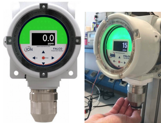
(a) PID commercial sensor. (b) PID sensor during preliminary tests.
