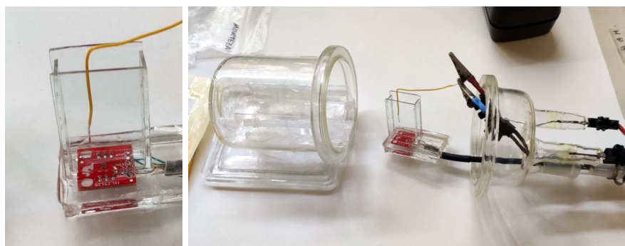
(a) Assembled "tumbler" with colorimetric sensor at base.
