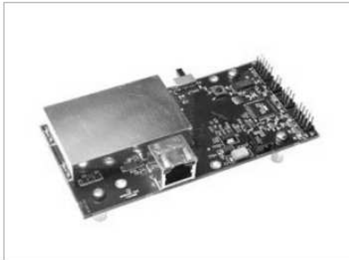
Figure 4.4: Coordinator board MIB600
