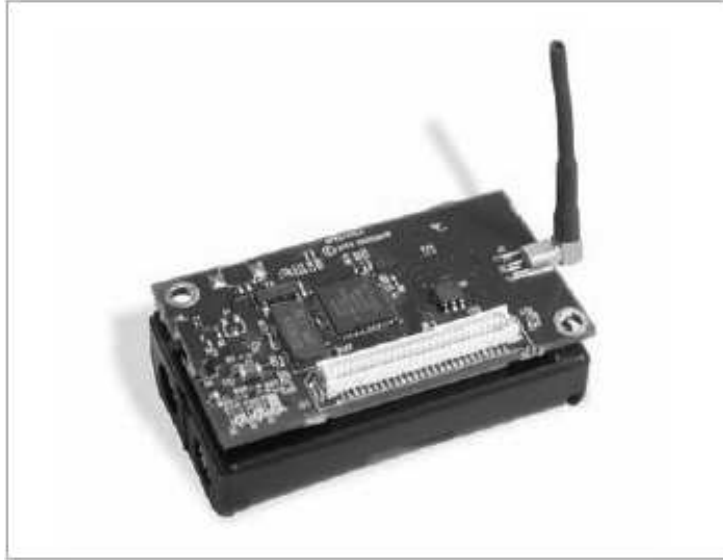
Figure 4.3: Radio board MicaZ
