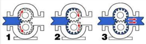
External gear pump operation [112].
