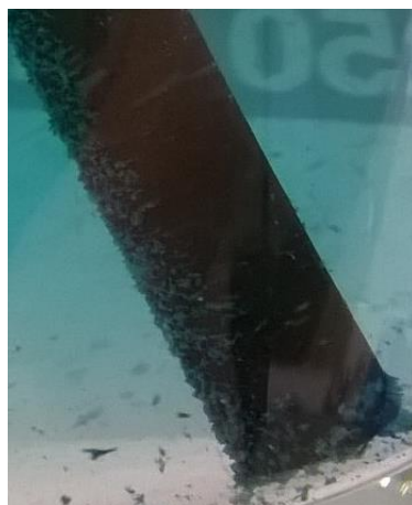
Fig. 9.7. Picture of the anodic chamber showing cells on the surface of the clean electrode at the end of the experiment.
