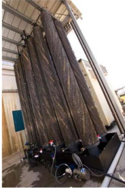
Fig. 3.2. Tubular microbial fuel cells tested for power production using wastewater produced at Foster's brewery in Yatala, Australia ( www.microbialfuelcell.org ).
