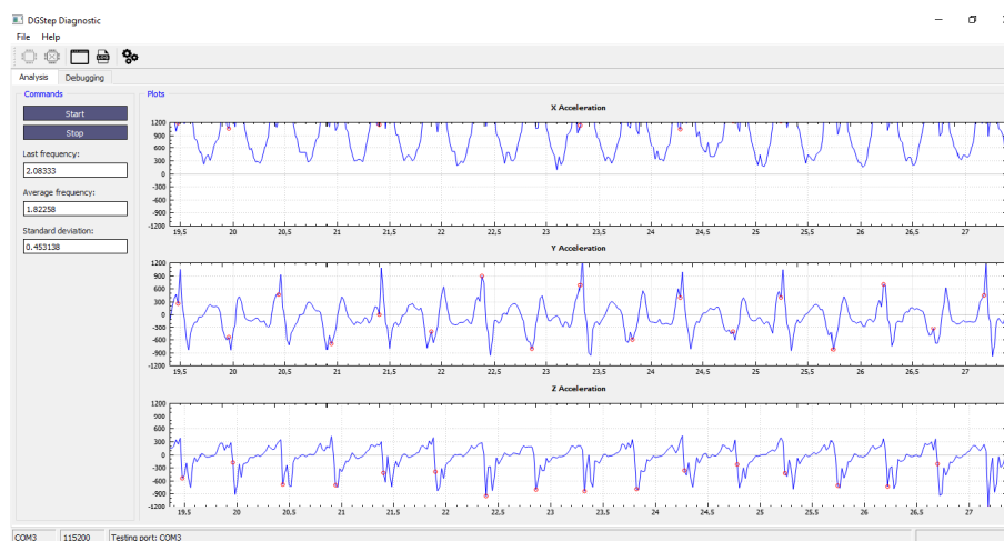
Figure 2.15: DGStep Diagnostic tool. Foot contact events detected in real-time are marked with red dots. Step frequency extracted from the last 10 steps (Last Frequency) and the average value since the beginning of the trial (with the correspondent standard deviation) are reported in the boxes on the left. Time is reported in [s], accelerations in [mm/s 2 ], step frequency in [Hz].
