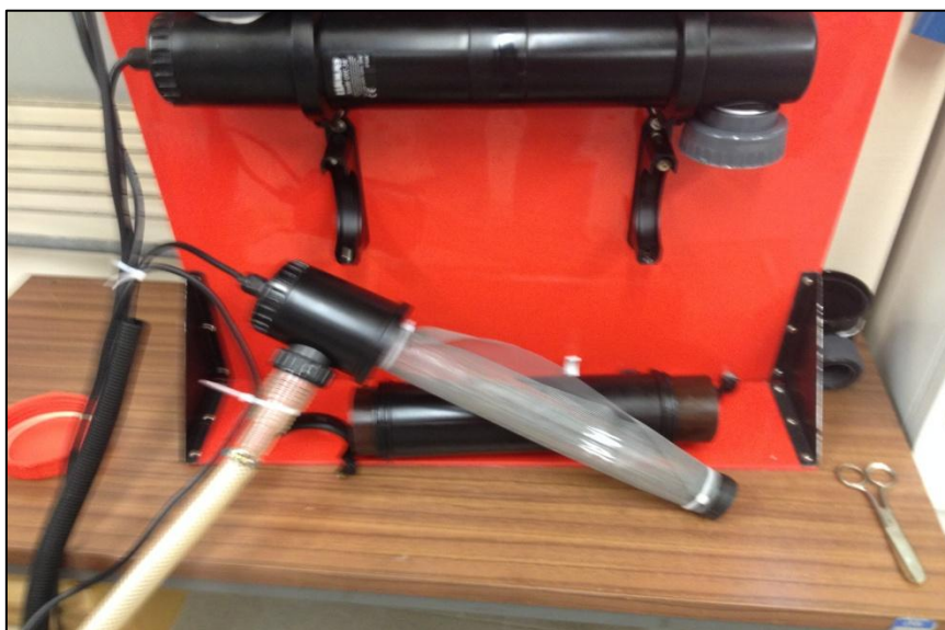
Figure 4.5 UV lamp covered with the TiO 2 net of fiberglass
