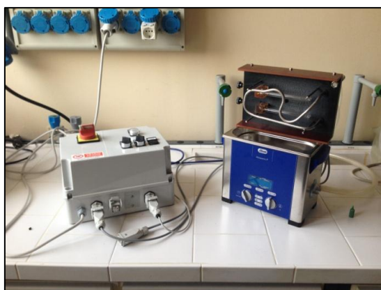
Figure 4.7 Apparatus for the ultrasounds / UVC - \text{TiO}_2 hybrid technique.
