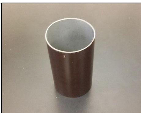
Figure 4.4 Tube with TiO 2 on the inner layer
