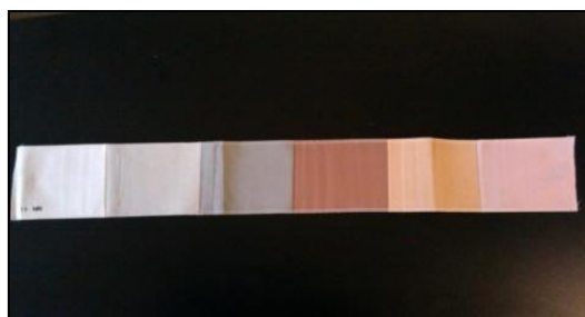
Figure 4.6 Standard strip used during the laundry machine washing cycle.
