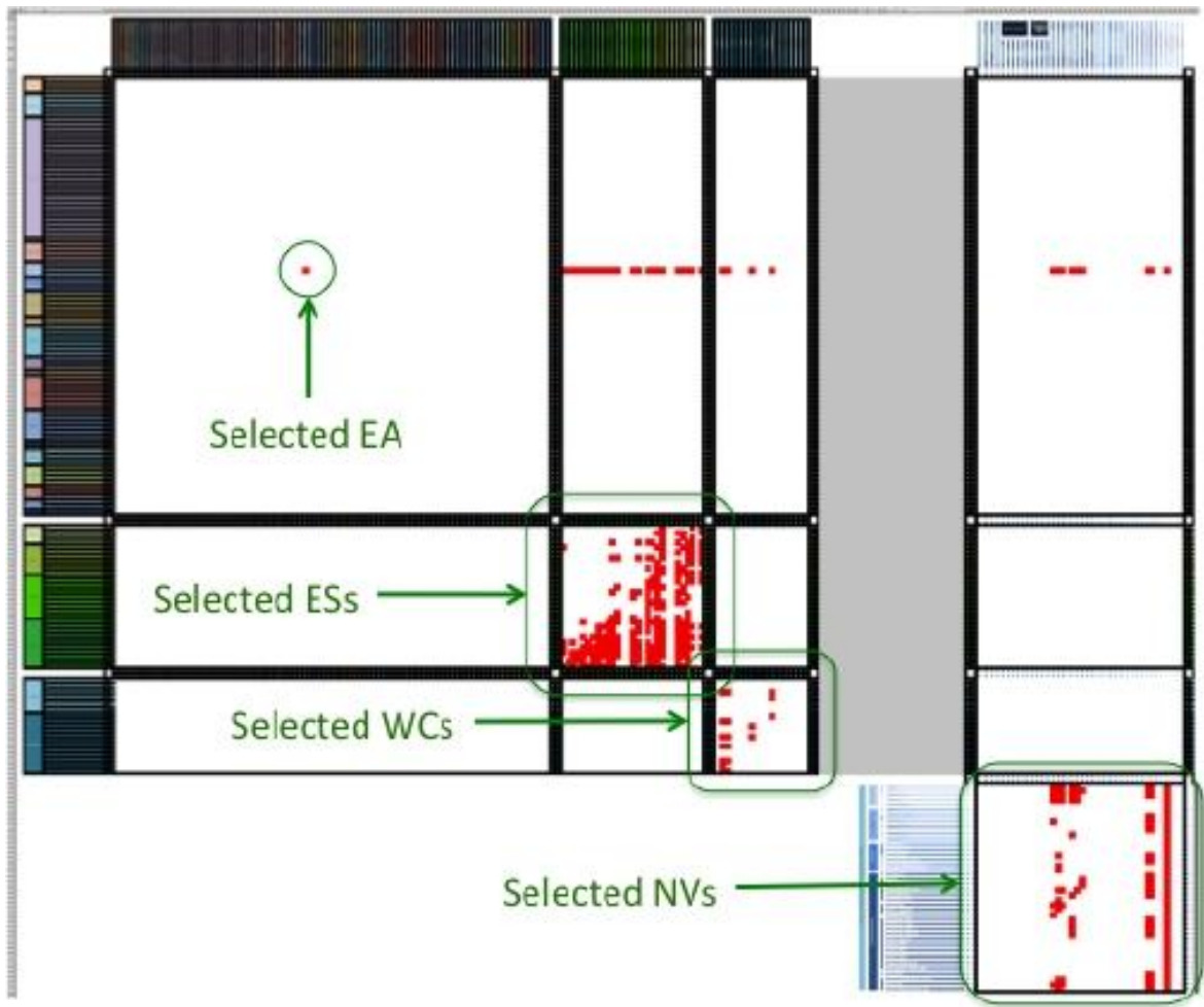
Figure 41 - The output from the PoChASSy42 Excel tool applied to the case of a bridge with pylons described in section 3.4. The red cells are the ESs, WCs and NVs connected to the starting Economic Activity derived from the 1 st order path: EA → ES/WC/NV.
