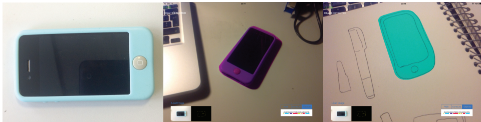
Figure 4.17: Moments invariants allow to compare objects under rotation, scale, translation and slight perspective transformations, while shape matching is enough robust to match different representation of the same object. In the example, a smartphone is detected in different orientation and also when is hand drawn.
