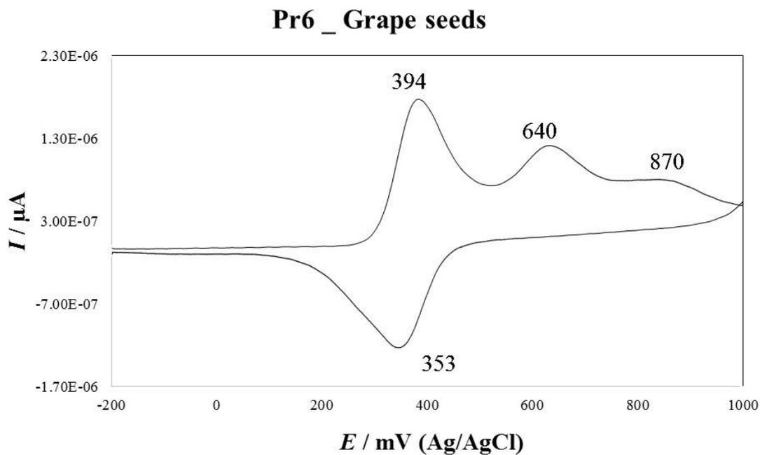
**Figure 6.2.** Cyclic voltammograms (background subtracted) of a grape seed tannin (sample Pr6) in model wine solution, measured at  $100 \text{ mV s}^{-1}$  above the potential range: -200 to 1000 mV, at a 3 mm glassy carbon electrode.
