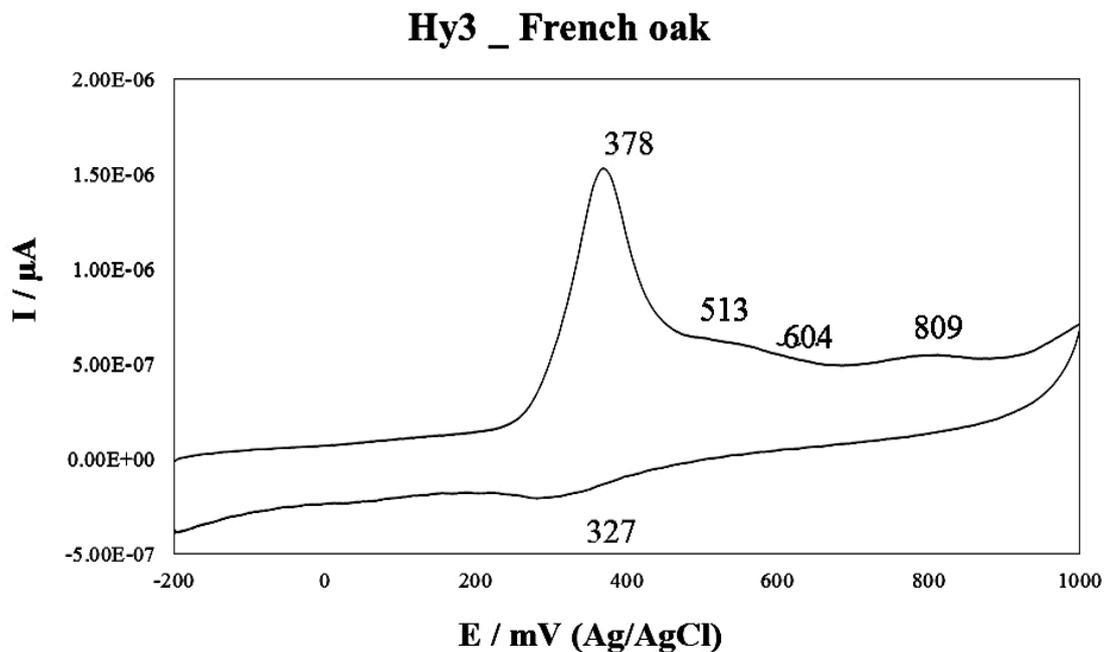
**Figure 6.1.** Cyclic voltammograms (background subtracted) of a French oak tannin (sample Hy3) in model wine solution, measured at  $100 \text{ mV s}^{-1}$  above the potential range: -200 to 1000 mV, at a 3 mm glassy carbon electrode.
