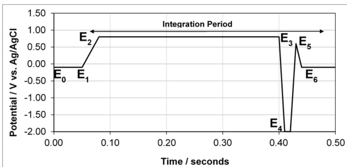
**Figure 5.3.** Integrated amperometry waveform used to determine the antioxidant activity of phenolic compounds in wines and model wine solutions. Detector response is the charge from integration of the phenolics oxidation current between 0.20 and 0.50 s, expressed as nC.
