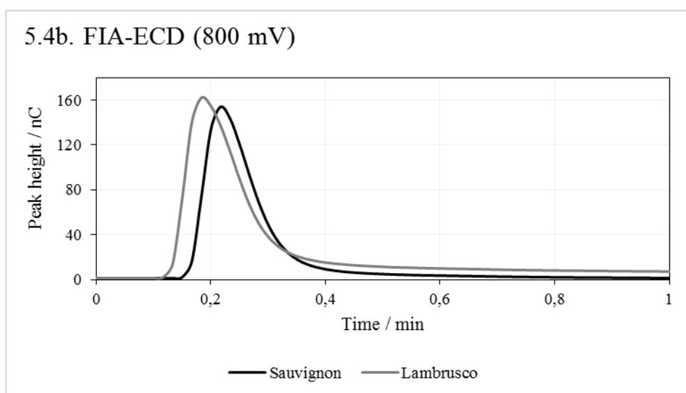
**Figure 5.4.** FIA-DAD (5.4a) and FIA-ECD (5.4b) experiments performed on a white wine (Sauvignon Blanc) and a red wine (Lambrusco). The same injection was used for subsequent analyses, following re-equilibration of both detection systems. Peak areas were then calculated to calibrate the response in  $\text{mmol GAE L}^{-1}$ .
