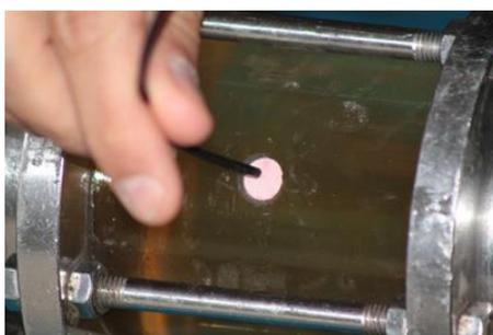
**Figure 3.3.** Measuring the DO through the glass of the specula using the PSt3 sensor (Nomacork, France).
