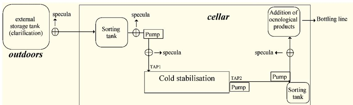
**Figure 3.8.** Disposition of facilities in cellar and identification of the sampling points.
