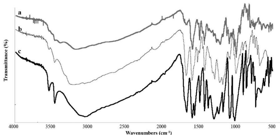
Fig. 3. ATR FT-IR spectra of the most common monomeric units of tannins. (a) (+)-catechin; (b) gallic acid; (c) ellagic acid.
