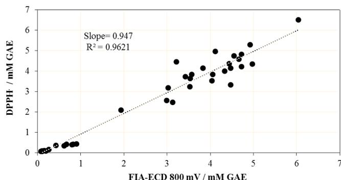
**Figure 5.5.** Linear regression between the FIA-ECD results and the DPPH• spectrophotometric assay to determine the antioxidant activity for the proposed series of wines and oenological tannins. Results were expressed in mM gallic acid / L for both analyses.
