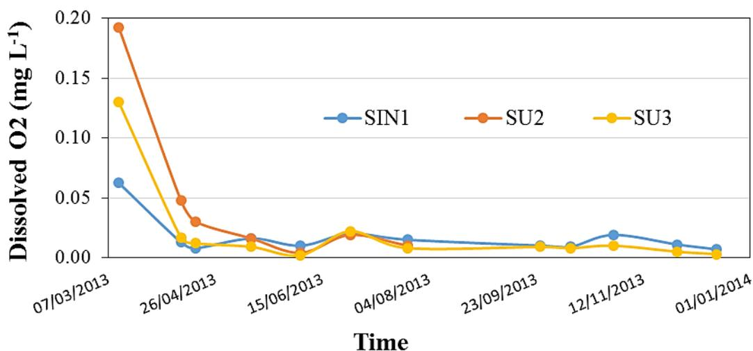
**Figure 4.6.** Time course of dissolved  $\text{O}_2$  parameters in the three bottled series. The SIN 1 sample has a less noticeable percentage decrease (-88%) related with a lower content in oxygen at bottling.
