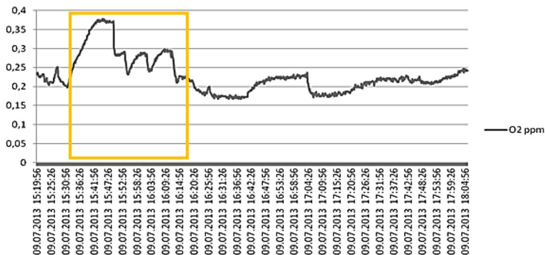
**Figure 3.5.** Time course of DO in the tank during the production process, measured in the specula with the fluorescent dot.
