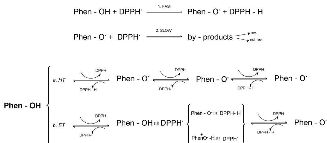
**Figure 5.6.** Electron transfer (ET) and Hydrogen transfer (HT) mechanisms occurring during the DPPH assay.
