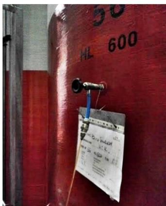
**Figure 3.2.** Attachment to tap for sampling using the QboxQC oxygen meter (Anton Paar, Austria)
