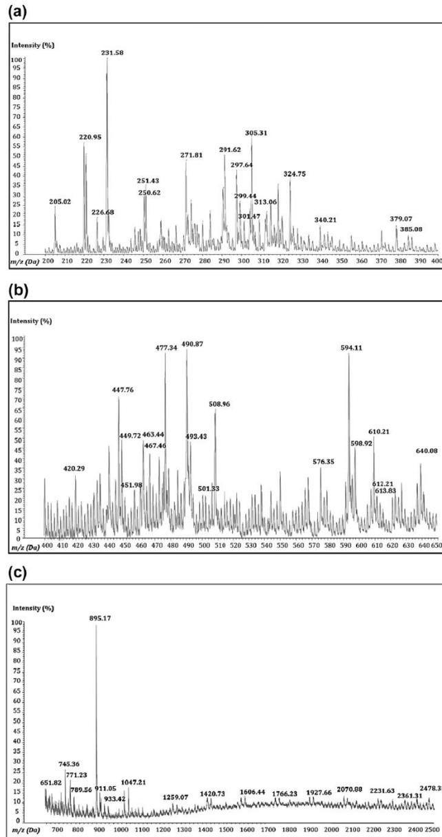
Fig. 2. MALDI-TOF spectra recorded in linear positive mode. (a) range 200–400 Da, ion gate off; (b) range 400–650 Da, ion gate off; (c) range 650–2500 Da, ion gate 400 Da. The most significant peaks are highlighted in the figures; a detailed description is provided in Table 2.
