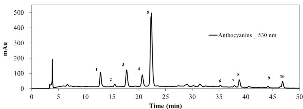
**Figure 5.1.** HPLC-DAD anthocyanins profile of a Vranec wine, following 9 days of maceration. Peaks: delphinidin-3-glucoside, (1); cyanidin-3-glucoside, (2); petunidin-3-glucoside, (3); peonidin-3-glucoside, (4); malvidin-3-glucoside, (5); petunidin-(6 acetyl)-3-glucoside, (6); peonidin-(6 acetyl)-3-glucoside, (7); malvidin-(6 acetyl)-3-glucoside, (8); peonidin-coumaroyl-glucoside, (9); malvidin-coumaroyl-glucoside, (10).
