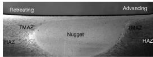
Figure 4.7. Representative macrostructure of FSP processed zone, characterized by the presence of the nugget zone, at the weld center, thermo-mechanically affected zone (TMAZ), heat affected zone (HAZ) and base materials (BM). Retreating and Advancing side are defined on the basis of relative rotating and linear motion direction of the pin [111] .
