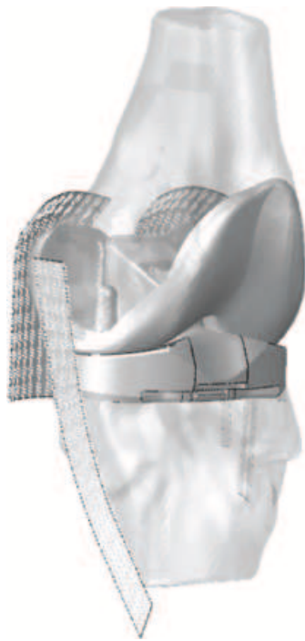
Figure 4.3: Finite element model of the tibiofemoral joint with posterior-stabilized implant and soft-tissue constraint.
