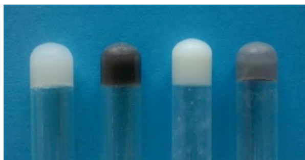
Figure 85. Photographs of hydrogels A-D prepared with Fmoc-L-Phe-D-pGlu-OH at different concentration. From left to right: A , 1% gelator/water; B , 1% gelator/GO/water; C , 2% gelator/water; D , 2% gelator/GO/water.
