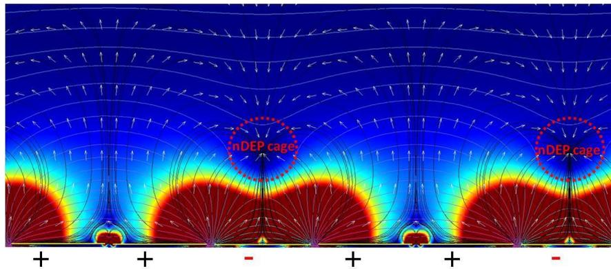
**FIGURE 3 nDEP CAGES:** NEGATIVE DIELECTROPHORESIS CAN CREATE A "CAGE" WHERE CELLS CAN BE TRAPPED ALLOWING THEIR HANDLING
