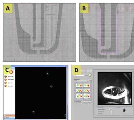
**FIGURE 5 CELL DIRECTOR.** GRAPHIC INTERFACE WHERE IT IS HIGHLIGHTED THE PATHS THAT CELLS WILL HAVE TO GO THROUGH TO REACH THE PARKING CHAMBER (A) AND THE EXIT CHAMBER (B). CAMERA LIVE SOFTWARE ALLOWING TO MONITOR IN-STREAMING CELLS MOVEMENTS (C). RECOVERY OF THE CELLS
