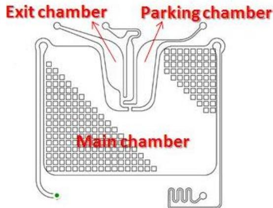
**FIGURE 2 ACTIVE AREA OF THE CHIP.** THE MAIN CHAMBER IS THE AREA WHERE THE SAMPLE IS LOADED. THE PARKING CHAMBER IS THE AREA USED AS A TEMPORARY PARKING PLACE OF THE CELLS READY TO BE RECOVERED; THE EXIT CHAMBER IS THE AREA WHERE THE CELLS ARE DIRECTED TO THE SINGLE-CELL RECOVERIES
