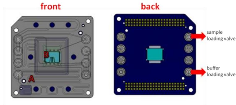
**FIGURE 1 DEPARRAY CHIP (A300K).** FRONTAL VIEW: MICROFLUIDIC SYSTEM (A) WHERE THE SYSTEM IS ABLE TO LOAD THE SAMPLE THROUGH THE PRESSURE CONTROLLED IN THE VALVES AND TO CARRY THE RECOVERIES IN VOLUMES CHOSEN BY THE OPERATOR; THE ACTIVE AREA OF THE CHIP (B) WHERE SAMPLES ANALYSIS TAKES PLACE. BACK VIEW, CONTROL VALVES, ONE FOR THE LOADING THE SAMPLE AND ONE FOR THE BUFFER LOADING.
