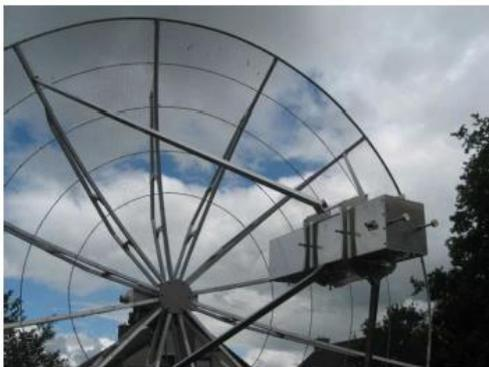
**Figure 15. Septum dish feed mounted on a 3m parabolic dish by RF Hamdesign**
