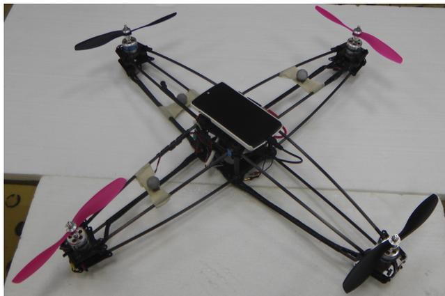
Figure 4.1: The quadrotor prototype
