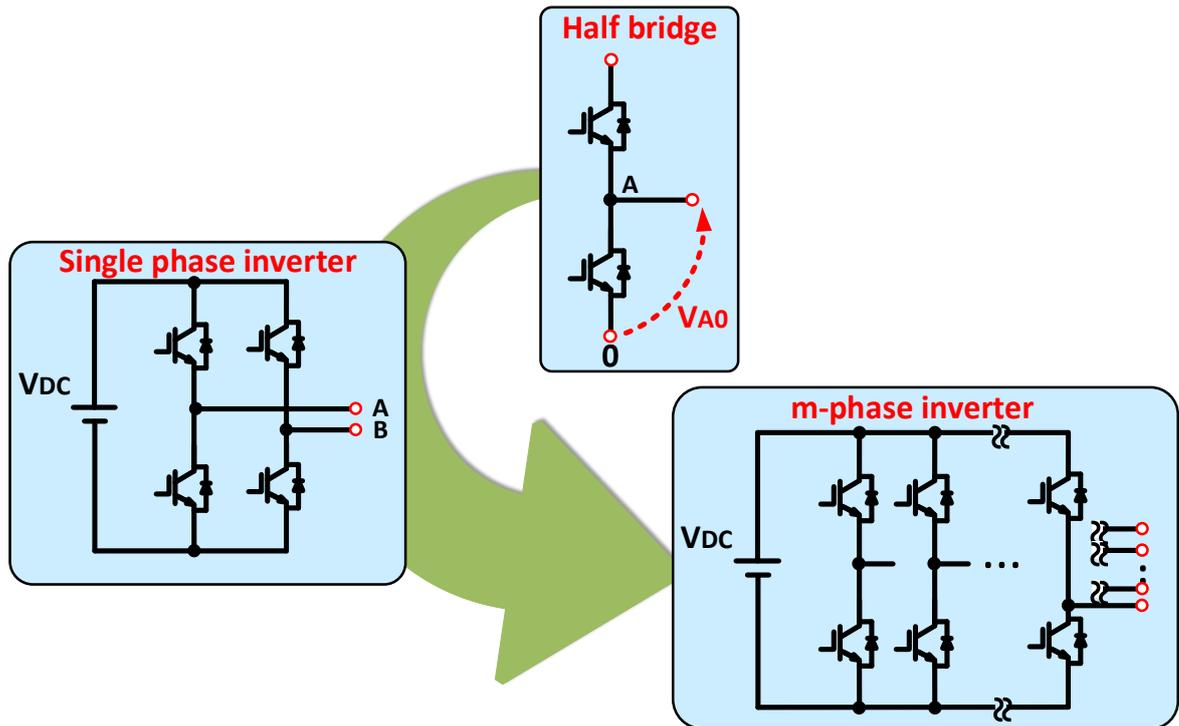
Figure 2.2 – multi phase DC/AC converters based on the half bridge leg.
