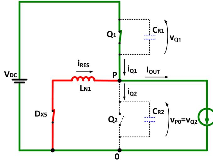
Figure 3.28 - Equivalent circuit of the ZVT2CI converter during time  $[t_5, t_6]$ .
