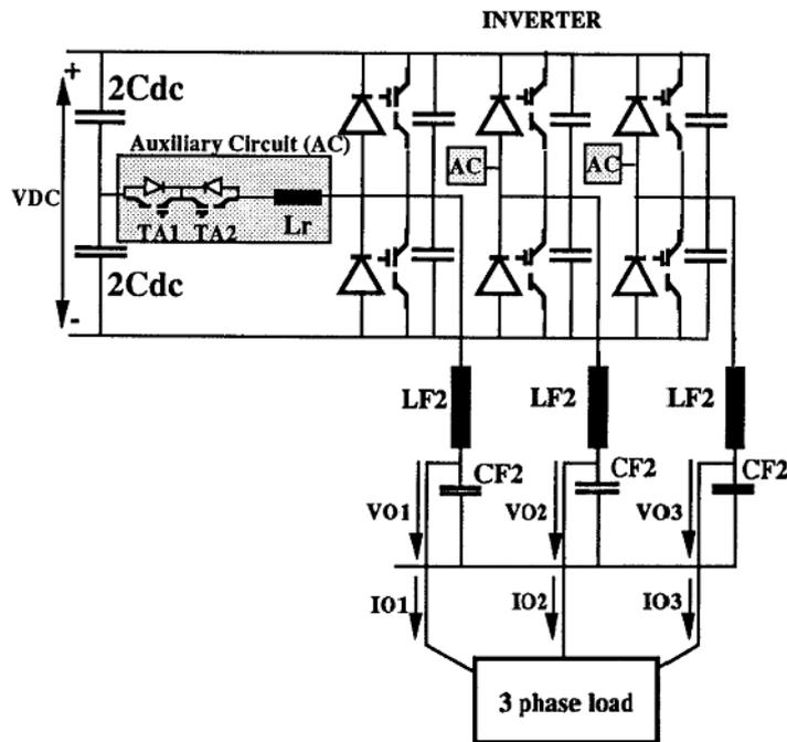
Figure 3.6 - ARCP DC to AC converter.
