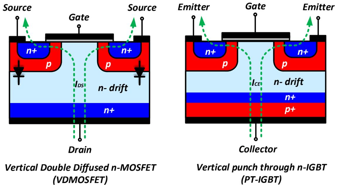
Figure 1.7 – Comparison of the structure of a VDMOSFET and of a PT IGBT.
