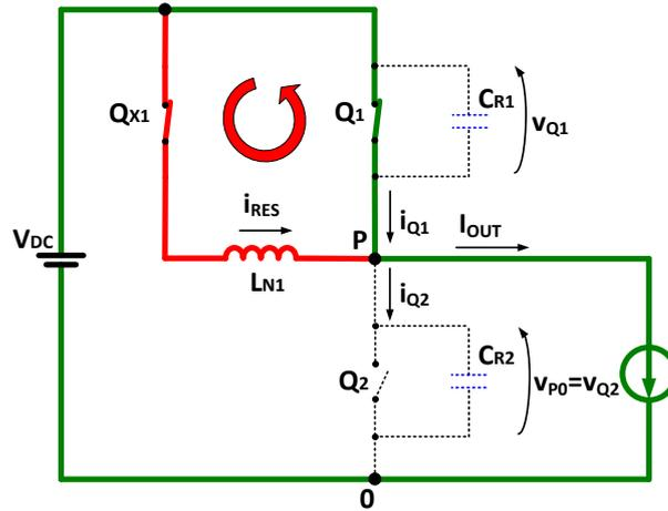
Figure 3.26 - Equivalent circuit of the ZVT2CI converter during time  $[t_4, t_5]$ .
