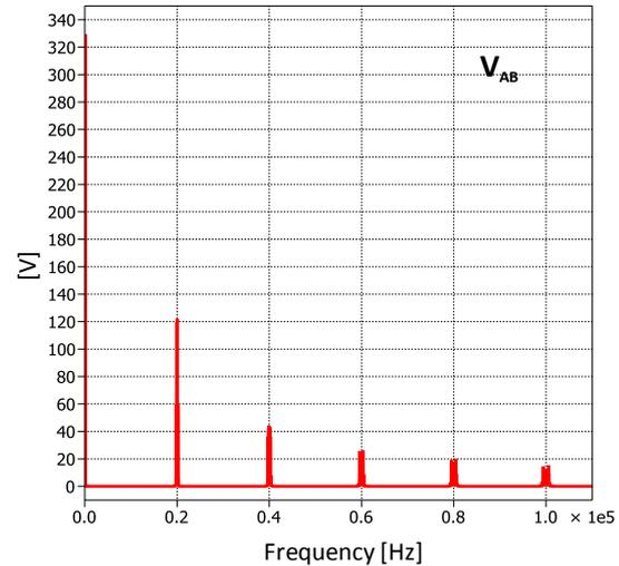
Figure 4.25 - Harmonic content of the output voltage  $V_{AB}$  generated by high side discontinuous modulation.
