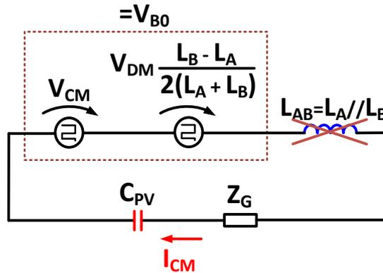
Figure 4.21 – Simplified CM circuit of the full bridge converter controlled by means of hybrid modulation. The total common mode voltage is equal to  $V_{B0}$ .
