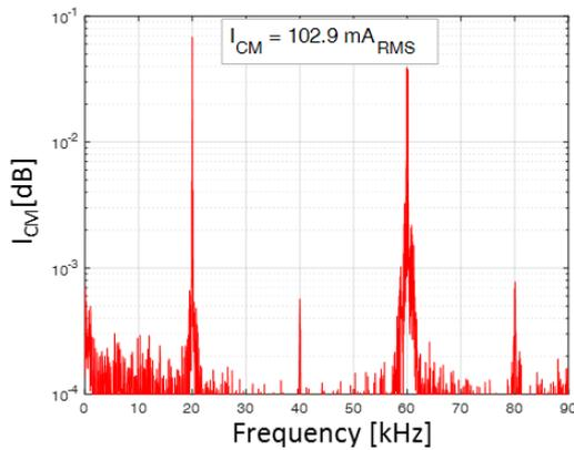
c) Harmonic content of the leakage current
