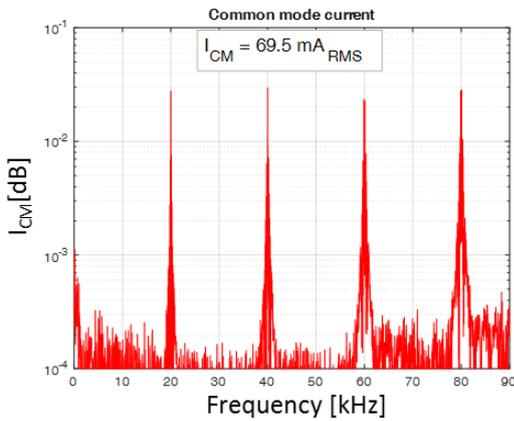
c) Harmonic content of the leakage current
