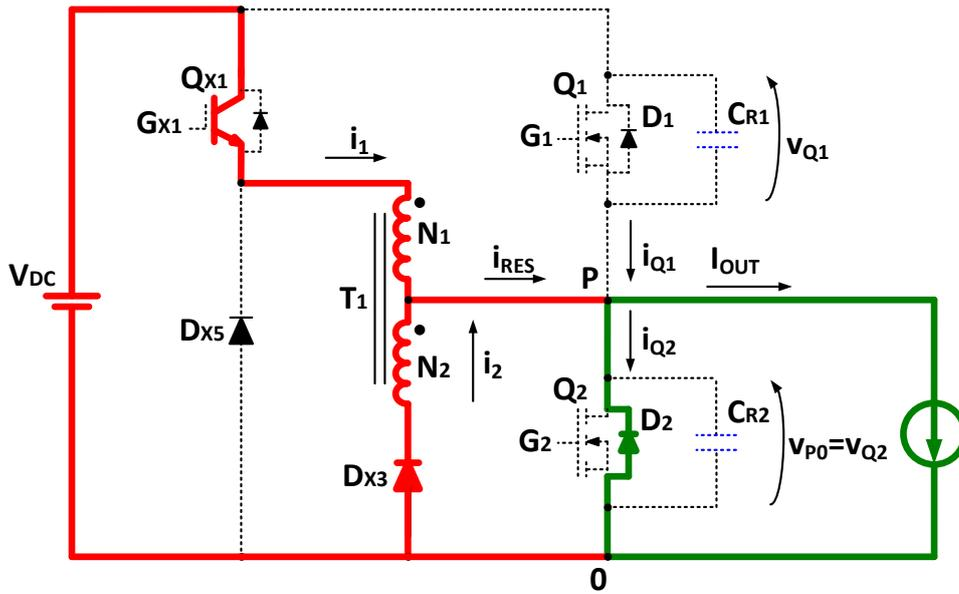
Figure 3.16 - Detail of the ZVT2CI converter during time  $[t_1, t_2]$ .
