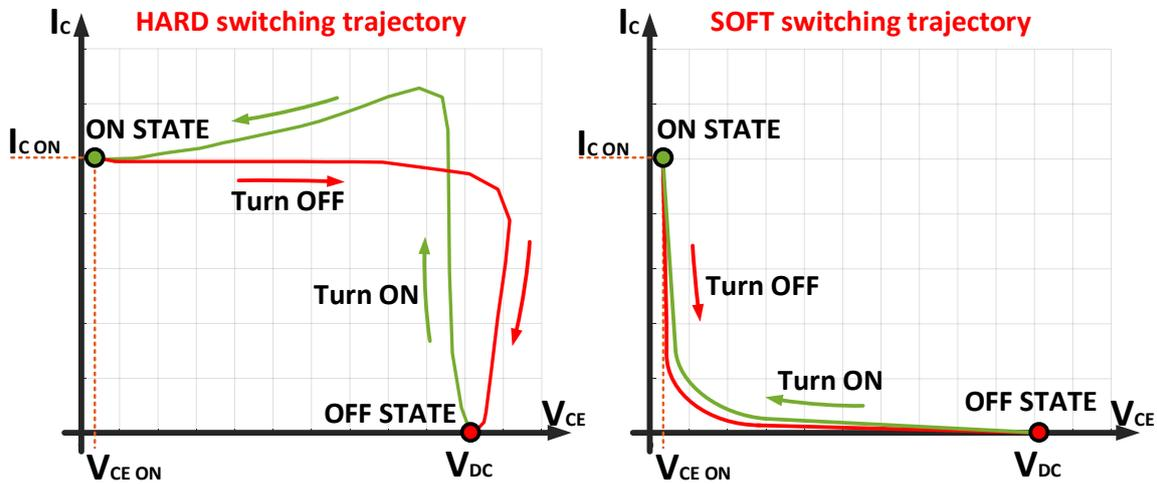
Figure 2.6 – Comparison of hard and soft switching trajectories.
