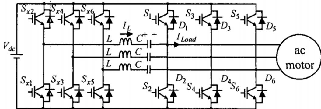
Figure 3.7 – Schematic of a three phase ZCT.
