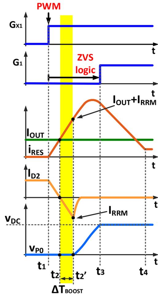
Figure 3.35 - Resonant transition of the converter if real diodes are considered.
