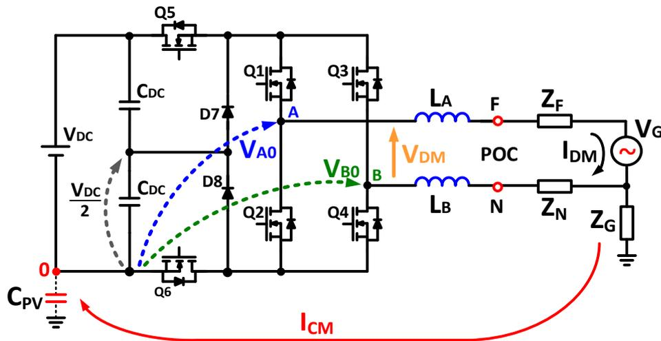
Figure 4.26 - Grid connected H6 converter.
