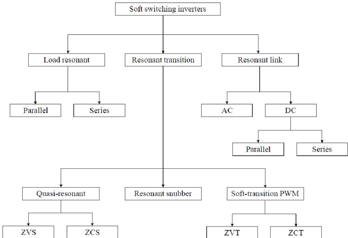
Figure 3.2 – Classification of soft switching DC/AC converters
