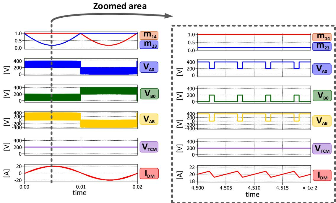
Figure 4.27 - Simulation results of H6 converter.
