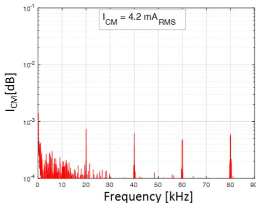
c) Harmonic content of the leakage current
