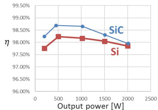
b) Efficiency comparison of SiC and Si prototypes.
