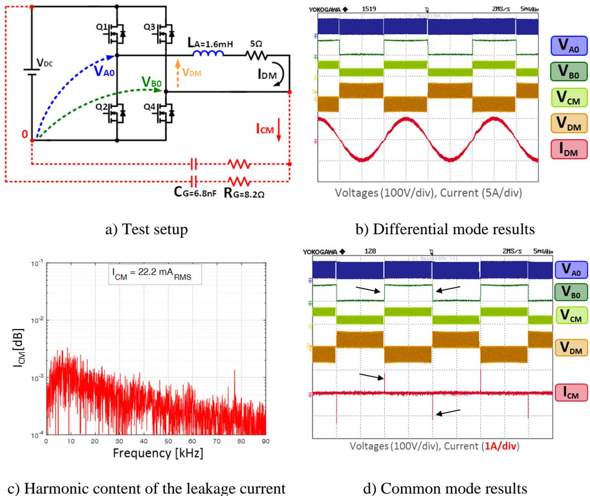
Figure 4.38 - Experimental results of full bridge converter controlled by means of hybrid modulation.
