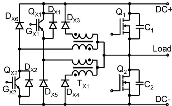
Figure 3.11 - Schematic of a ZVT2CI inverter leg.
