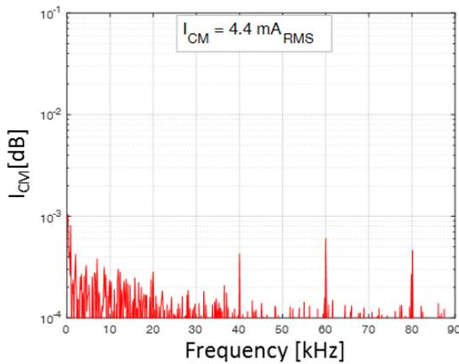
c) Harmonic content of the leakage current
