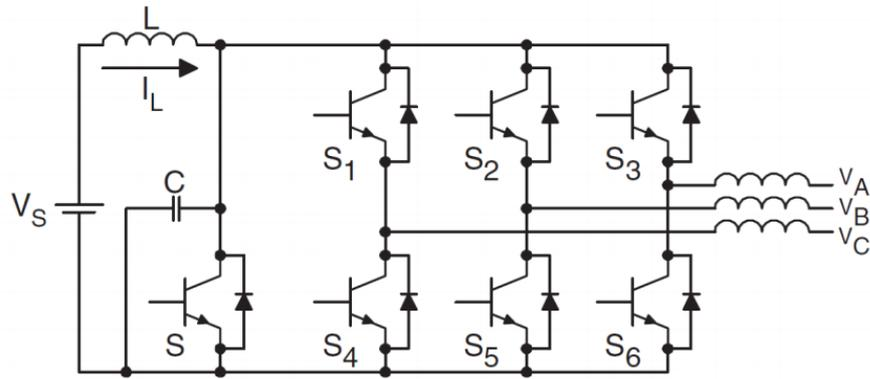
Figure 3.3 - Resonant DC-Link Inverter.
