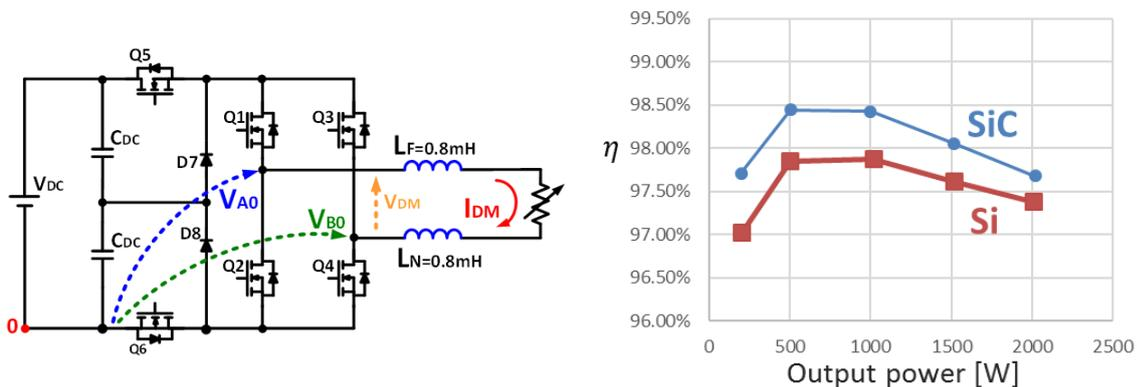
a) Test setup.      b) Efficiency comparison of SiC and Si prototypes.
