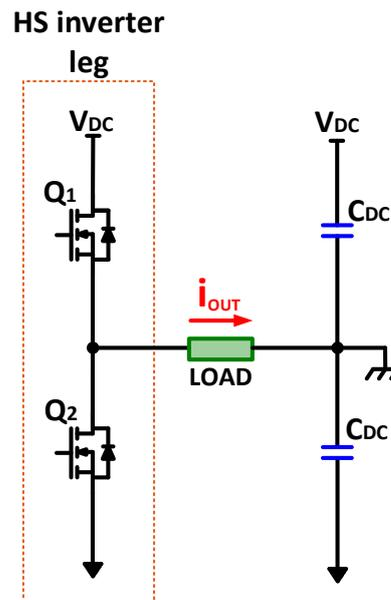
Figure 3.52 - Schematic of a leg of the hard-switching inverter.
