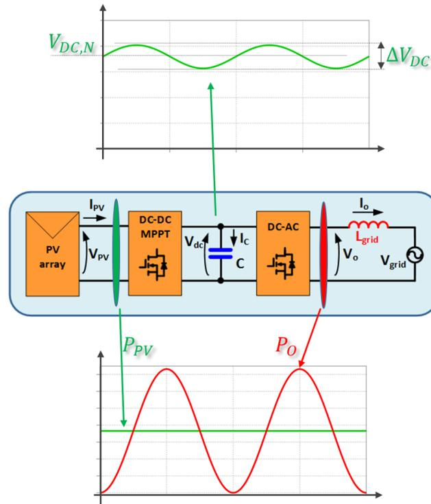
Figure 4.33 – Power balance on the DC link capacitor of a single phase PV system.
