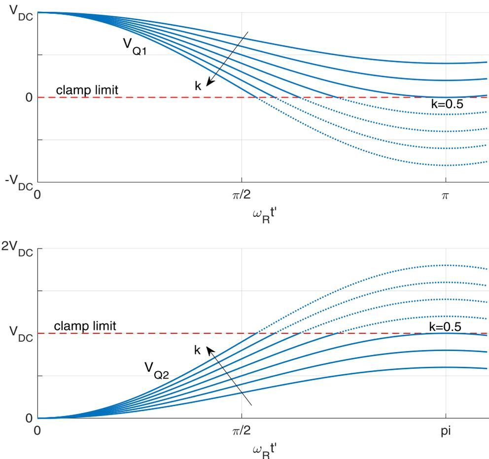
Figure 3.21 – Resonant transition of voltages  $V_{Q1}$  and  $V_{Q2}$  during time  $[t_2, t_3]$ .
