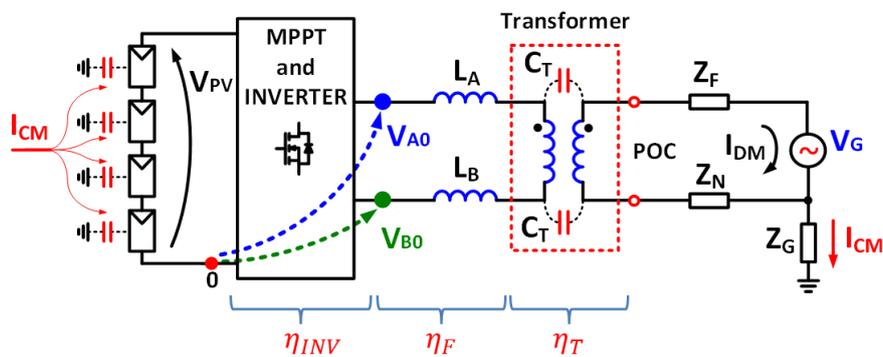
Figure 4.4 – Single phase PV system with isolation transformer.
