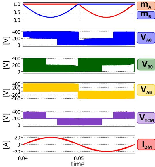
Figure 4.24 - Simulation results of H5 converter controlled by means of high side discontinuous modulation.
