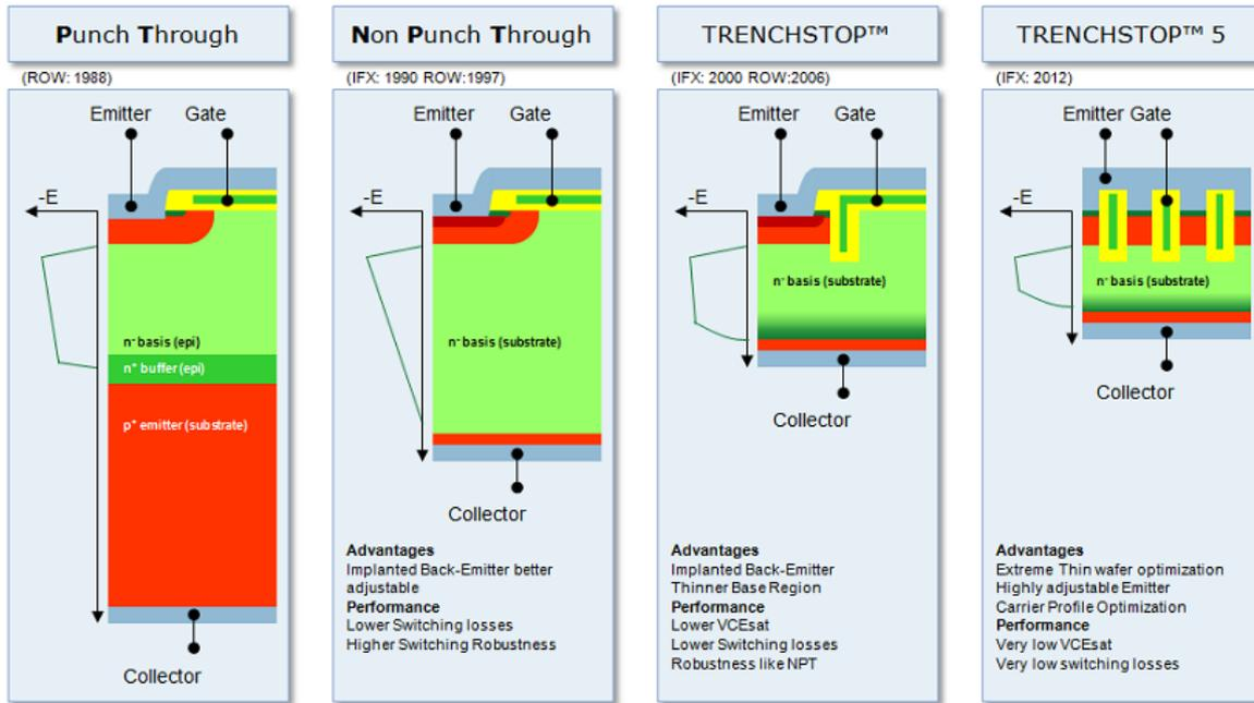
Figure 1.8 - Evolution of Infineon IGBTs, from Punch Trough to TRENCHSTOP™ 5 technology
