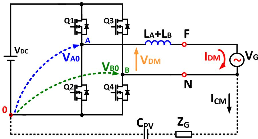
Figure 4.19 - Grid connected full bridge converter controlled by means of hybrid modulation.
