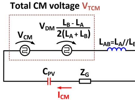
Figure 4.9 - Simplified model of the PV system showing the total common mode voltage  $V_{TCM}$ .
