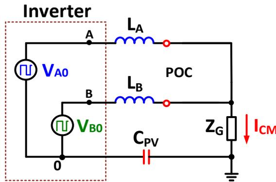
Figure 4.8 - High frequency model of the PV system
