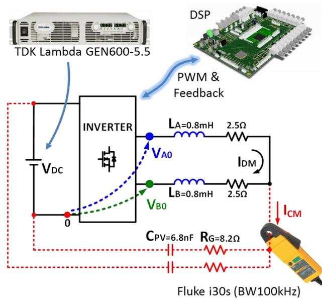
Figure 4.34 – Experimental test setup.
