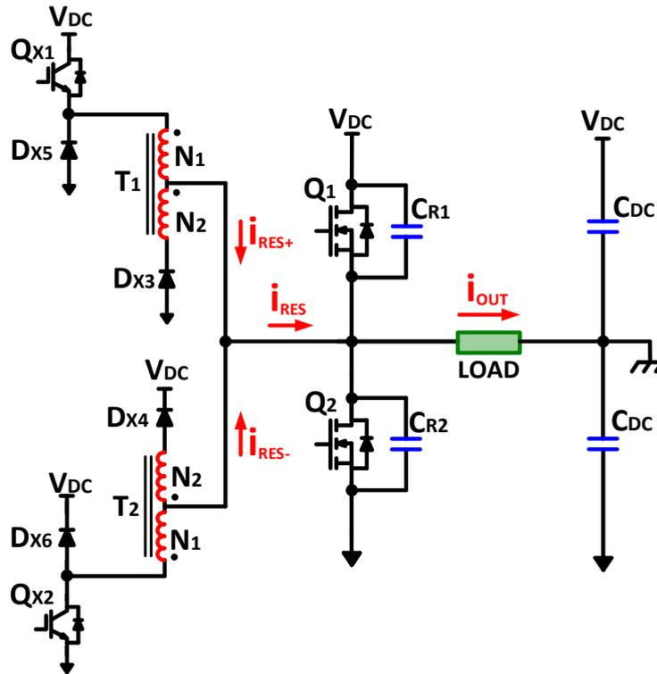
Figure 3.46 - Schematic of a leg of the ZVT2CI inverter.
