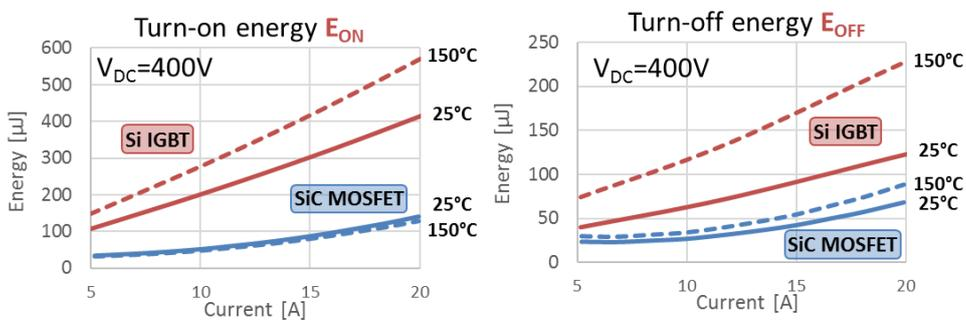
Figure 3.54 – Switching energies of the Si IGBT and SiC MOSFET selected.
