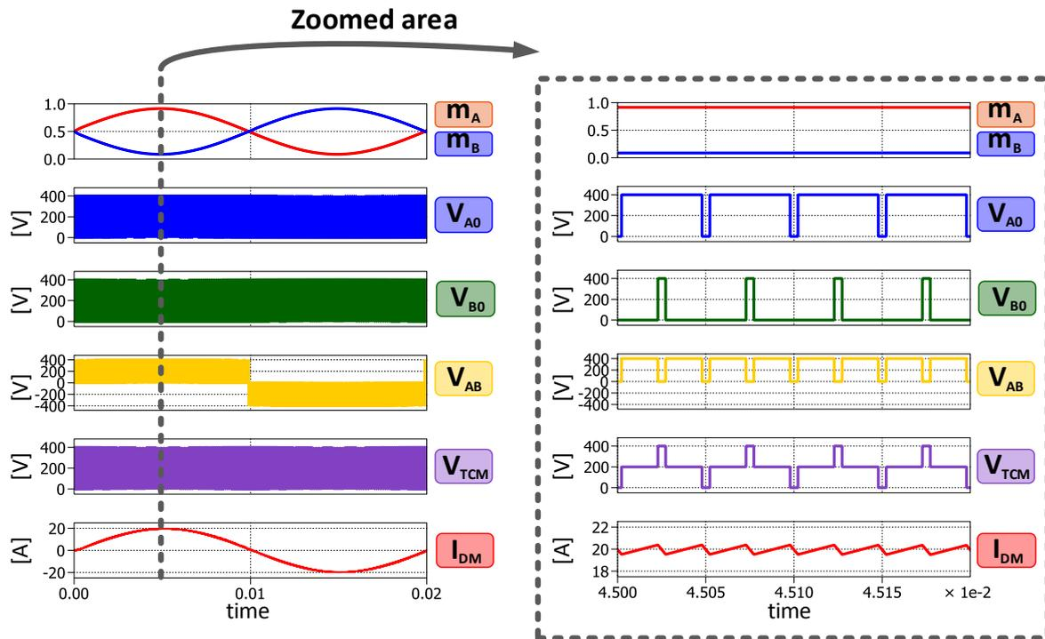
Figure 4.15 - Simulation results of full bridge converter controlled by means of unipolar modulation.
