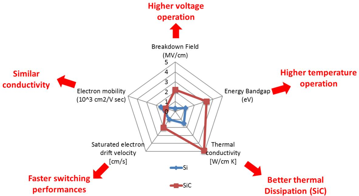
Figure 1.9 - Material properties of silicon and silicon carbide.
