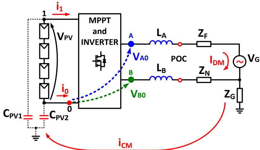
Figure 4.6 – Transformerless PV system schematic showing the leakage loop.
