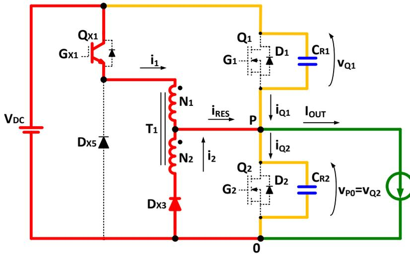
Figure 3.18 - Detail of the ZVT2CI converter during time  $[t_2, t_3]$ .
