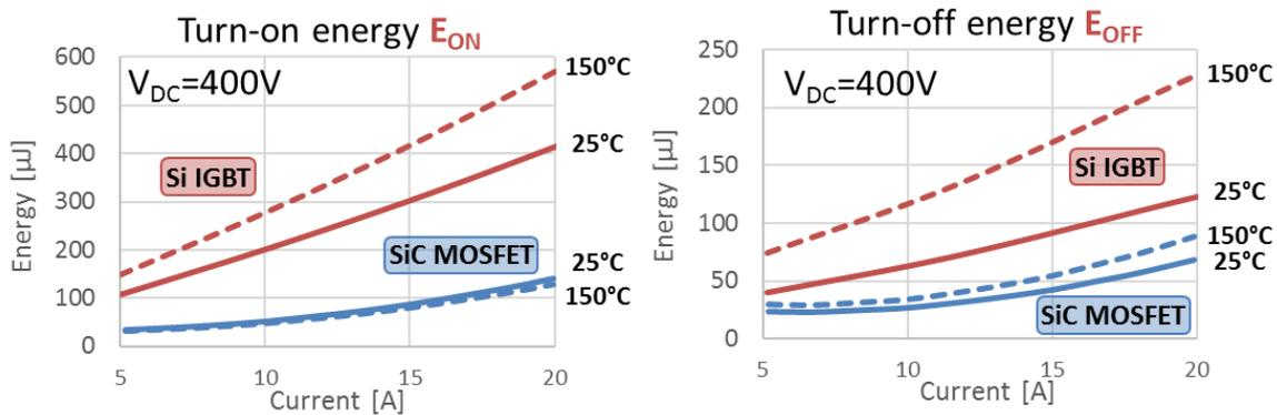
Figure 4.44 – Switching energies of the Si IGBT and SiC MOSFET selected.
