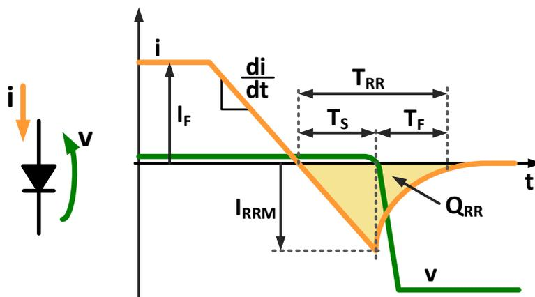
Figure 3.33 - Reverse recovery waveforms and definitions.
