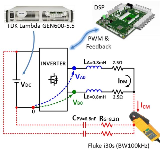
Figure 4.34 – Experimental test setup.
