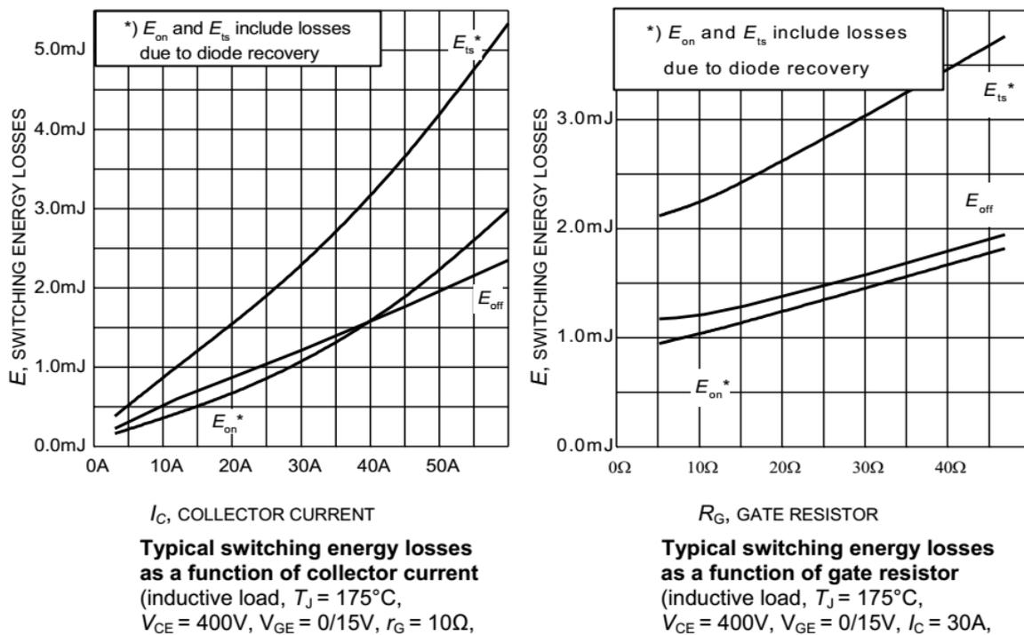
Figure 2.4 – Switching energies of the IGBT Infineon IKW30N60T as function of collector current (left figure) and of gate resistance (right figure)
