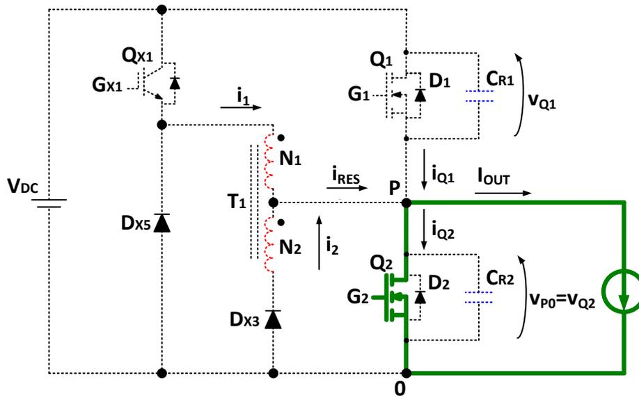
Figure 3.32 - Detail of the ZVT2CI converter during time  $[t_8, t_9]$ .
