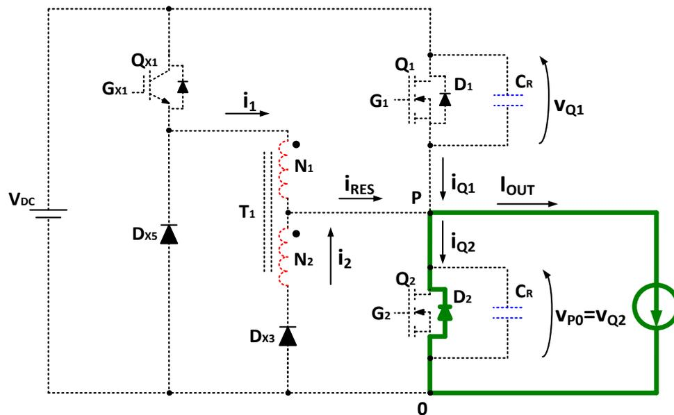
Figure 3.15 –Detail of the ZVT2CI converter during time  $[t_0, t_1]$ .
