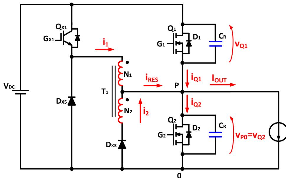
Figure 3.13 - Schematic of the ZVT2CI converter, considering only the main bridge and the positive current auxiliary pole.
