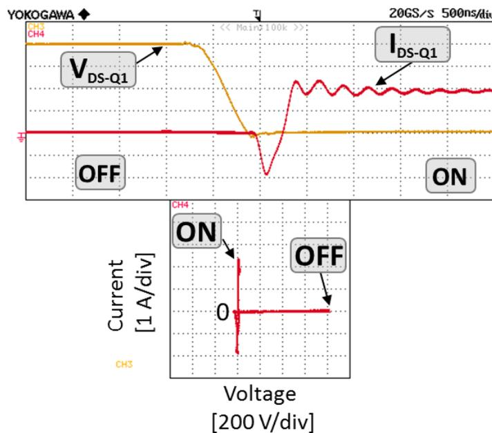
Figure 3.49 - Detail of the zero-voltage turn-on of switch  $Q_1$  and switching trajectory.
