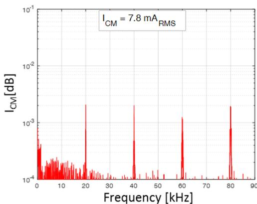
c) Harmonic content of the leakage current
