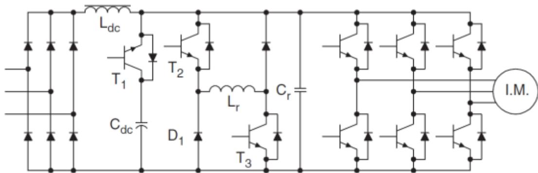
Figure 3.5 - Resonant Inverter with Minimum Voltage Stress.
