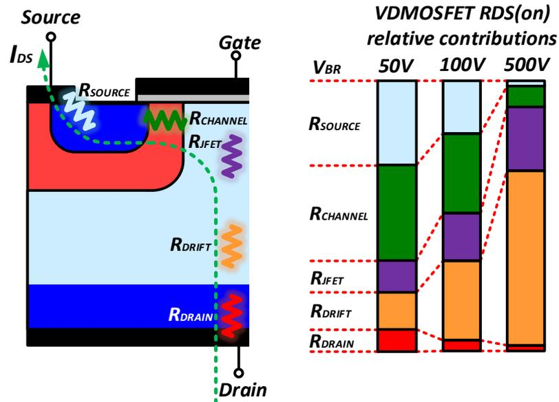
Figure 1.4 - Contribution to the on state resistance of a VDMOSFET as function of the blocking voltage
