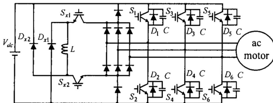
Figure 3.9 - Schematic of a three phase ZVTSI.
