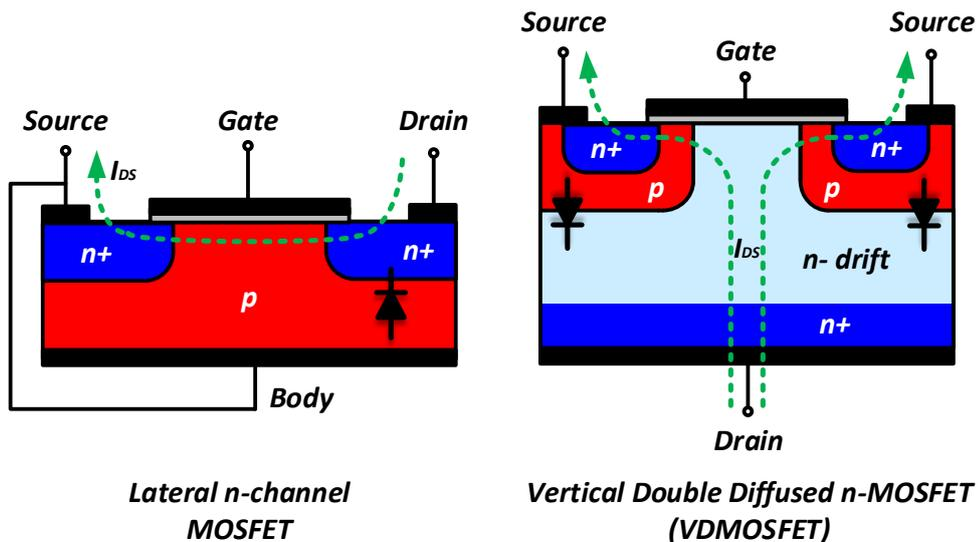
Figure 1.3 – Lateral and vertical MOSFET structures.
