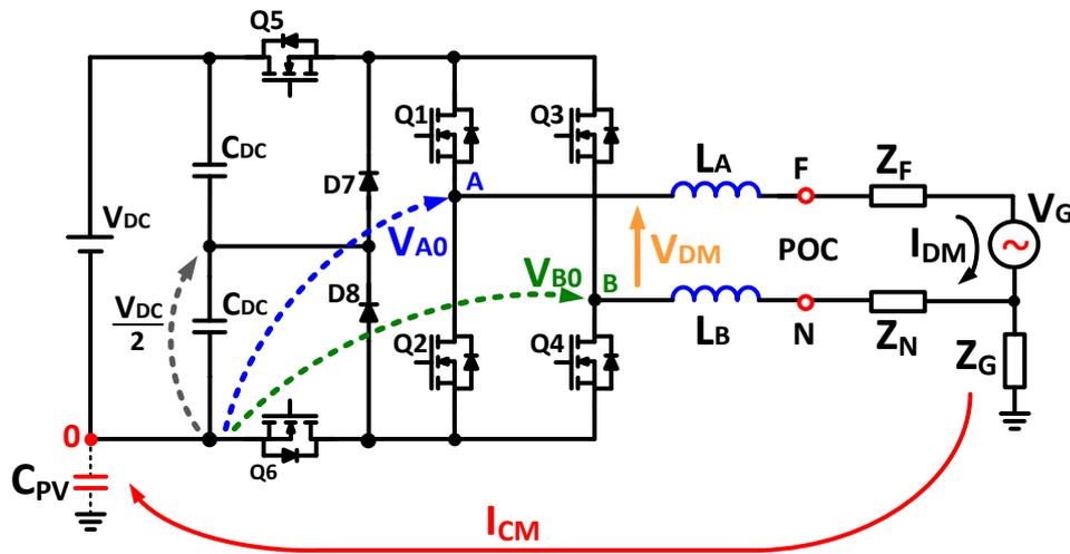
Figure 4.26 - Grid connected H6 converter.
