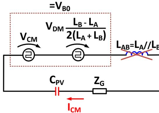
Figure 4.21 – Simplified CM circuit of the full bridge converter controlle by means of hybrid modulation. The total common mode voltage is equal to  $V_{B0}$ .
