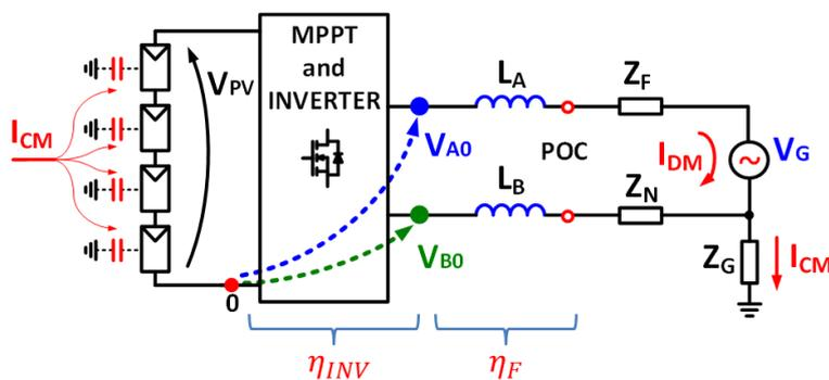
Figure 4.5 - Single phase transformerless PV system.
