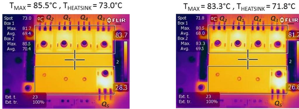
c) IR picture of the Si prototype at output power of 2000 W.      d) IR picture of the SiC prototype at output power of 2000 W.
