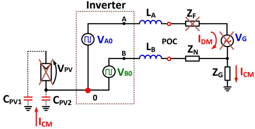
Figure 4.7 – Simplified model of the PV system.
