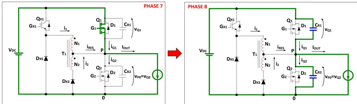
Figure 3.36 – Turn-off of  $Q_1$  considering ideal switches. ZVS is achieved since the load current commutate instantly from the transistor to the capacitor  $C_{R1}$ .
