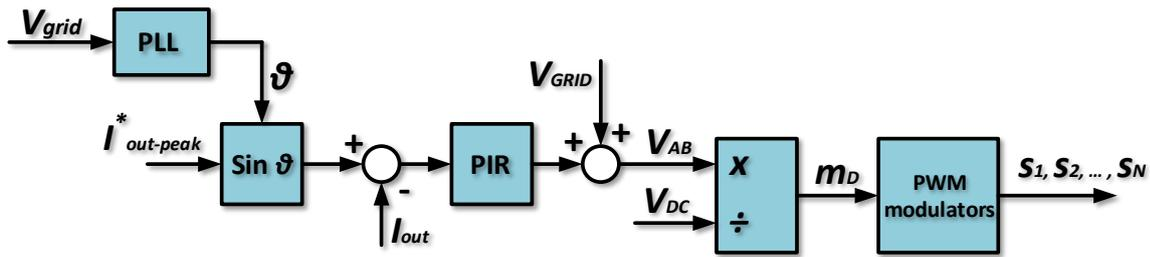
Figure 4.11 - Output current control scheme.
