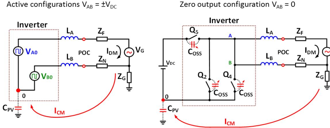
Figure 4.23 – Simplified circuit of the H5 converter during active configurations (left) and zero output configurations (right).
