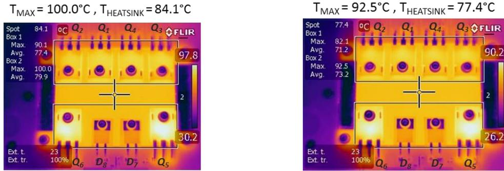
c) IR picture of the Si prototype at output power of 2000 W.      d) IR picture of the SiC prototype at output power of 2000 W.
