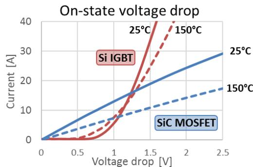
Figure 3.53 – V-I characteristic of the Si IGBT and SiC MOSFET selected.
