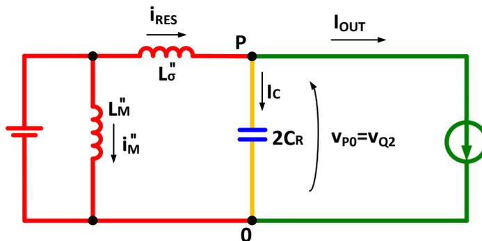
Figure 3.20 - Equivalent circuit of the ZVT2CI converter during time  $[t_2, t_3]$ .
