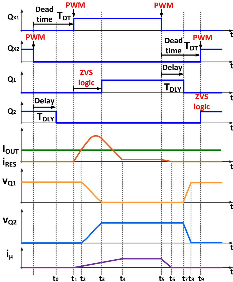
Figure 3.14 - Timing diagram of the ZVT2CI inverter.
