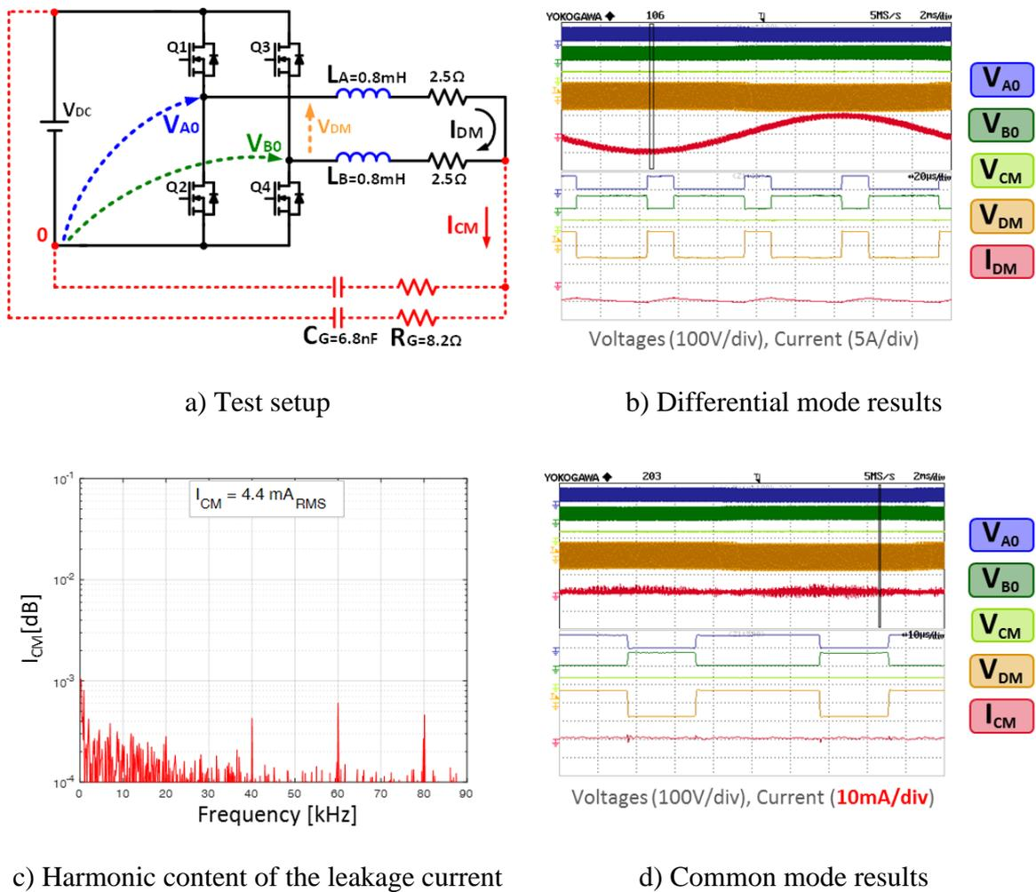
Figure 4.35 – Experimental results of full bridge converter controlled by means of bipolar modulation.
