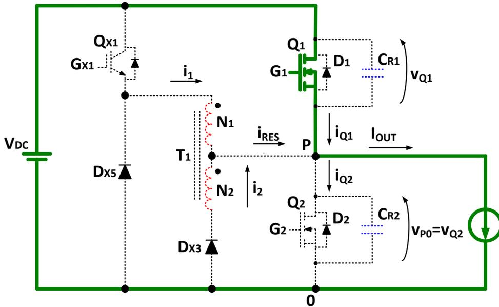
Figure 3.29 - Detail of the ZVT2CI converter during time  $[t_6, t_7]$ .
