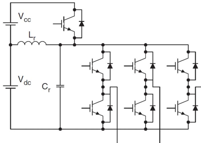
Figure 3.4 - Active-Clamped Resonant DC-Link Inverter.
