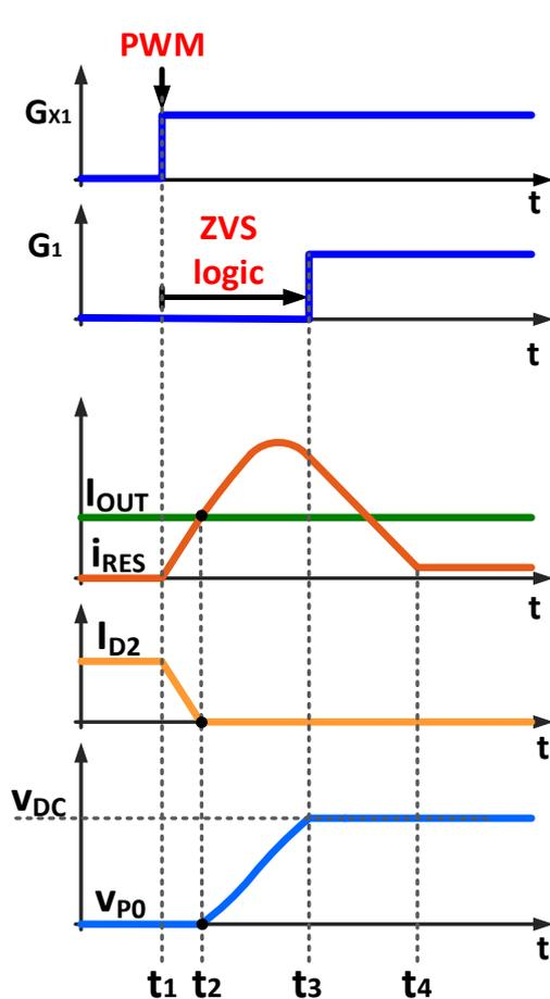
Figure 3.34 - Resonant transition of the converter if ideal diodes are considered.
