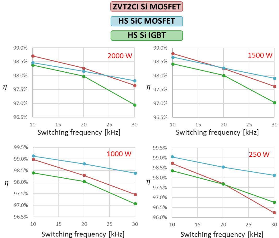
Figure 3.59 - Comparison of the efficiency of prototypes as a function of the switching frequency for different output power.
