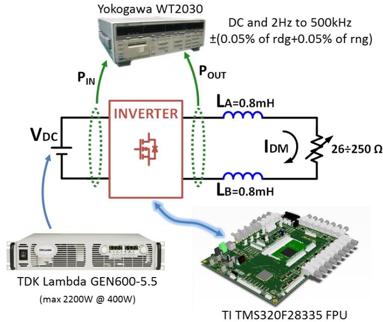
Figure 4.45 – Experimental test setup.
