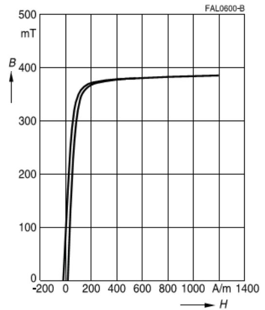
Figure 3.42 – Magnetic hysteresis loop of N87 ferrite.
