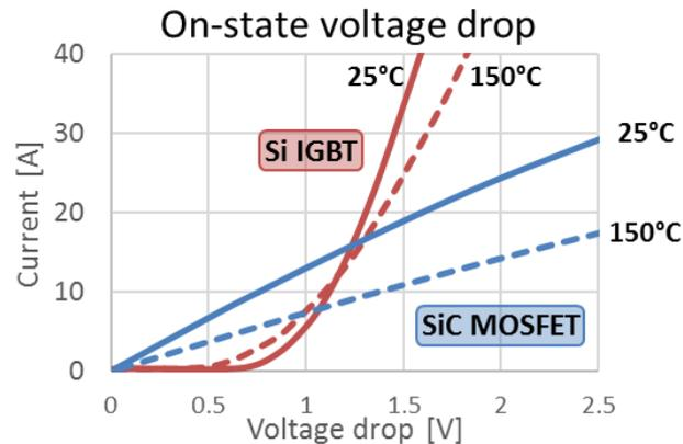
Figure 4.43 - V-I characteristic of the Si IGBT and SiC MOSFET selected.
