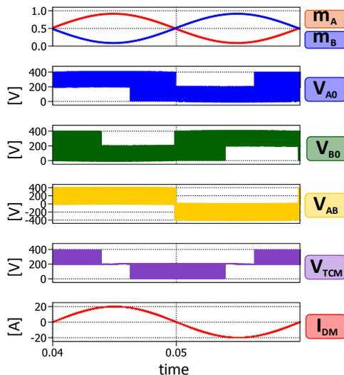
Figure 4.29 - Simulation results H6 converter controlled by means of unipolar modulation.
