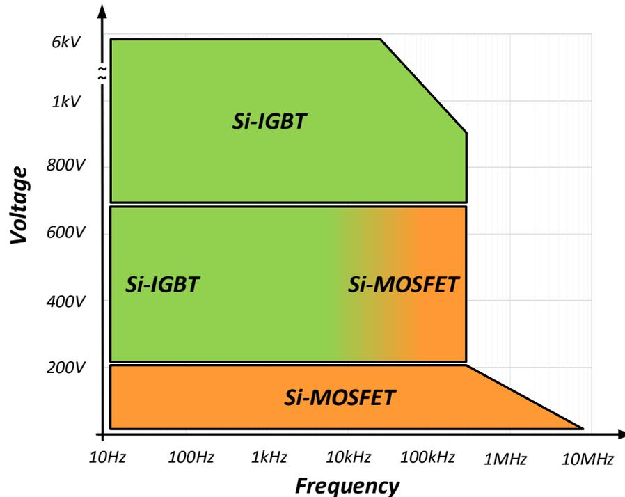
Figure 1.2 - Typical MOSFETs and IGBTs selection as a function of blocking voltage and switching frequency.
