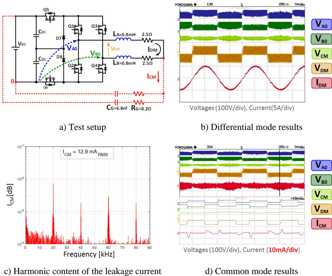
Figure 4.41 - Experimental results of H6 converter controlled by means of unipolar modulation.
