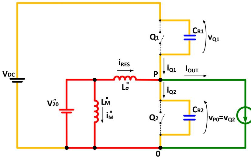
Figure 3.19 - Equivalent circuit of the ZVT2CI converter during time  $[t_2, t_3]$ .
