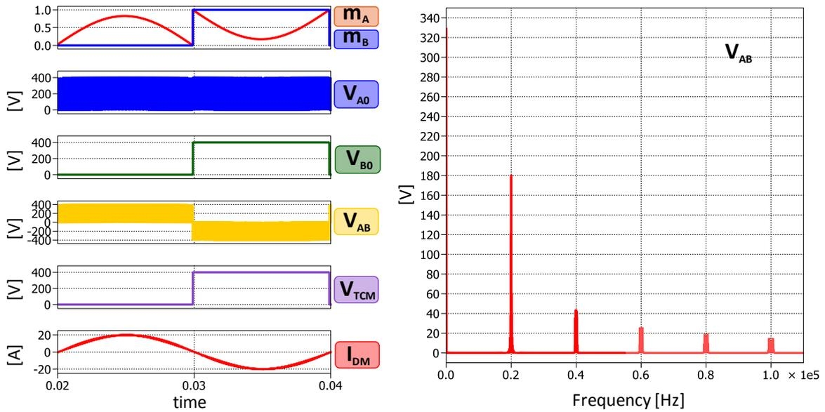
Figure 4.20 - Simulation results and harmonic content of the output voltage  $V_{AB}$  in case of full bridge converter controlled by means of hybrid modulation.
