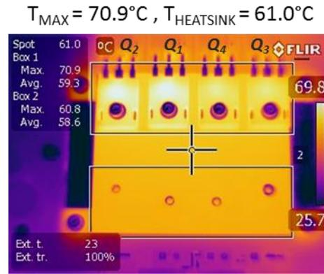
d) IR picture of the SiC prototype at output power of 2000 W.
