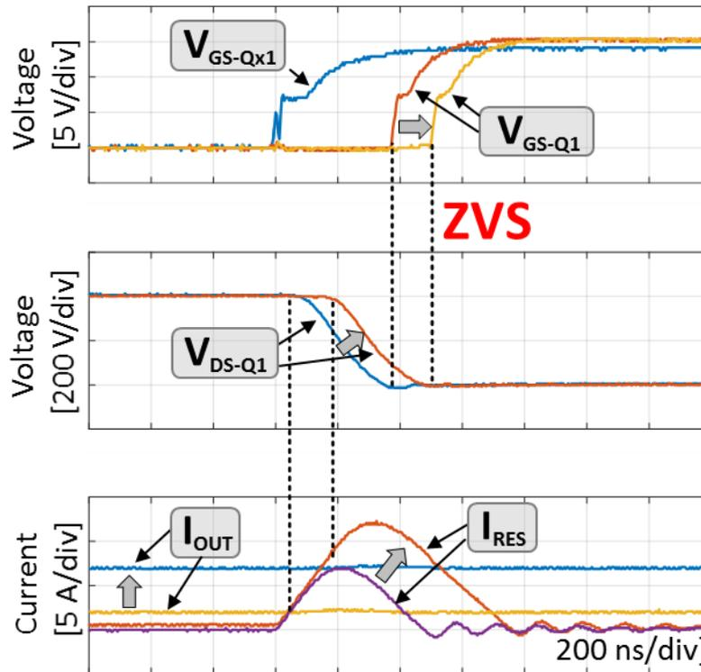
Figure 3.50 - Behavior of the ZVT2CI inverter as the load current increases.
