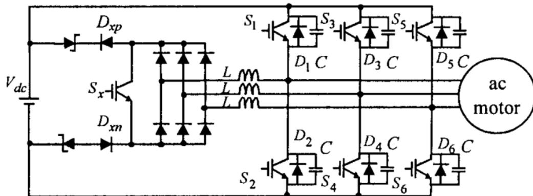
Figure 3.8 - Schematic of a three phase ZVTSS.
