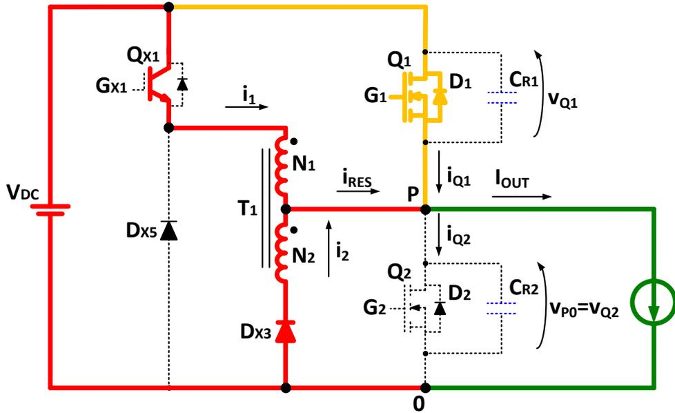
Figure 3.22 – Detail of the ZVT2CI converter during time  $[t_3, t_4]$ .
