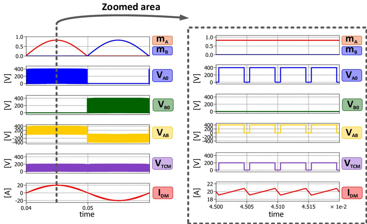
Figure 4.17 - Simulation results of full bridge converter controlled by means of low side discontinuous modulation.
