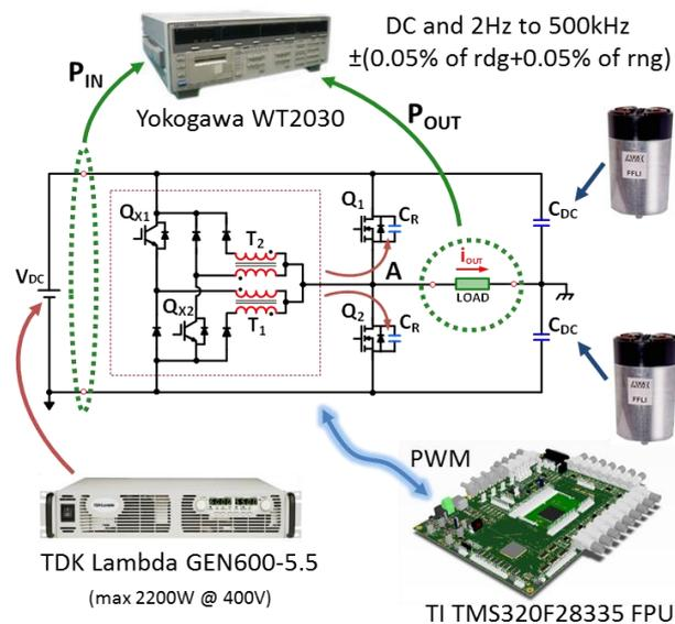
Figure 3.55 – Experimental test setup.
