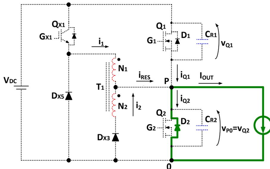
Figure 3.31 - Detail of the ZVT2CI converter during time  $[t_8, t_9]$ .
