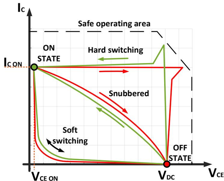
Figure 3.1 – Comparison of typical hard, snubbed and soft switching trajectories of an IGBT or BJT.
