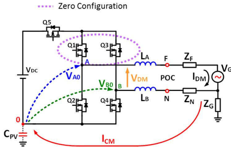
Figure 4.22 - Grid connected H5 converter.
