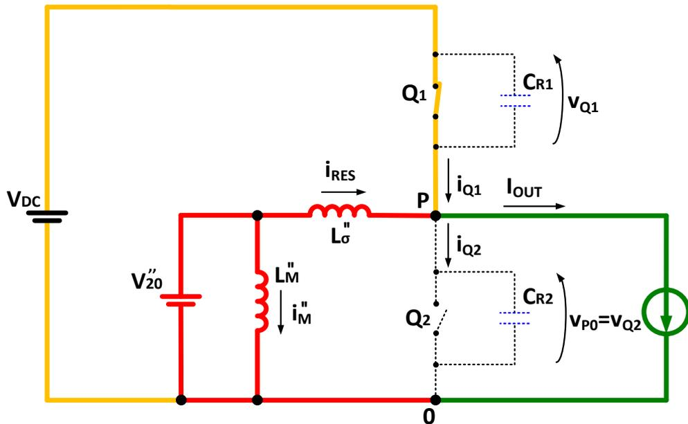
Figure 3.23 - Equivalent circuit of the ZVT2CI converter during time  $[t_3, t_4]$ .
