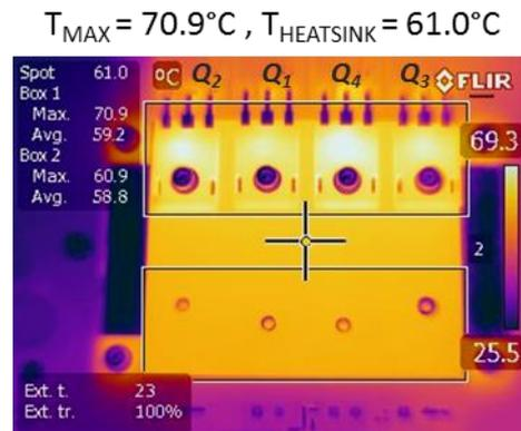
d) IR picture of the SiC prototype at output power of 2000 W.
