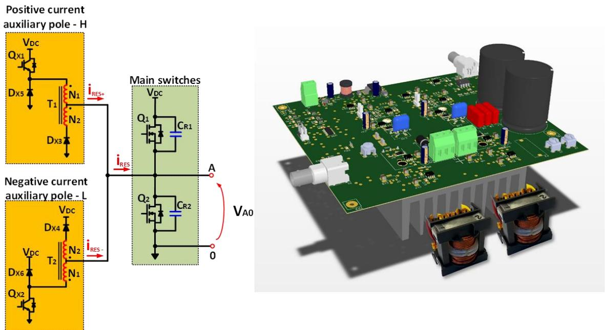
Figure 3.45 – Schematic and 3D rendering of the prototype of ZVT2CI converter.
