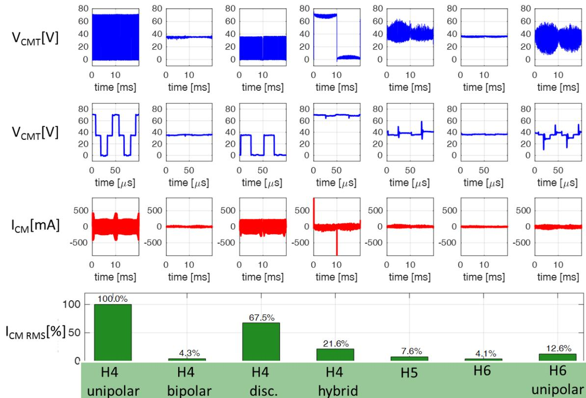
Figure 4.42 – Comparison of the total common mode voltage and leakage current generated by the tested modulation strategies.
