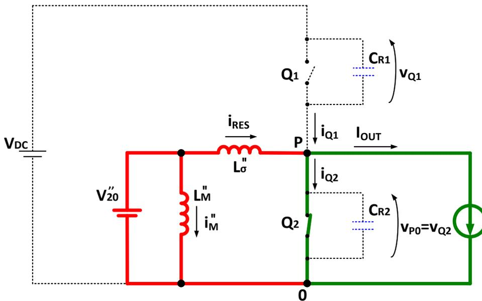
Figure 3.17 – Equivalent circuit of the ZVT2CI converter during time  $[t_1, t_2]$ .
