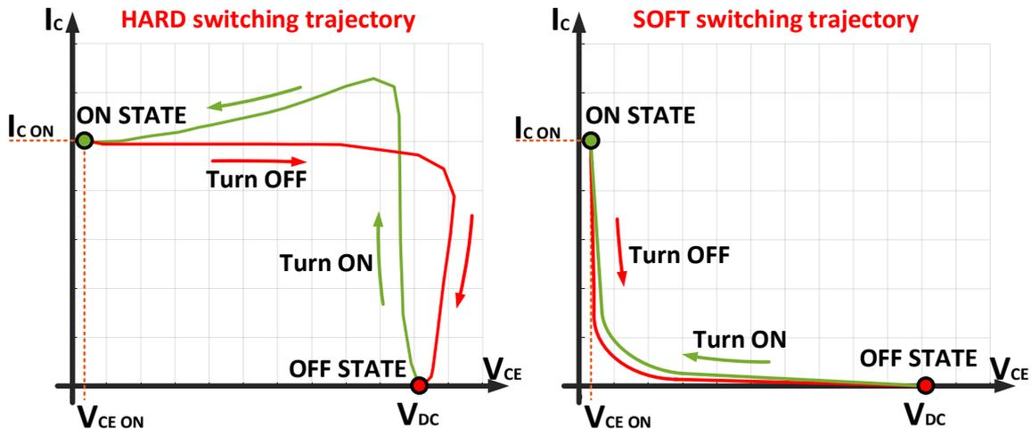
Figure 2.6 – Comparison of hard and soft switching trajectories.
