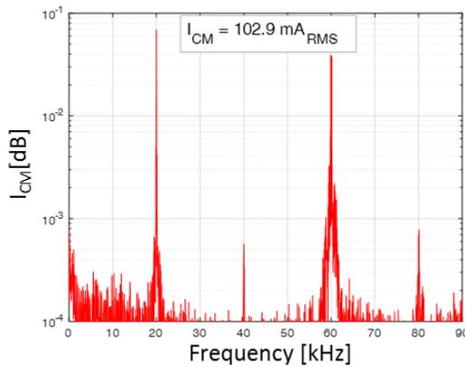
c) Harmonic content of the leakage current
