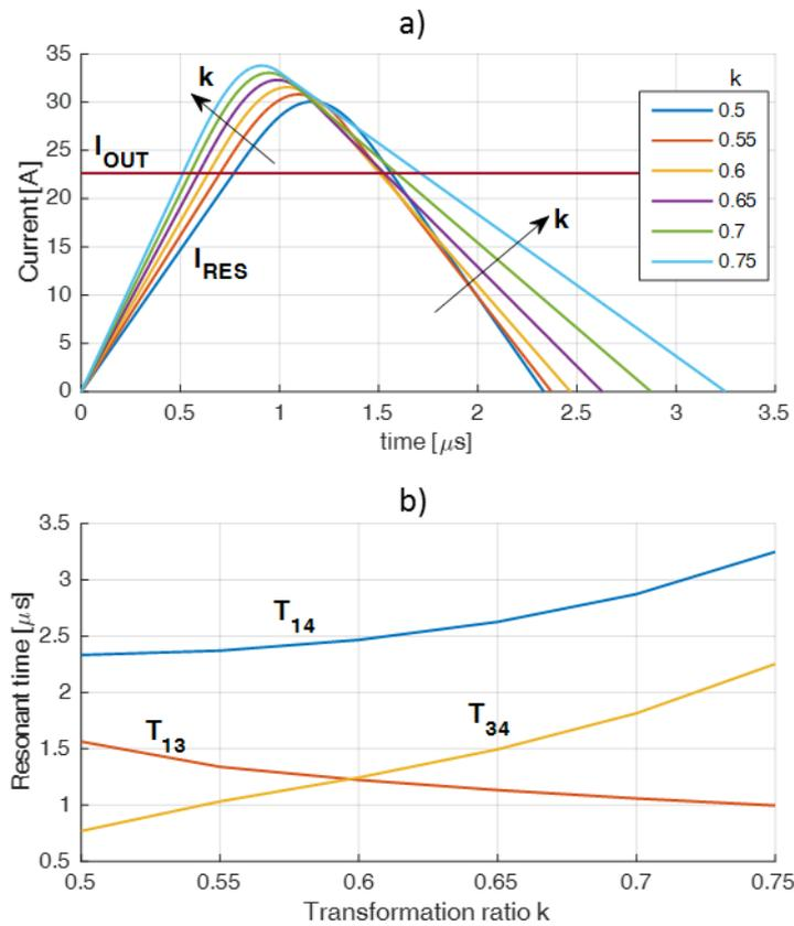
Figure 3.40 - a) Auxiliary current as a function of the transformation ratio of the autotransformer. b) Duration of phases 1, 2, and 3 as a function of the transformation ratio of the autotransformer.
