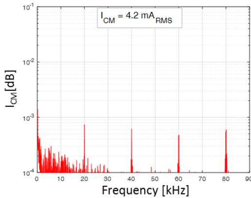
c) Harmonic content of the leakage current
