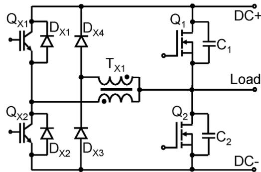
Figure 3.10 - Schematic of a ZVTCI inverter leg.
