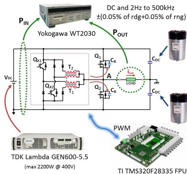
Figure 3.55 – Experimental test setup.
