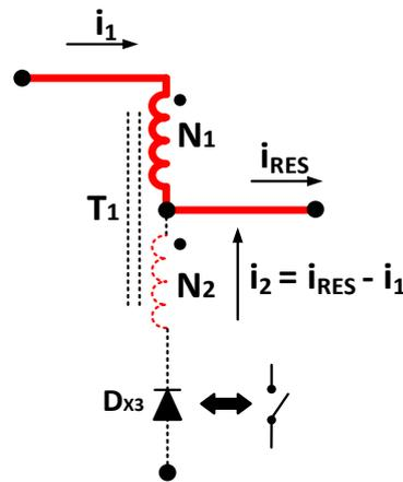
Figure 3.24 – Relation between the resonant current and the currents in the windings of the autotransformer.
