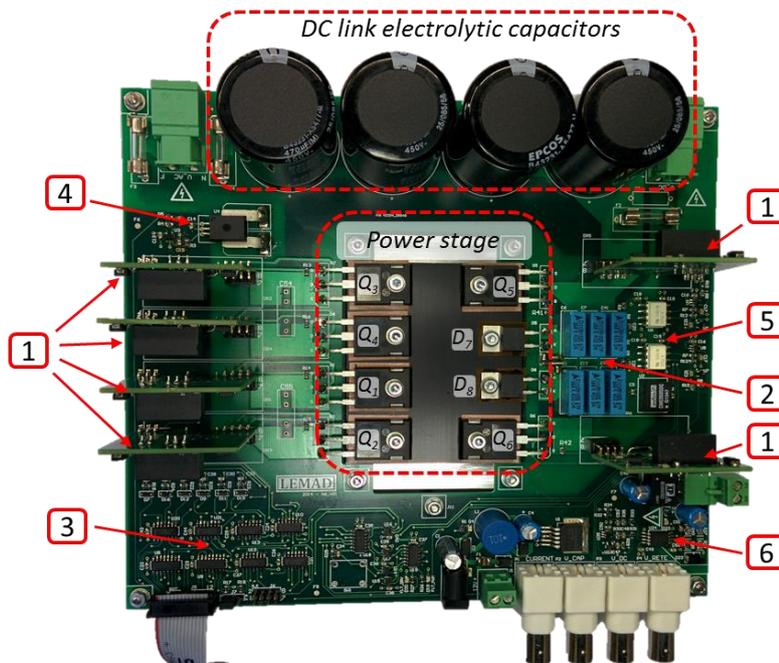
Figure 4.31 – Picture of the H6 converter prototype.
