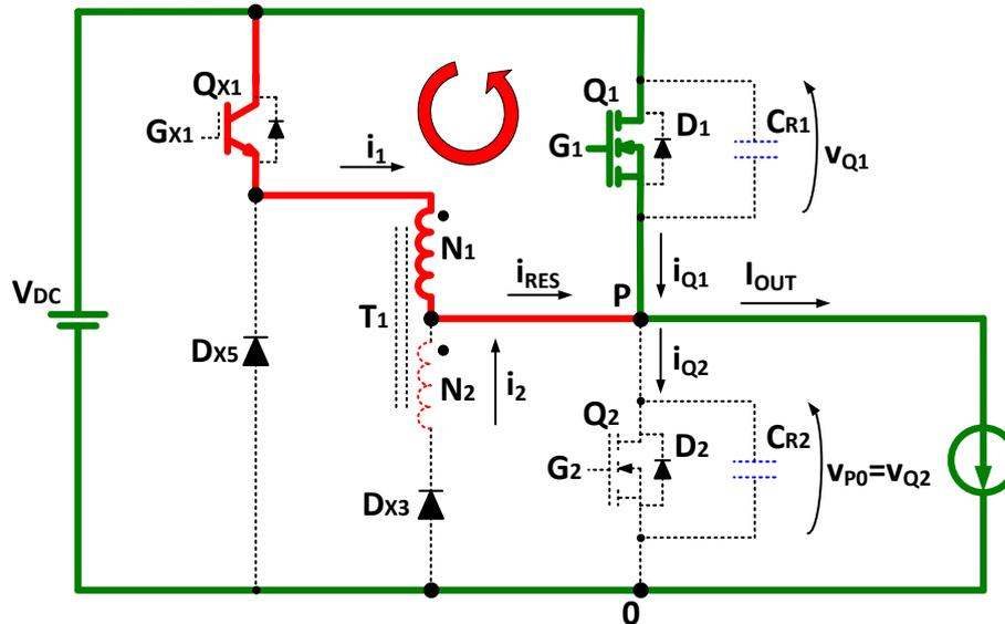
Figure 3.25 - Detail of the ZVT2CI converter during time  $[t_4, t_5]$ .
