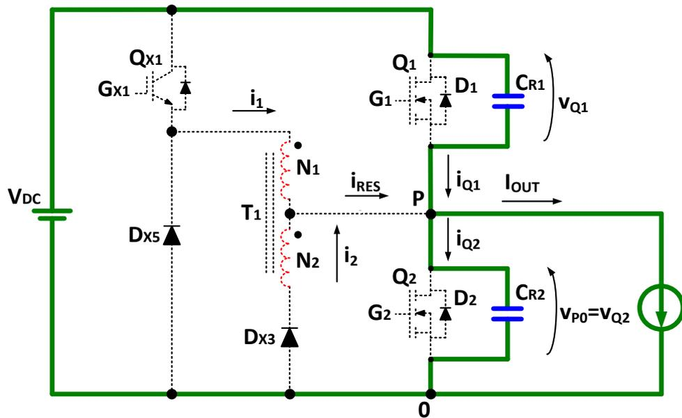
Figure 3.30 - Detail of the ZVT2CI converter during time  $[t_7, t_8]$ .
