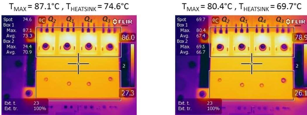
c) IR picture of the Si prototype at output power of 2000 W.
