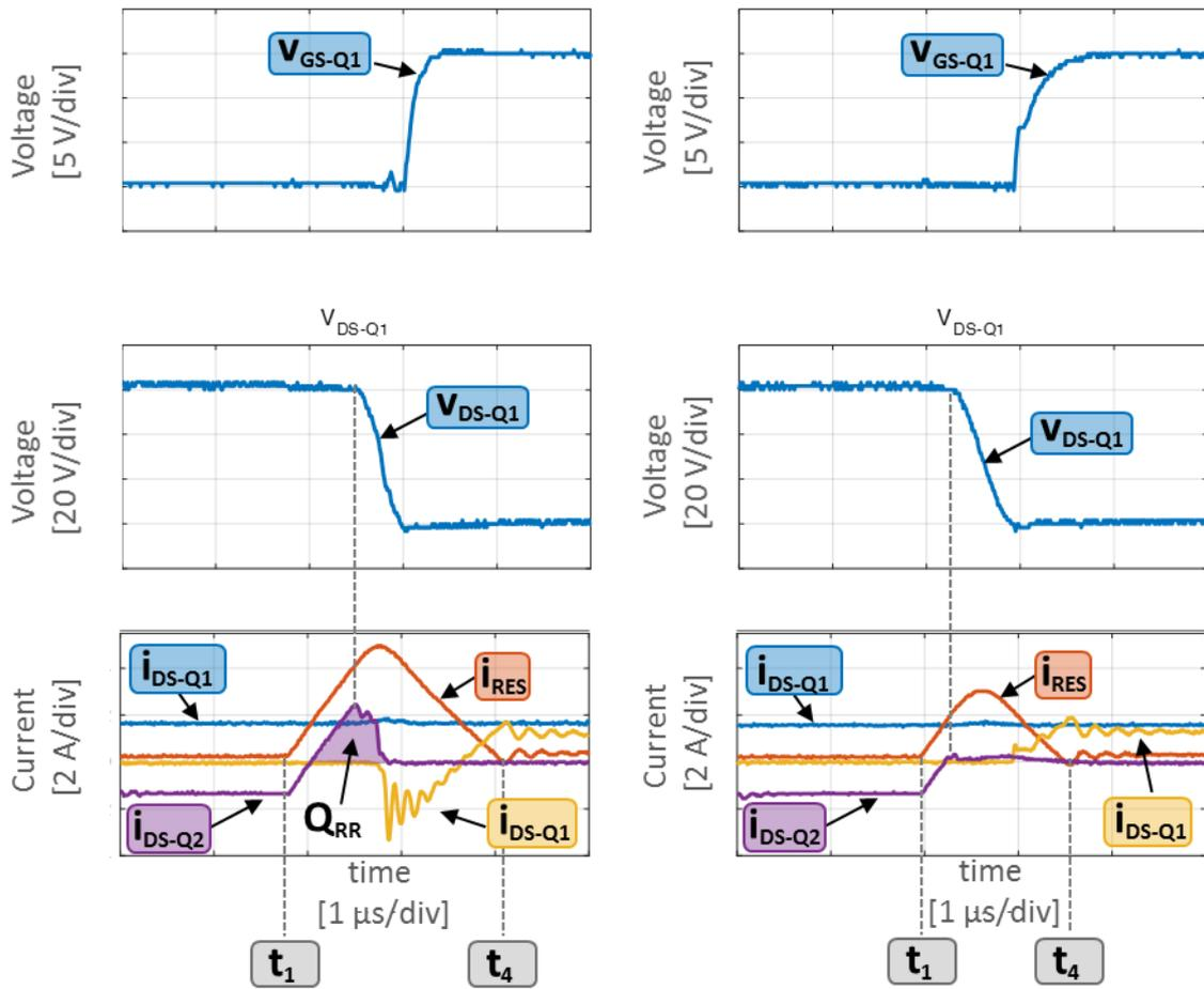
Figure 3.51 – Effect of the reverse recovery of diodes on the behaviour of the converter.
