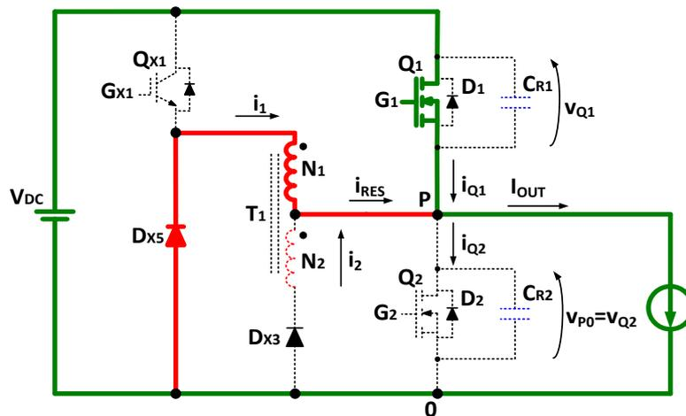
Figure 3.27 - Detail of the ZVT2CI converter during time  $[t_5, t_6]$ .
