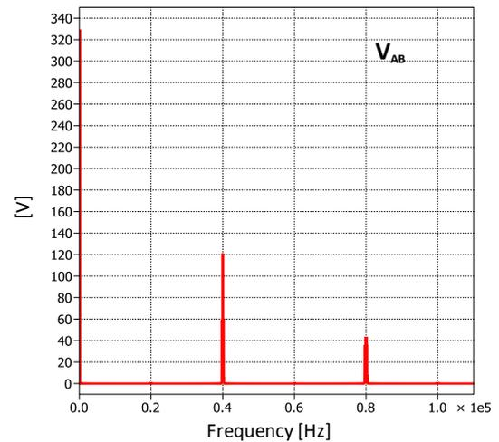
Figure 4.30 - Harmonic content of the output voltage  $V_{AB}$  generated by unipolar modulation.
