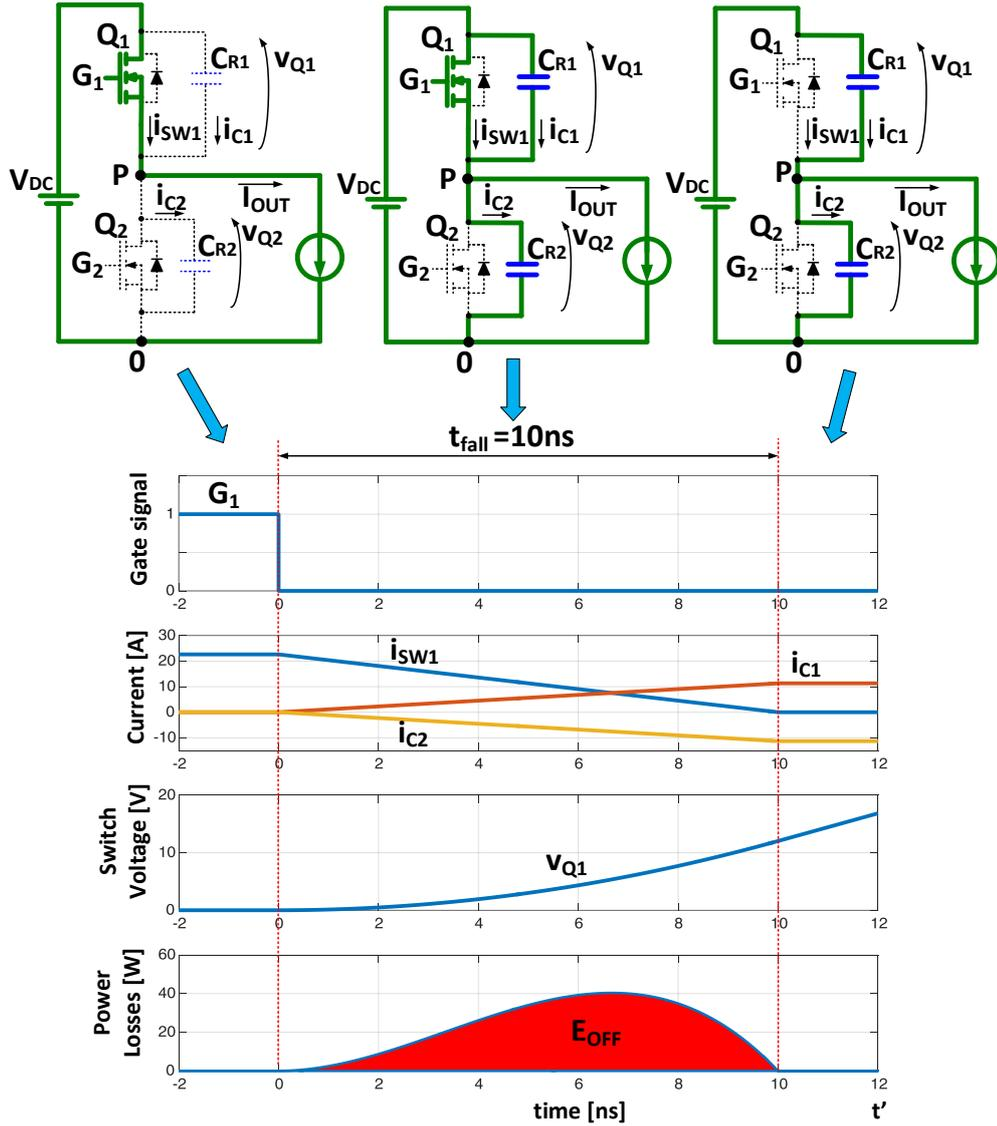
Figure 3.37 - Turn-off loss generation of  $Q_1$  considering a real power transistor.
