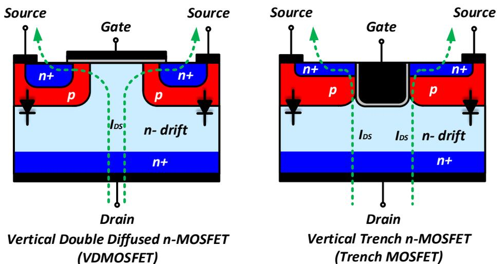
Figure 1.5 – VDMOSFET and trench MOSFET structures.
