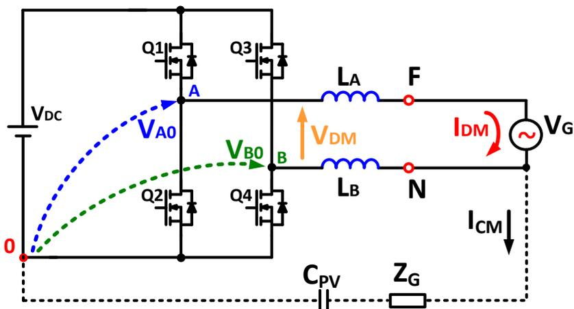
Figure 4.12 – Grid connected full bridge converter.
