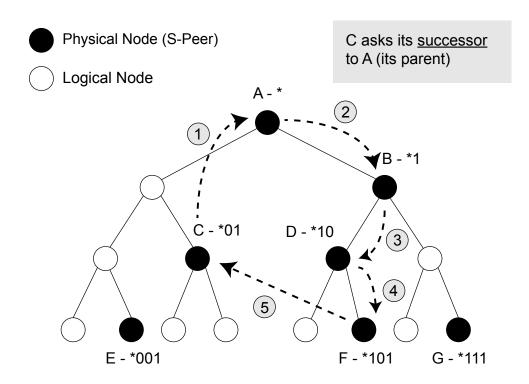
Figure 4.8: Finding the successor node in the ring by G-Grid structural links.
