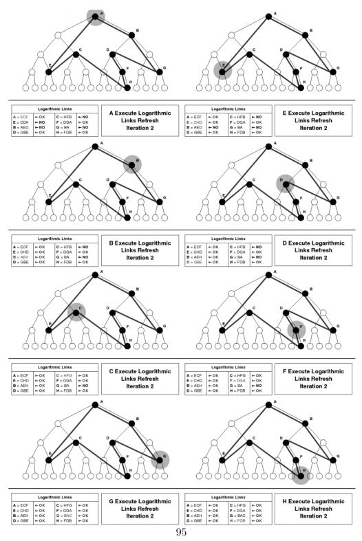
Figure 4.15: Example of logarithmic links construction – iteration 2.
