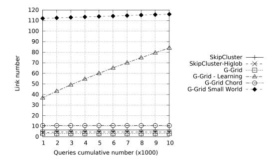
Figure 5.7: Number of links needed to maintain the overlay structure.
