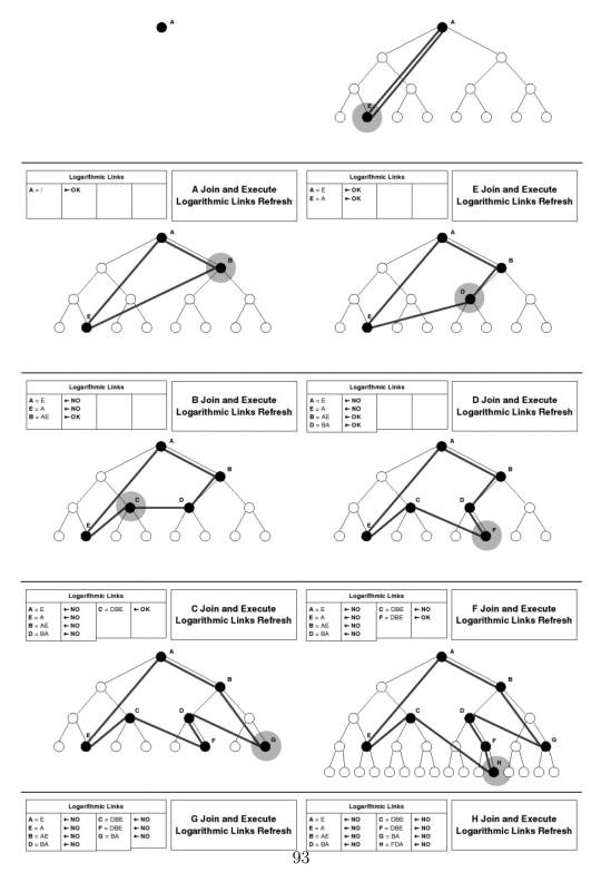
Figure 4.13: Example of logarithmic links construction – incoming peers.
