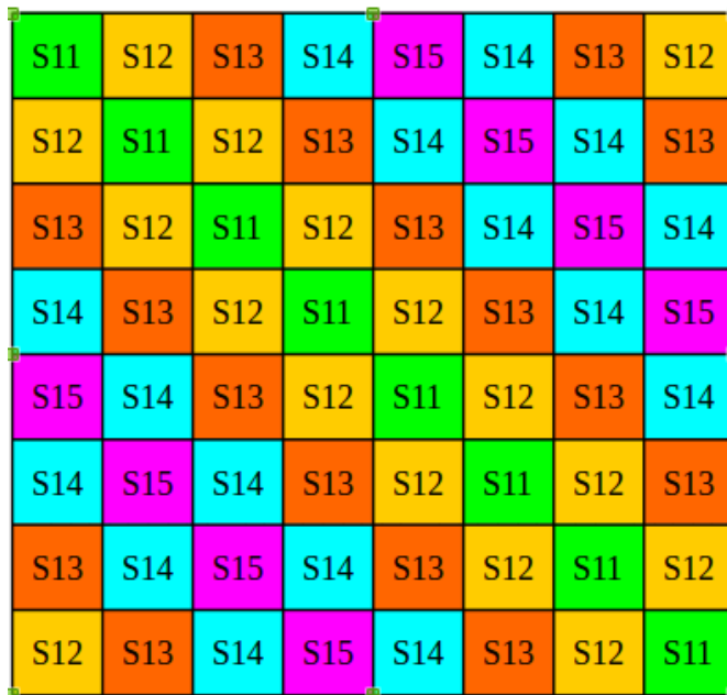
Figure 5.3: Independent elements in a multistatic central symmetric geometry with 8 antennas: each color represent a different element
