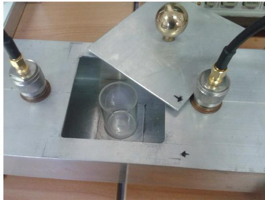
**Fig. 19 Square window for sample holder introduction.**
