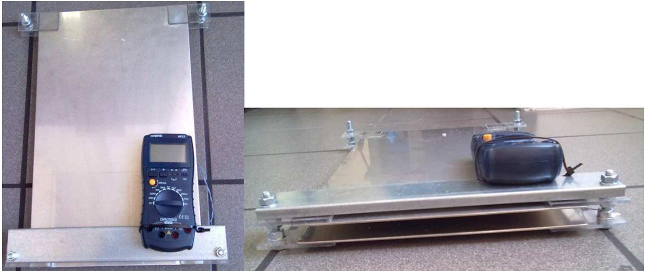
**Fig. 42 Parallel plate capacitor**
