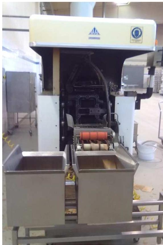
**Fig. 41** Cooking machine for wafer sheet.
