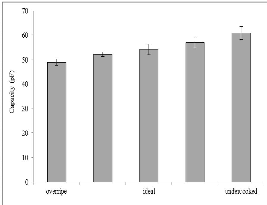
**Fig. 46** Capacitance values of one wafer sheet in function of the cooking level.
