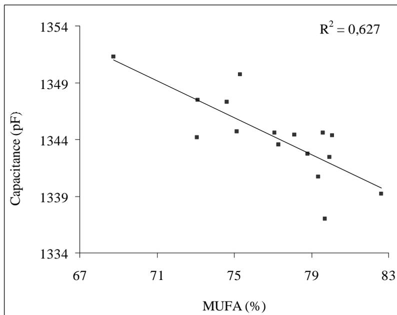
**Fig. 10 Correlation between capacitance and monounsaturated fatty acids (MUFA) for all oils at 2 kHz frequency.**
