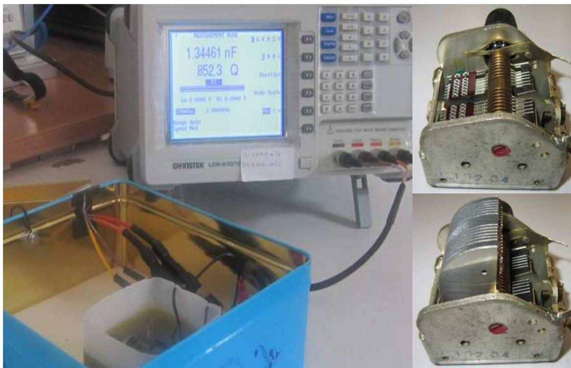
**Fig. 4 Instrumental chain and parallel plate capacitor with mobile and fixed plates.**
