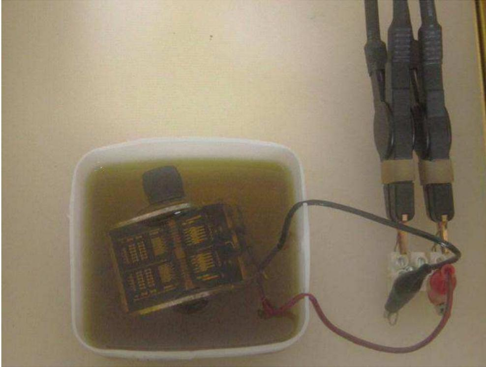
**Fig. 5 Parallel plate capacitor covered by EVOO sample.**
