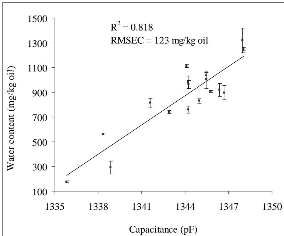
**Fig. 7 Correlation between capacitance and water content for all oils at 8 kHz frequency.**
