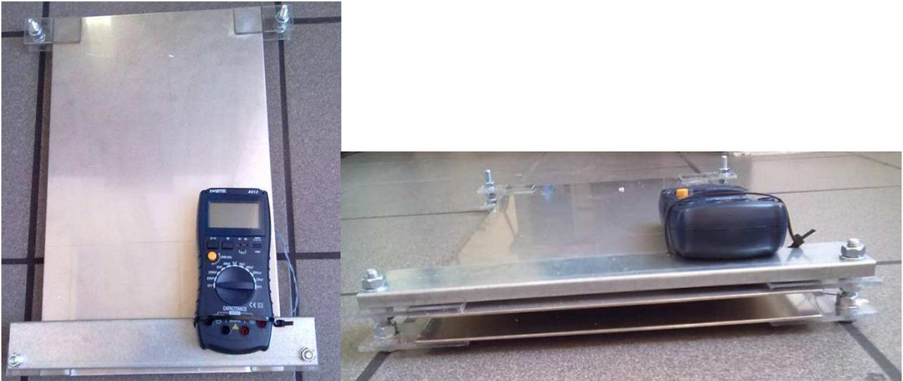
**Fig. 42 Parallel plate capacitor**
