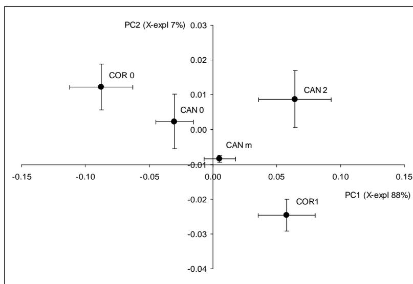
**Figure 39 Scores plot (mean values) for the first two principal components of the TDR acquisitions Horizontal and vertical bars are standard deviations respectively for PC1 and PC2.**
