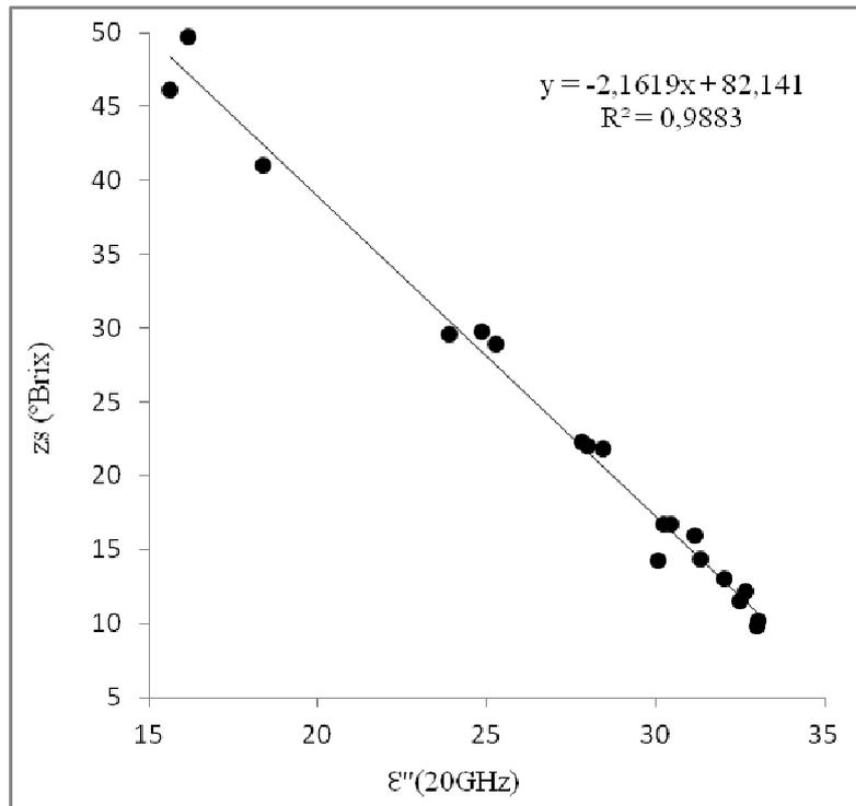
**Fig. 16 Correlation between solid soluble content and loss factor at 20 GHz.**
