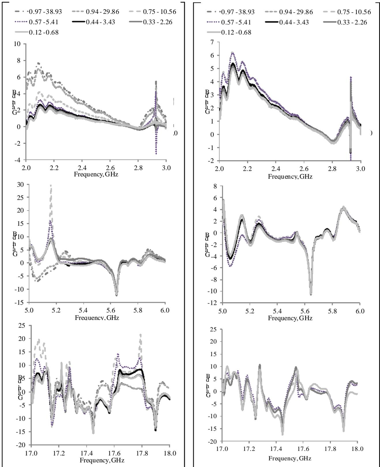
**Fig. 20** Acquired spectra for green (on the right) and roasted coffee (on the left) in the frequency range selected for water activity and moisture, 2-3, 5-6 and 17-18 GHz.
