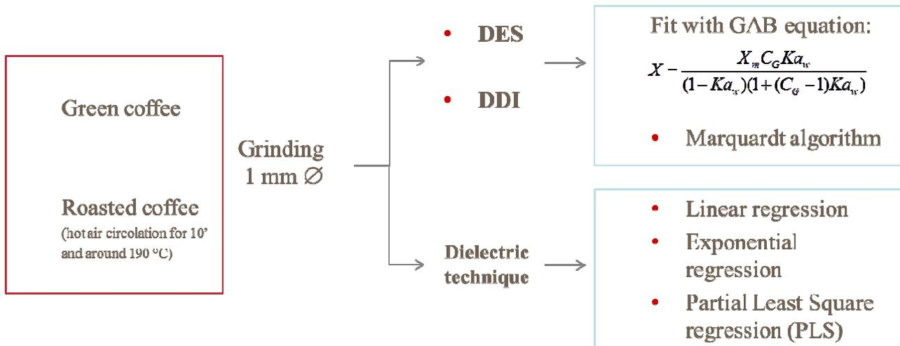
**Fig. 17 Experimental plan, DES (Saturated salt slurry method) and DDI (Dinamic Dewpoint Isotherm method)**
