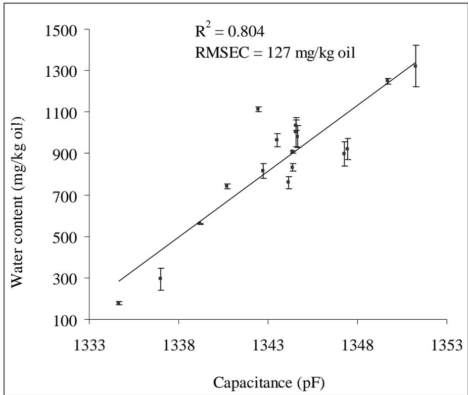
**Fig. 6 Correlation between capacitance and water content for all oils at 2 kHz frequency.**
