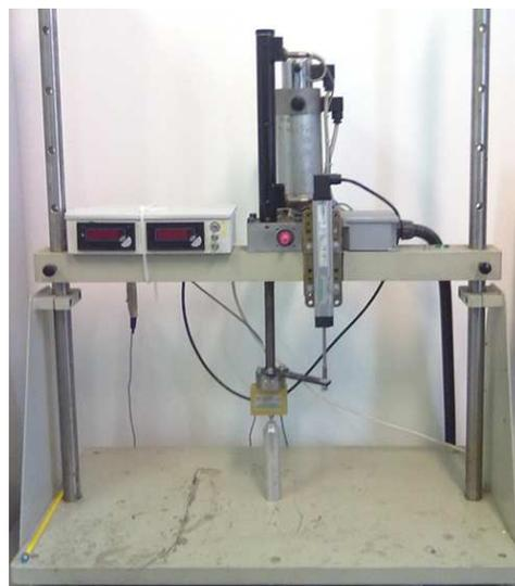
**Fig. 43 Compression device with cell of charge of 1 kg.**
