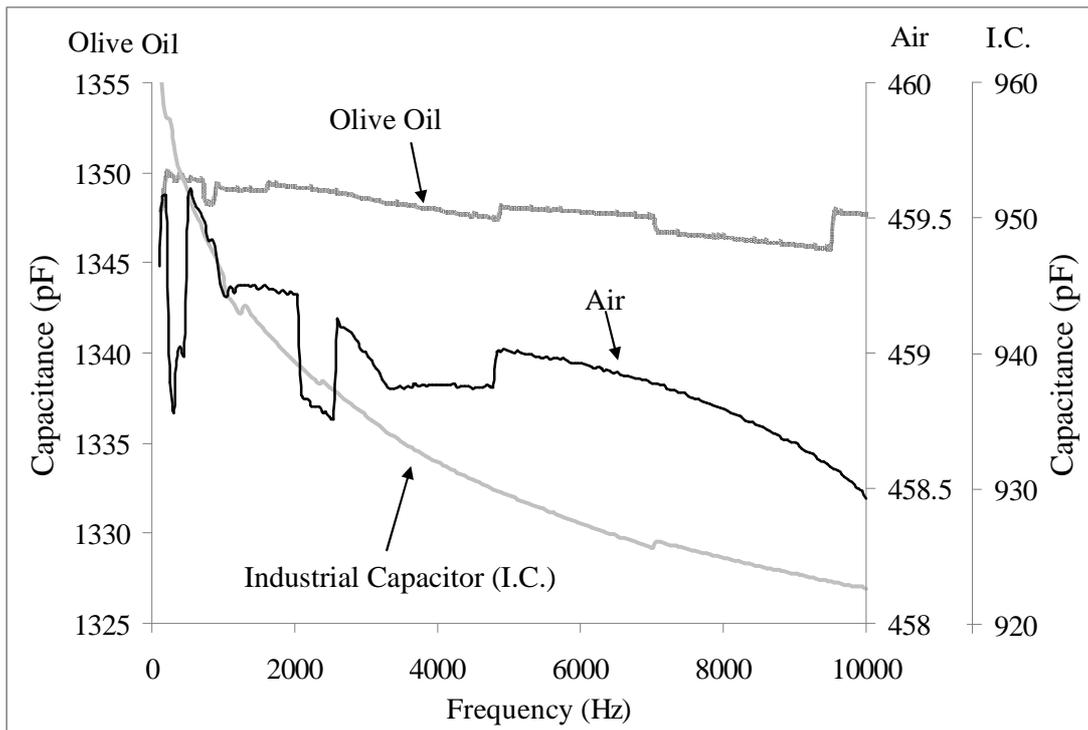
**Fig. 11** Capacitance for the probe in air and with an oil having a water content of 1321 mg/Kg oil (n. 12, in Tables 1 and 2), together with an industrial capacitor having a rated capacitance of 1 nF, in the range 100 Hz to 10 kHz.
