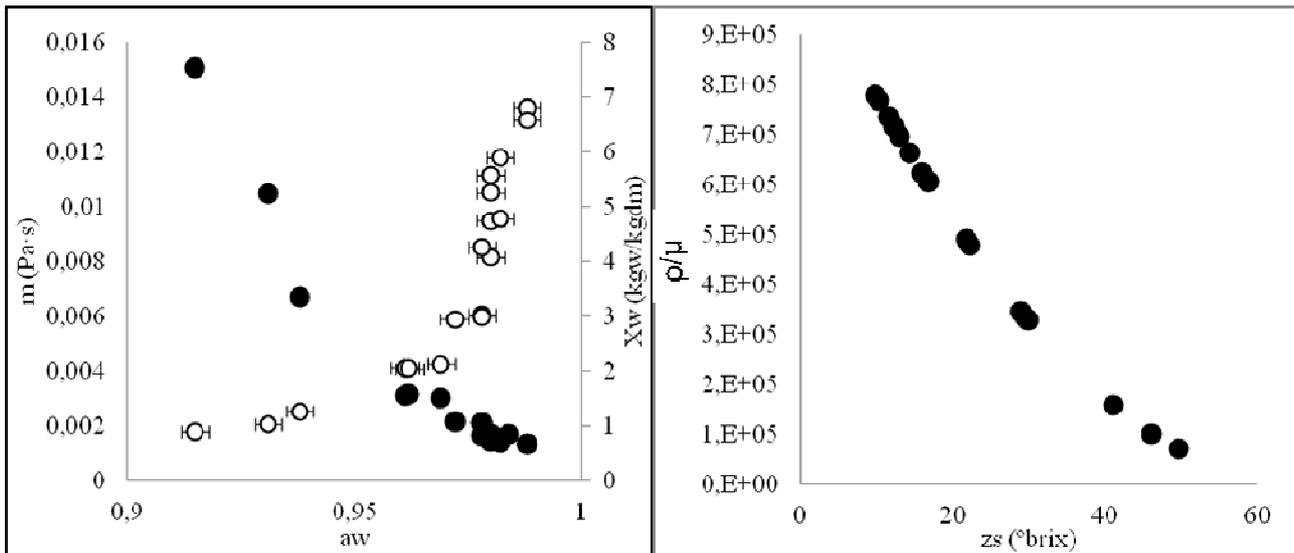
Fig. 13 Physical characterization during the concentration process, the empty dots represent the correlation between  $a_w$  and  $X_w$ ; the full dots show the correlation between  $a_w$  and  $m$ .
