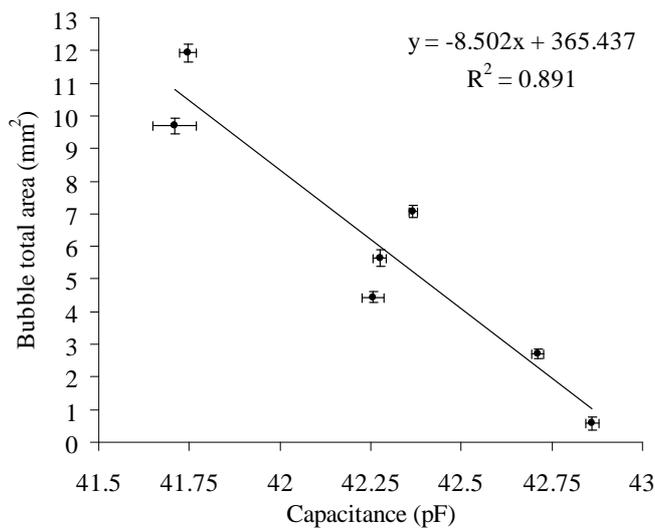
Fig. 37 Correlations between the capacitance and freezing process parameters (with standard error bars).
