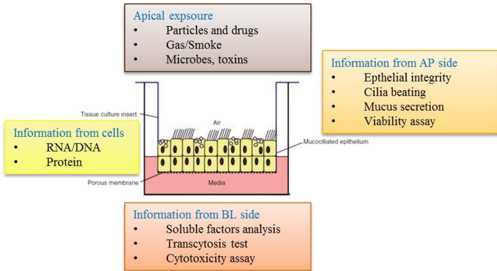
**Figure 3** Schematic of experimental output obtainable from a transwell-model of the respiratory epithelium
