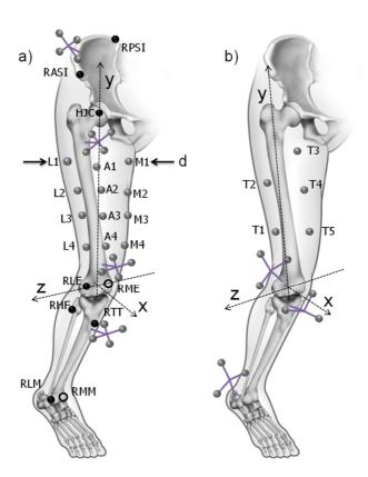
**Figure 3.1 -** *Ex-vivo* (a) and *in-vivo* (b) experimental set-ups. The pin-marker clusters, the skin-markers and the calibrated anatomical landmarks (black dots) are indicated. The specimens' maximum thigh diameter (d in Fig. a) and the thigh anatomical frames are also indicated.
