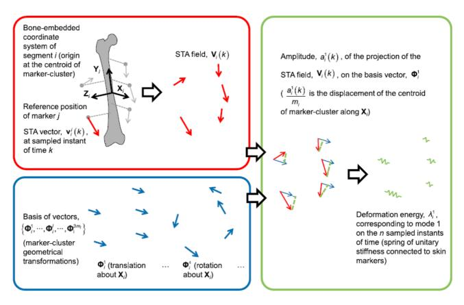
**Figure 4.1** – Framework of the generalized mathematical representation of the STA.
