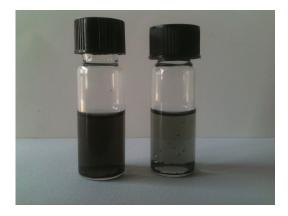
Figure 2.4: Picture of 1.SWCNT and 2.SWCNT before filtration.
