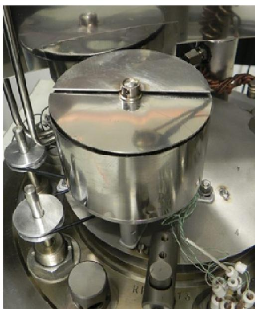
**Figure 1.3:** organic sublimation cells system with shutters.
