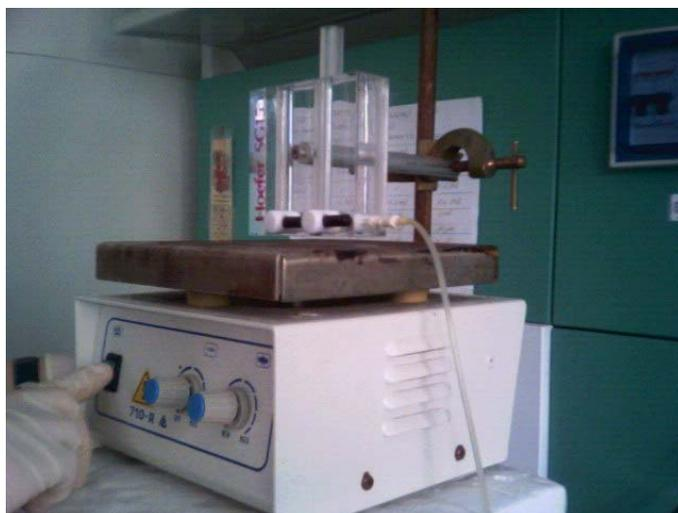
Fig. 3.2: The gradient maker used for BN polyacrylamide gel electrophoresis. The gradient maker is placed on a magnetic stirrer.
