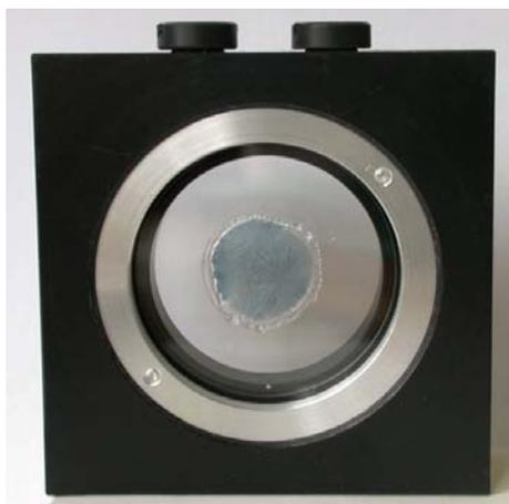
Fig. 3.5 A RC-trehalose matrix inserted into the gas-tight sample holder used in spectrophotometric measurements.
