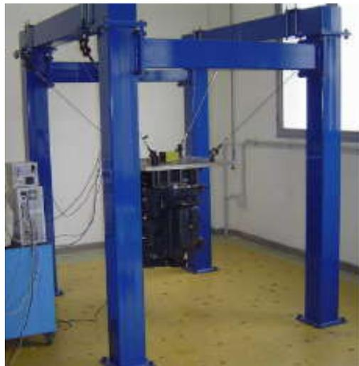
Figure 1.14: The InTensino test rig (built in 2002) for relatively compact rigid bodies up to 400 kg ([Gobbi et al. \[2011\]](#))
