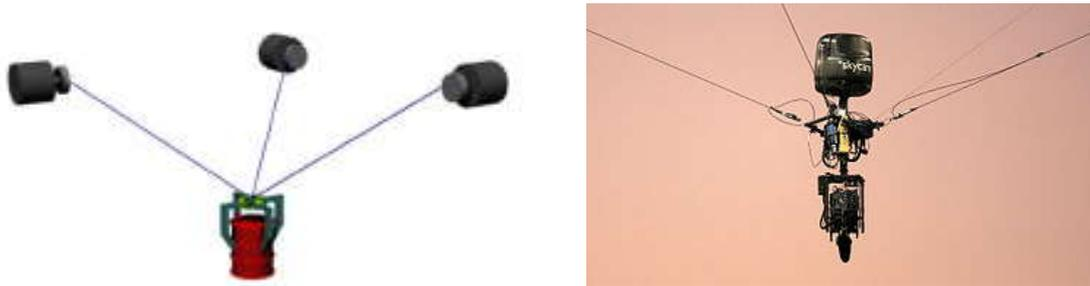
Figure 1.10: Examples of the point mass cable robot
