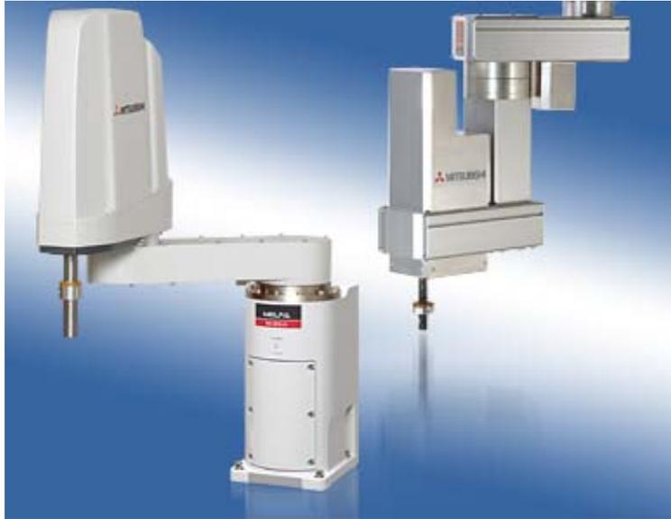
Figure 1.1: The SCARA robot, manufactured by MITSUBISHI (Mitsubishi [2013])
