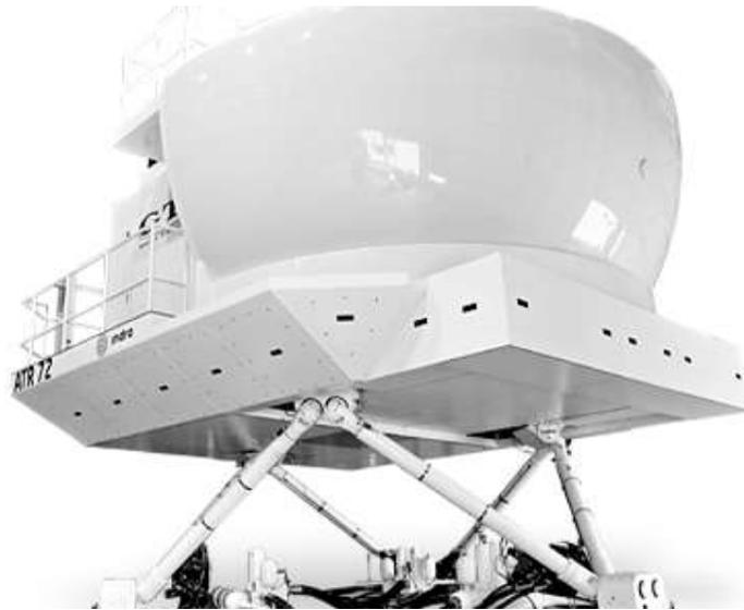
Figure 1.2: The Art 72-500 full flight simulator: an example of the Gough-Stewart platform ([Baltic Aviation \[2013\]](#))
