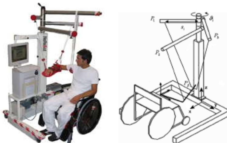
Figure 1.13: The NeReBot overall view and structural diagram (Rosati et al. [2007])
