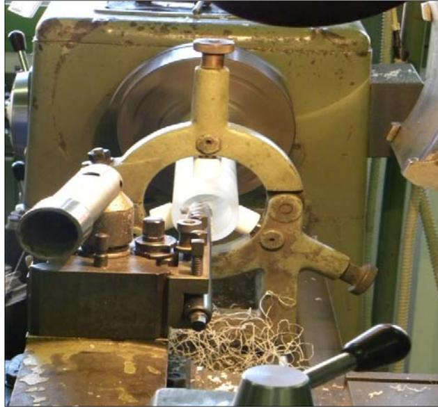
Figure 42: Realization of the rigid tube at the Hydraulic Laboratory of University of Bologna..
