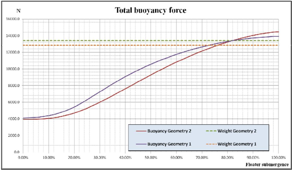
Figure 141: Trend of the buoyancy force for both geometries, the weight has been chosen in order to have the same buoyancy reserve force for both geometries.
