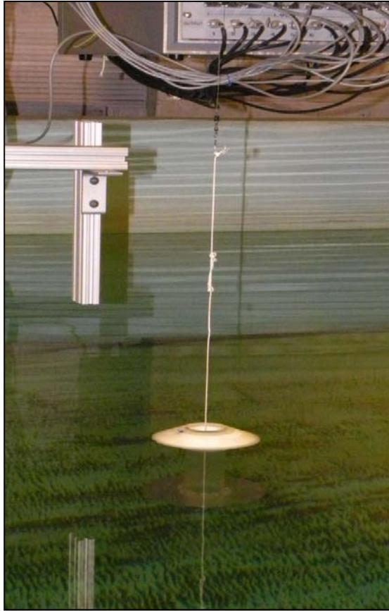
Figure 68: Displacements measuring method at Davidson Laboratory
