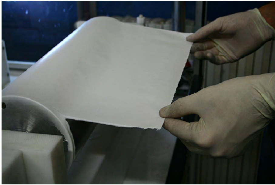
Fig. 4.2. Collecting the nanofibrous mat from the collector
