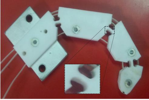
Figure 3.1: Mono-piece robotic finger employing SBFs [26]
