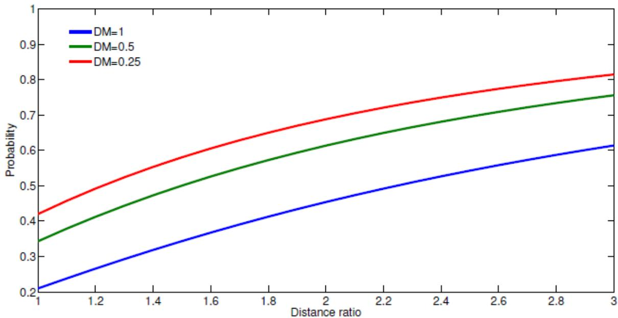
Figure 1: Probability that the peak ground acceleration (PGA) caused by an aftershock with magnitude  $M_0+DM$  is higher than the PGA caused by the mainshock with magnitude  $M_0$ , as a function of the distance ratio. The distance ratio is the ratio between the distance of the mainshock and the aftershock from the site.
