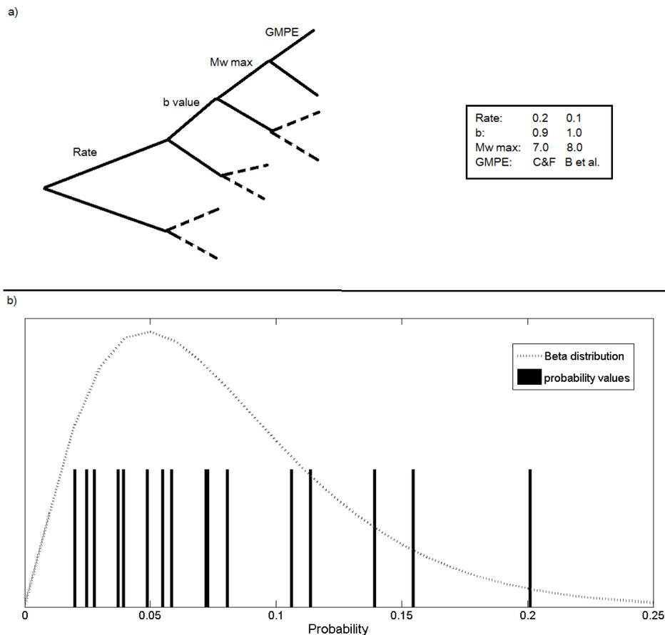
Figure 2. Panel a) logic tree of the seismic hazard example; panel b) the 16 values of the final branches of the logic tree and the Beta distribution made by these values.
