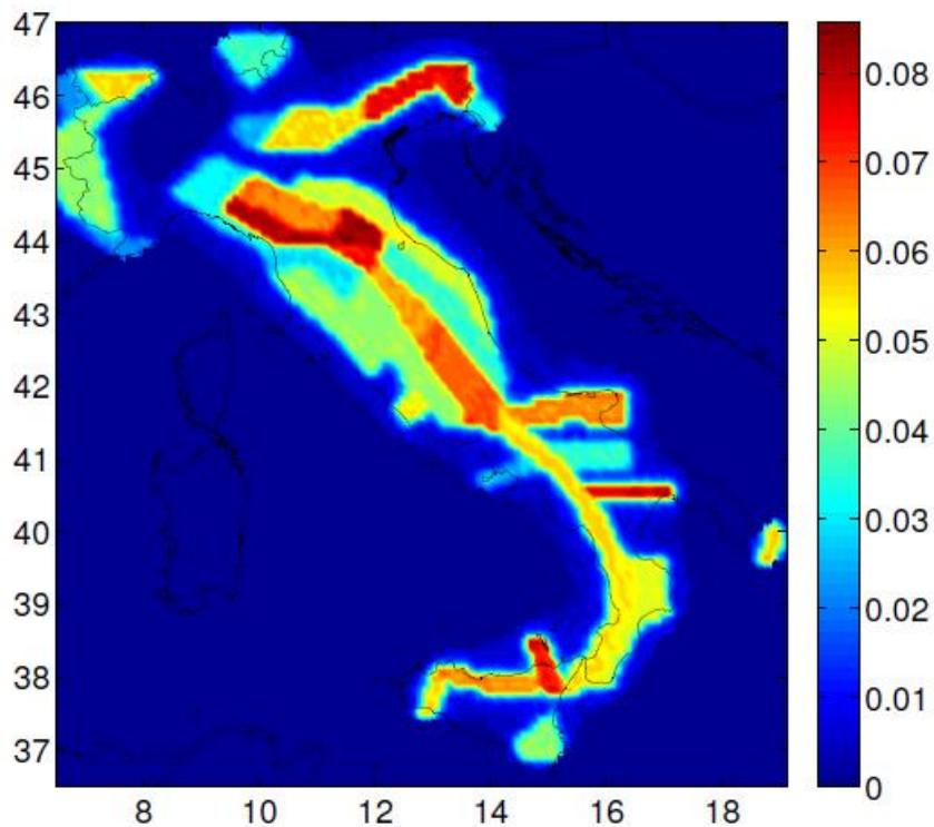
Figure 4: Differences between PGA values with exceeding probability of 10% in 50 years calculated with the corrected seismicity rates and with the declustered rates.
