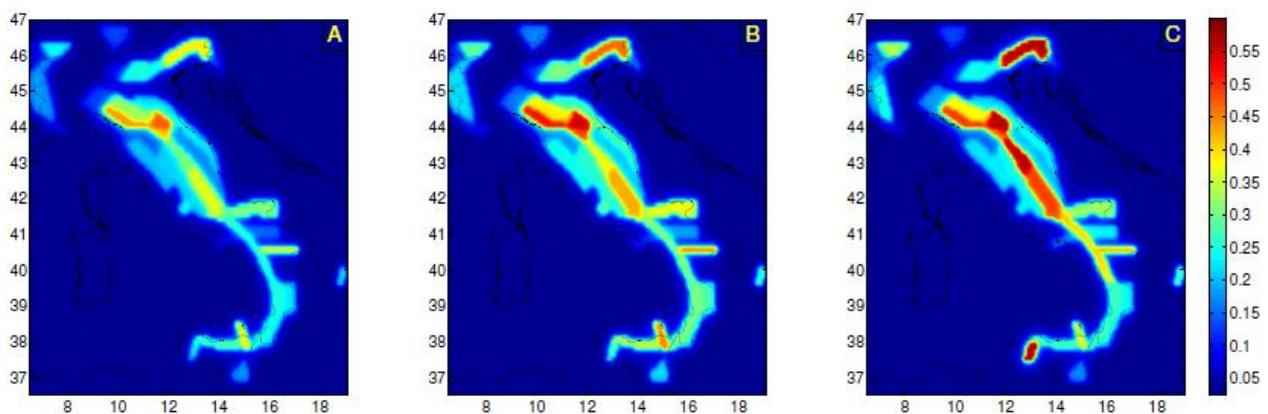
Figure 2: Seismic hazard map (10% of exceedance probability in 50 years) using (A) the declustered seismicity rates, (B) the corrected seismicity rates, and (C) the observed (undclustered) seismicity rates.
