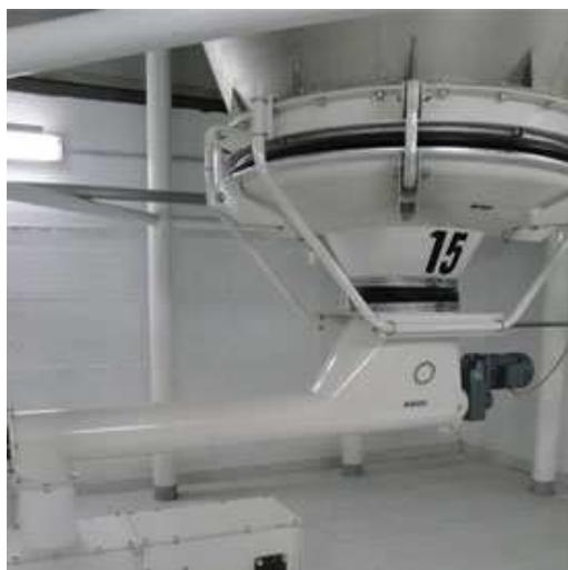
**Figure 4.** Automatic tubular screw conveyor for the dosing ingredients (Buhler, 2013)
