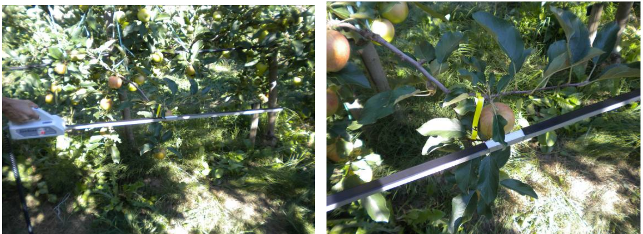
Fig. 6. a) Data collection using the ceptometer (left). b) Black tape used to allowed only 4-5-6 sensors for the readings (right).
