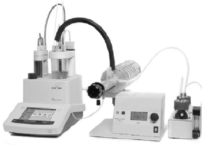
**Fig. 4.4 Karl Fischer system for water determination**
