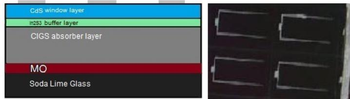
Figure 32: The structure of our CIGS thin film solar cell.
