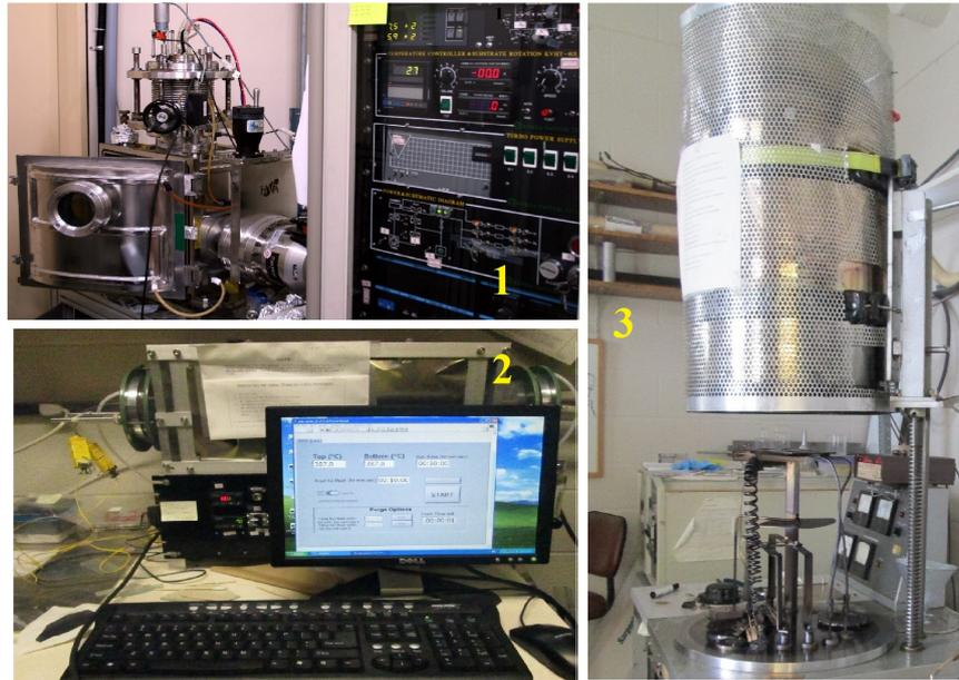
Figure 2: The three main step of CdTe deposition process; 1: R.F. sputtering machine, 2: activation chamber, 3: metallization bell.
