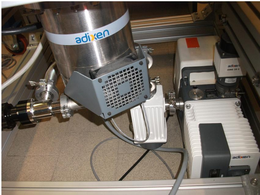
**Figure (2.7)** *Photo of the vacuum system assembled. A rotary vane pump (white) and a turbomolecular pump (grey) act in series to ensure the vacuum level required.*
