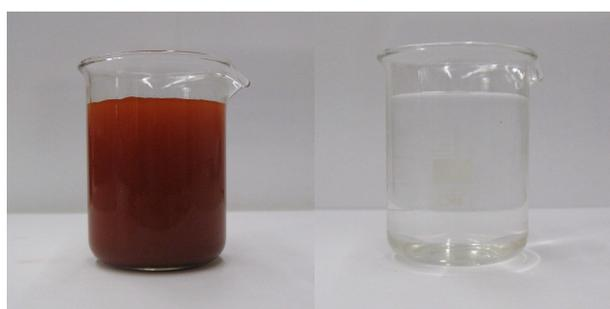
**Figure I.VI.** Sample of a water suspension of hematite #48100 before (left) and after (right) 10 minutes filtration in the wool magnetic filter.
