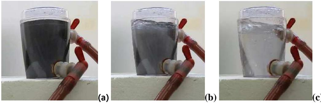
**Figure 4.2.c.** Pictures of the tank of setup #2 at the beginning of MACs filtration (a), after 10 seconds (b) and after 30 seconds (c).
