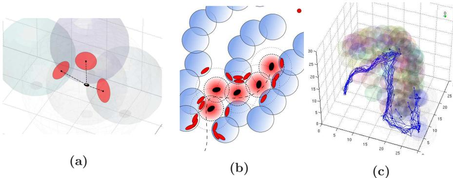
**Figure 5.4:** Each AUV, detecting an obstacle, creates a shared constraint that helps the other team-mates to find the best path, in order to achieve the final target.
