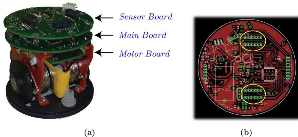
**Figure 8.1:** Prototype of the UniBot differential-wheeled mobile robot. In evidence the vertical bus on the main board's schema.
