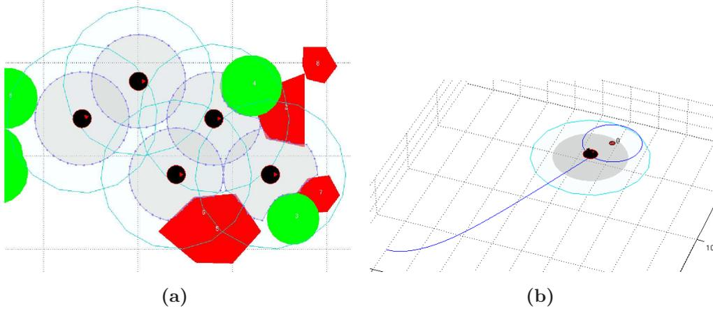
**Figure 6.3:** Obstacle detection is performed by sensors' device, providing the agent the possibility to perform obstacle avoidance while the agent is still computing the right control action to reach the final target. Notice that the sensor's area is clearly deformed by the presence of obstacles (6.3a).
