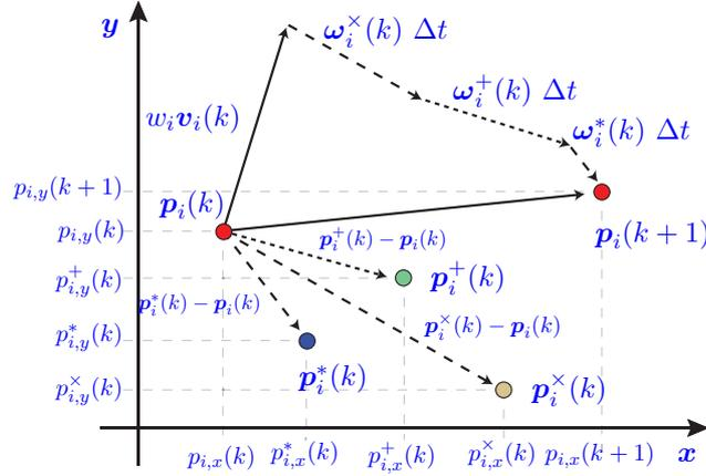
**Figure 3.3:** Original PSO algorithm applied to particles moving in a 2D environment.
