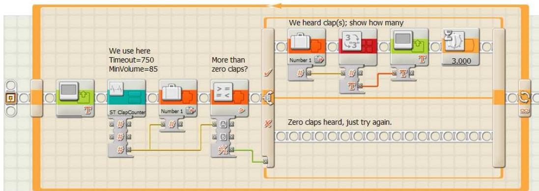
**Figure 7.6:** Screenshot from LEGO Mindstorms NXT-G programming interface.
