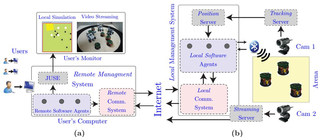
**Figure 8.3:** Scheme of the UniBot Remote Laboratory: Remote Management 8.3a and Local Management System 8.3b.
