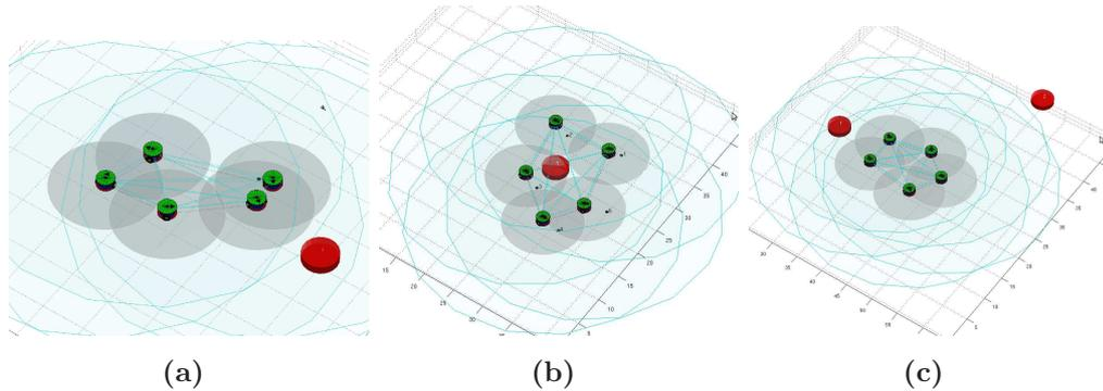
**Figure 6.7:** The soft formation control is performed by robots in order to avoid obstacles and remain connected.
