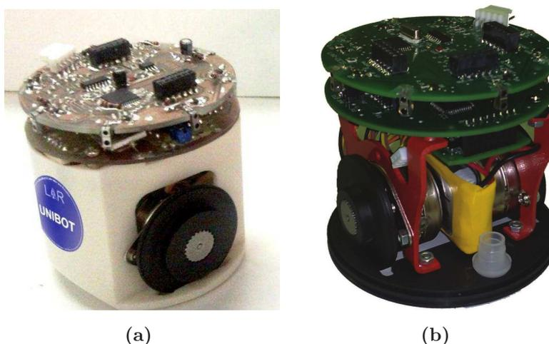
**Figure 7.1:** The prototype version (left) and the first full-functional version of Unibot  $V_1$  (right) have been the inspiration for designing the later version.
