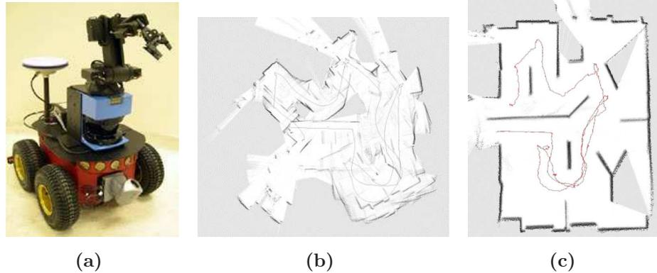
**Figure 2.7:** The 4 wheeled mobile platform Pioneer 3-AT, endowed with laser-scanner, GPS device, video-camera, robotic griper, ultrasonic sensors, is one of the best platforms used to study mobile robotics. By exploiting the laser scanner it is possible to build an environmental map (2.7b) which needs a post elaboration in order to be usefully exploited (2.7c).
