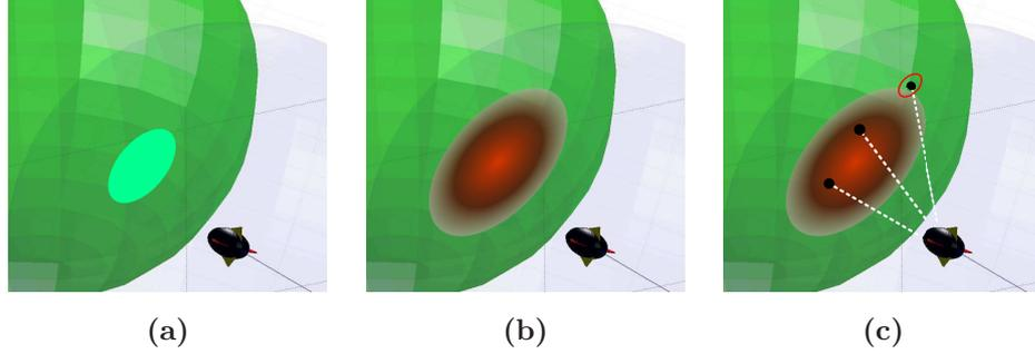
**Figure 5.3:** A circular collision area is produced when an AUV detects an obstacle (5.3a), such as the related virtual patch (5.3b) created as constraint, in the search space. Each virtual patch is defined by a 2D-Gaussian probability distribution that helps  $\mathcal{SA}^{oav}$  in the computation of  $PSO^{oav}$ .
