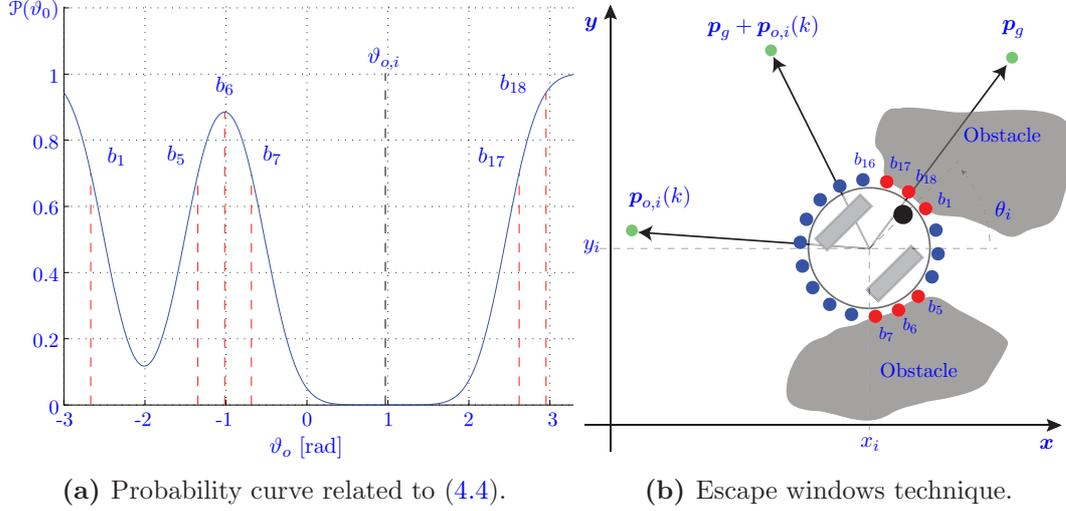
**Figure 4.3:** Example of escape window computed by considering obstacles detected by bumpers  $\{b_{17}, b_{18}, b_1\}$  and  $\{b_5, b_6, b_7\}$ .
