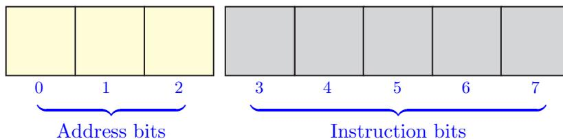
**Figure 8.2:** Byte command structure.
