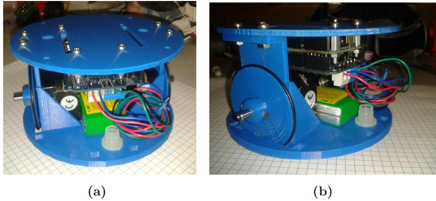
**Figure 7.4:** Frontal and lateral view of the A-Unibot chassis.
