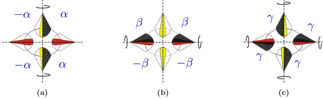
**Figure 5.2:** Rear view of the AUV with directional fins in  $\alpha, \beta, \gamma$  configurations.
