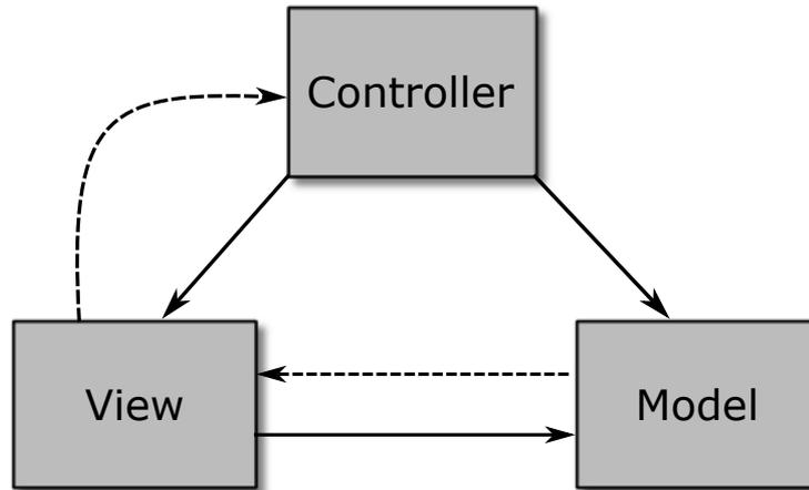
**Figure 9.2:** The Model-View-Controller Pattern Diagram.
