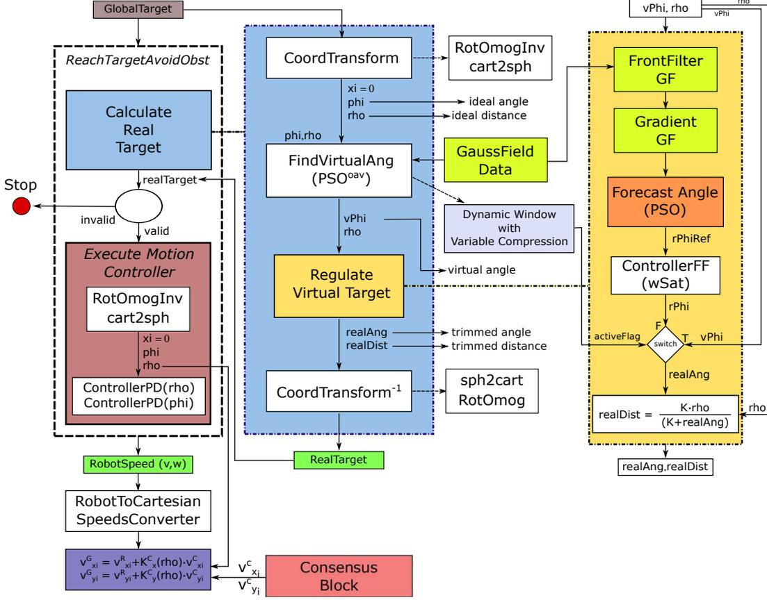
**Figure 6.6:** The global control scheme of the algorithm, from the robot’s (agent’s) point of view, is useful to better understand all the operations computed by the control system. Moreover it is possible to understand the interconnections between “classic” and modern control techniques as PSO and Consensus.
