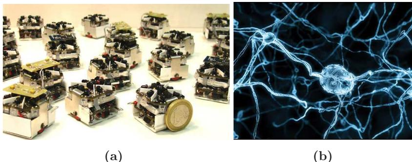
**Figure 2.13:** Alice (2.13a), developed at EPFL, is one of the most used mini-robots in the world. A very little area is large enough for the mobile robotics techniques applications that involve this robot model, because its dimensions are 2x2x2 cm. However the frontier of the robot dimensions' reduction process is in the nano-scale robotics. A futuristic vision of the nano-bots technology as substitution of neurons 2.13b may be representative of the future.
