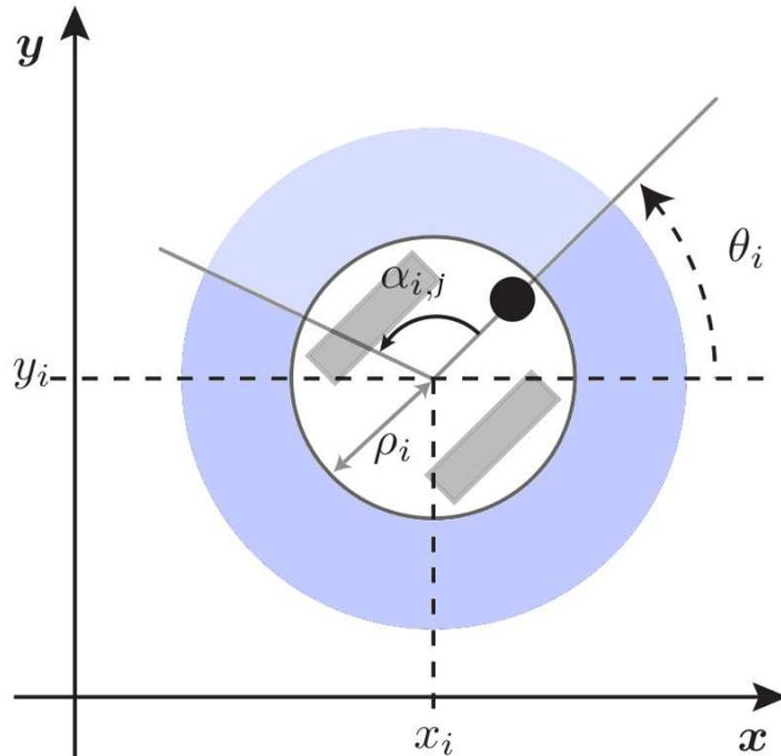
**Figure 6.1:** Kinematic model of the robots with the state variables. The blue ring represents the sensor's area defined by the 36 proximity sensors equally spaced around the robot, whose sensible distance and quantization can be freely configured. The parameter  $\alpha_{i,j}$  defines the angle of the  $j^{th}$  sensor.
