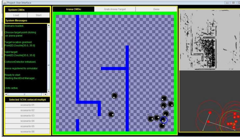
**Figure 9.1:** A screenshot of JUSE during a simulation in one of the maze-like scenario.
