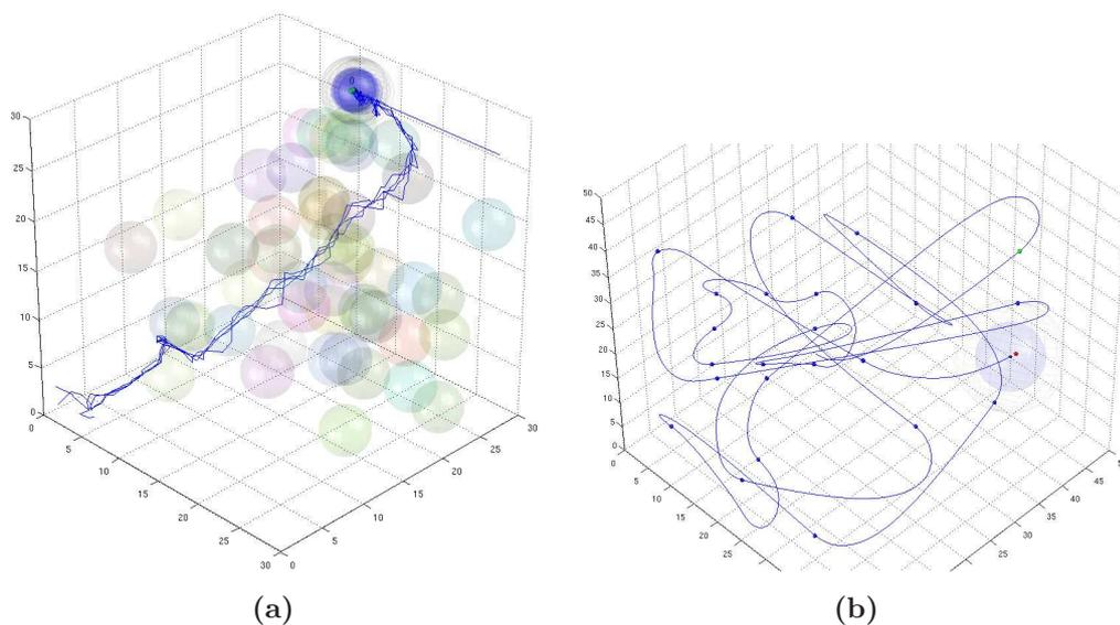
**Figure 9.7:** Simulations are fundamental for testing the designed techniques. A 3D simulation, on which the PSO technique presented in Chp. 4 is running, is depicted in 9.7a. Many simulation have been done in order to test AUV's behaviour and its orientation capability. One of this tests is shown in 9.7b.
