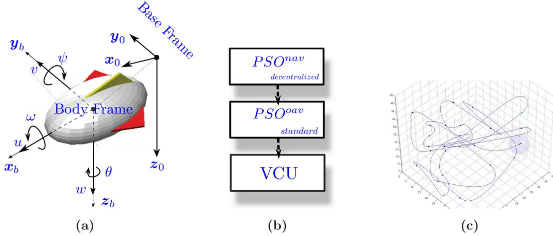
**Figure 5.1:** In order to define AUV's movements and to follow way-points, two different reference frames are needed, namely the Body and the Base Frame. By exploiting VCU's input variables, PSO control algorithm is able to change the AUV's attitude and speed, providing underwater navigation.
