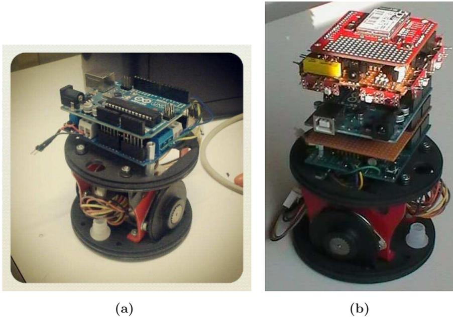
**Figure 7.3:** The A-Unibot prototype chassis with the main board (left) and the complete prototype equipped with a custom DIY square sensor board and the WiFi device.
