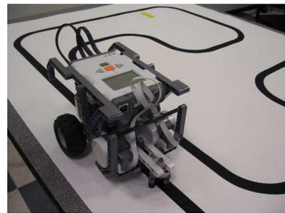
(f) A line-follower application developed with a NXT differential wheeled robot.
