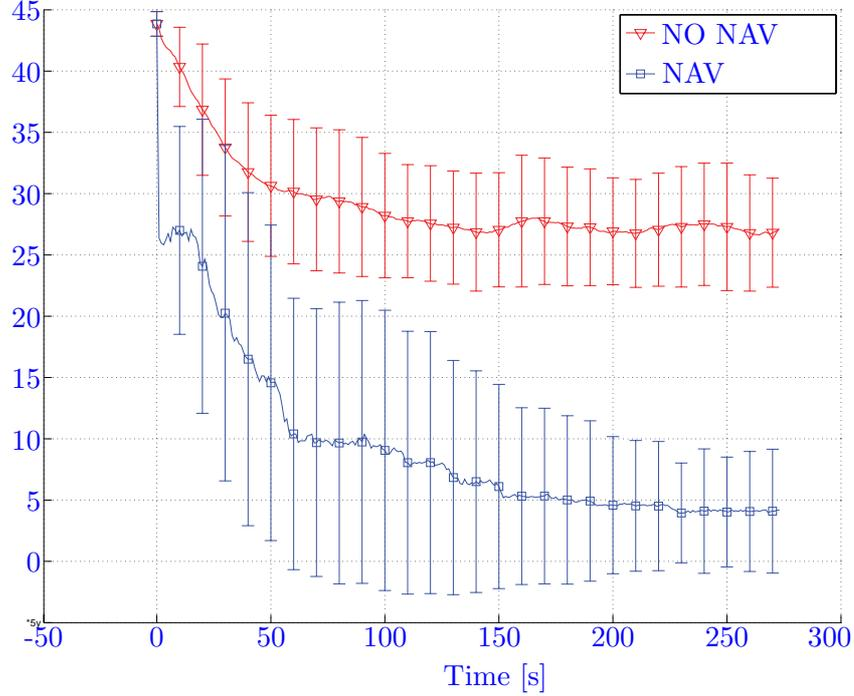
**Figure 4.4:** MSE and STDEV of distance error between each robot’s position and the goal both with and without NAV. Data gathered over 20 simulations on Scenario 3.
