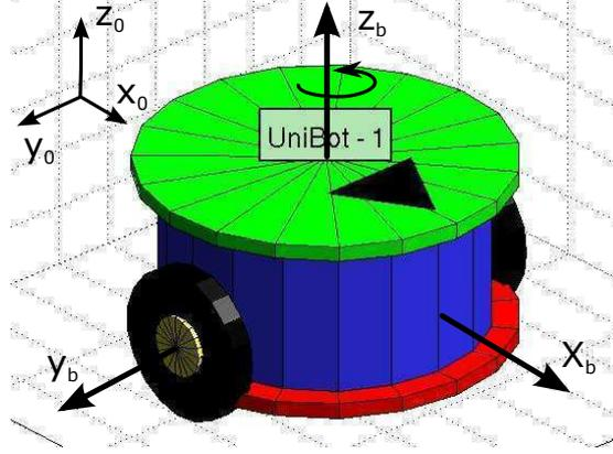
Figure 6.2: The base  ${}^oF$  and the body  ${}^bF_i$  frame.
