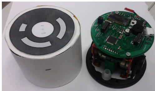
(a) The Unibot markers exploited by the system to recover the robot’s positions inside the arena.
