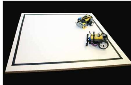
(d) A Sumo ring where the robots are controlled by a RCX brick.
