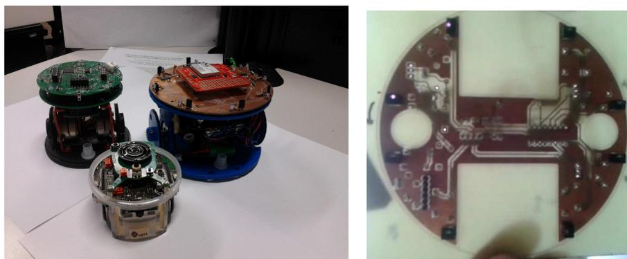
**(a)** A mobile robot comparison between Unibot  $V_1$ ,  $V_2$  and E-puck.
