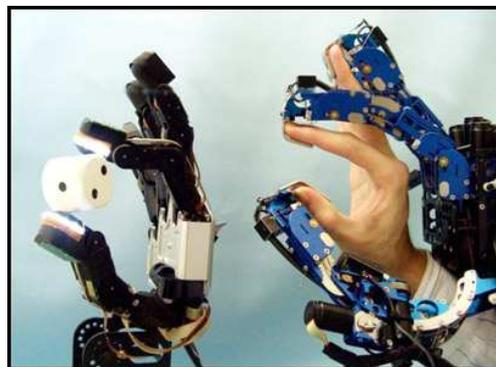
**Figure 2.3:** An haptic glove useful to remotely control a proper robotic hand.
