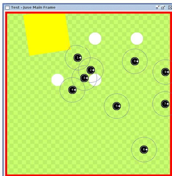
**Figure 9.3:** A top view of the simulated arena where a swarm of robots is performs a task. The depicted white circles are environmental obstacles, the yellow square a coloured area only. The obstacle detection performed by J.U.S.E. is based on the colours detected below the sensible area. This way it is quite simple to define if a coloured area is an obstacle or not.
