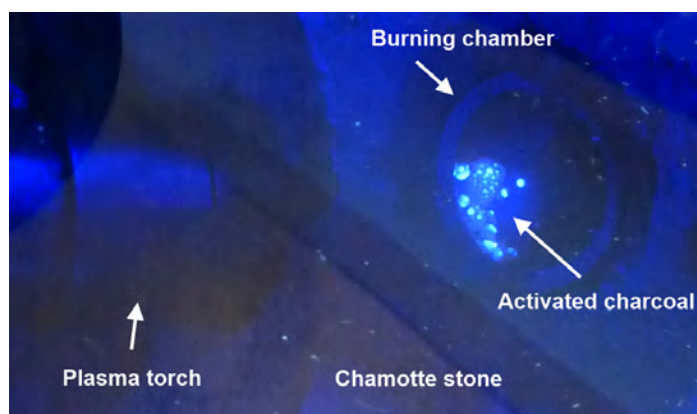
Figure 5.16: Photograph during burning of charcoal as viewed through a colored cobalt glass.
