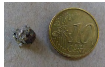
Figure 5.18: Treated mixture of glass particles and brazen chipping.
