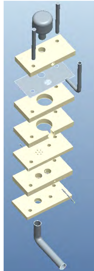
Figure 5.12: First design of a modular laboratory device with several combustion chambers. The fire bricks can be assembled in various ways for different experiments.
