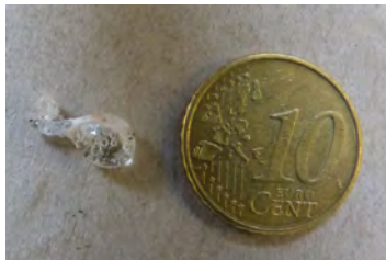
Figure 5.17: Treated mixture of glass particles and combustible waste. On the top of the glass droplet some dirt spots can be seen.
