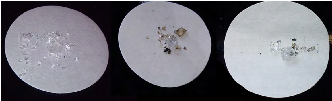
Figure 5.19: The sample on the left pictures the untreated sample. The second is the glass treated for 20 seconds and the third picture is the glass treated for 50 seconds. For comparison, the diameter of the filter paper is 30 mm.
