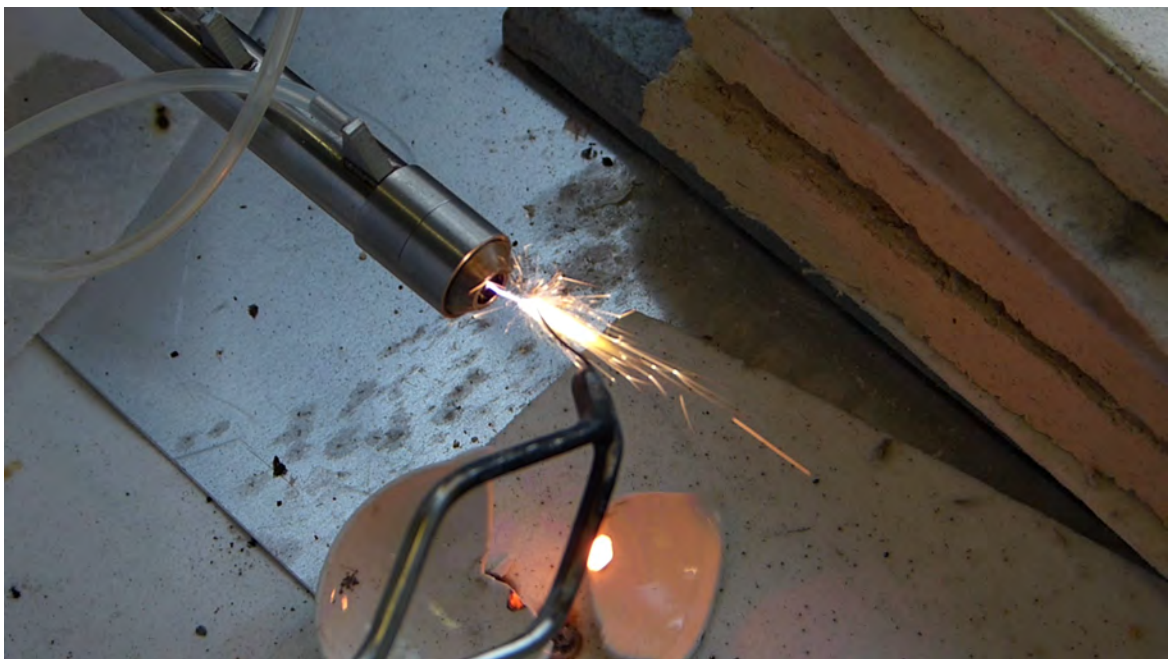
Figure 5.22: Capture of a metal droplet breaking the ceramic cup
