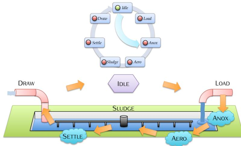
Figure 5.8: An idealised sketch of a Waste-Water Treatment Plant operated with a Sequencing Batch Reactor.
