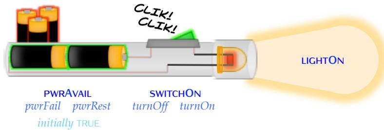
**Figure 2.4:** A simple flashlight with batteries, a switch and a led diode to project light and the EVENT CALCULUS terms to represent it.
