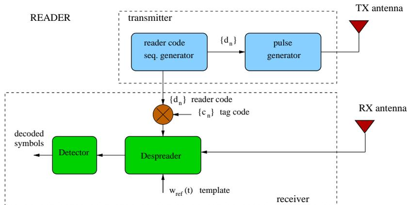
Figure 6.6: UWB reader architecture in backscattering schemes [271].
