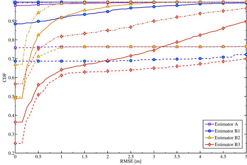
Figure 5.8: c.d.f.s of the RMSE. Dashed lines (--) refer to the absence of relays, continuous lines (—) refer to the presence of JF relays, dot-dashed lines (·-) refer to the presence of AF relays.
