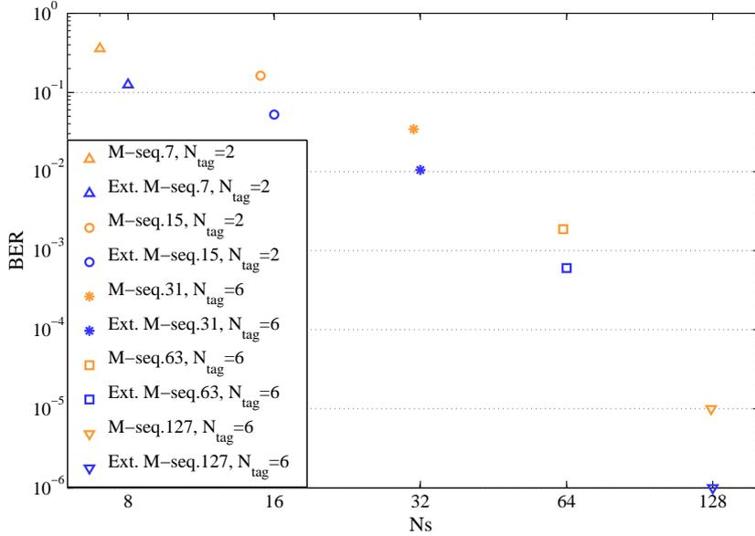
Figure 7.4: BER vs  $N_s$  in multi-tag laboratory environment and asynchronous scenario.
