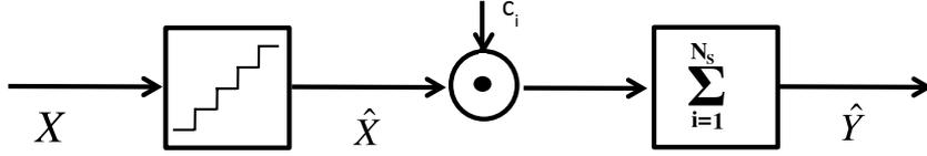
Figure 8.8: The considered scheme for the ADC and de-spreader.
