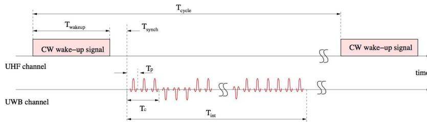
Figure 6.10: UHF-UWB interrogation cycle.
