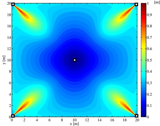
Figure 9.6: Configuration #5. PEB considering 1 transmitter in  $[10, 10]$ , and 4 receivers at the corners (multistatic).
