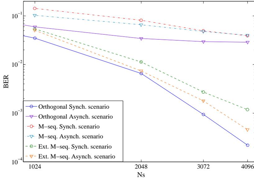
Figure 7.5: BER vs  $N_s$  in multipath 802.15.4a CM1 channel.
