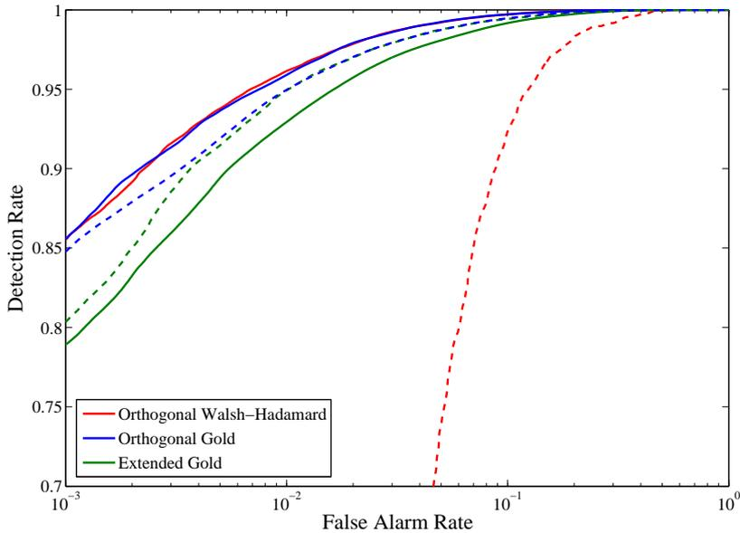
Figure 8.4: ROC for the tag detection in UWB backscatter system. Continuous lines (—) refer to the perfectly synchronous scenario, dashed lines (---) refer to the asynchronous scenario due the presence of clock drift, with ideal code phase retrieving.
