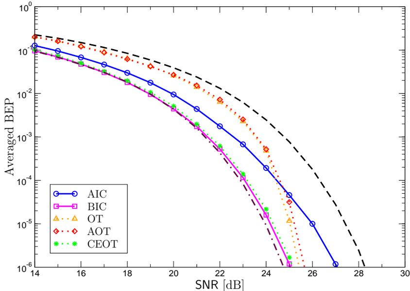
Figure 2.11: Performance of the SaG-AcR with different bin selection strategies. Continuous lines (—) are for the blind selection strategy. Dotted lines (· ·) are for the threshold-based strategies with  $\tilde{k} = 10$ . Dashed line (--) is for the conventional AcR. Dot-dashed line (- ·) is for the SaG-AcR with optimum threshold and prior parameter knowledge (ideal receiver).
