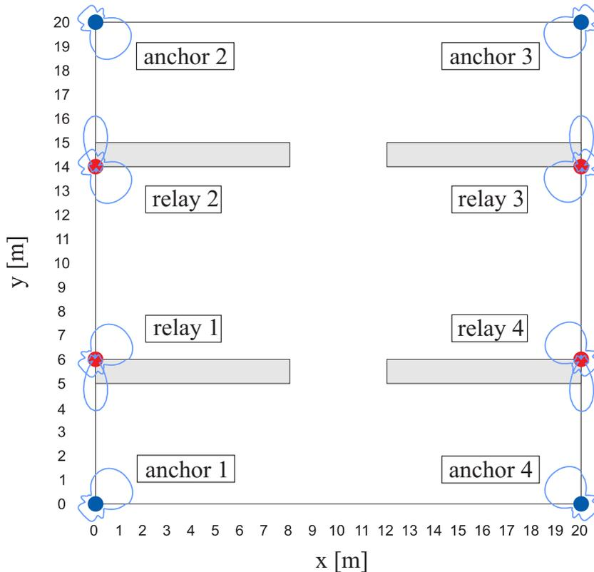
Figure 5.4: Scenario considered in the simulation results. Blue points refer to anchors. Red points refer to relays. Antennas' radiation patterns and orientation are reported. Obstacles are depicted in grey.
