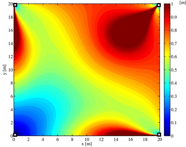
Figure 9.5: Configuration #4. PEB considering 1 transmitter, in  $[0, 0]$ , and 4 receivers at the corners (multistatic).
