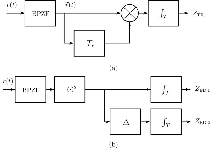
Figure 2.1: Conventional non-coherent receivers. (a) AcR. (b) EDR.
