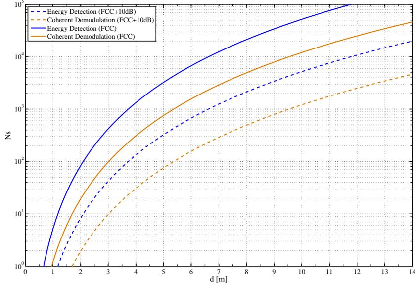
Figure 8.3: Minimum number of pulses per symbol as function of the reader-tag distance.
