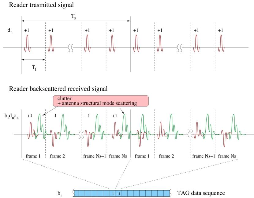
Figure 6.8: Backscatter modulation.
