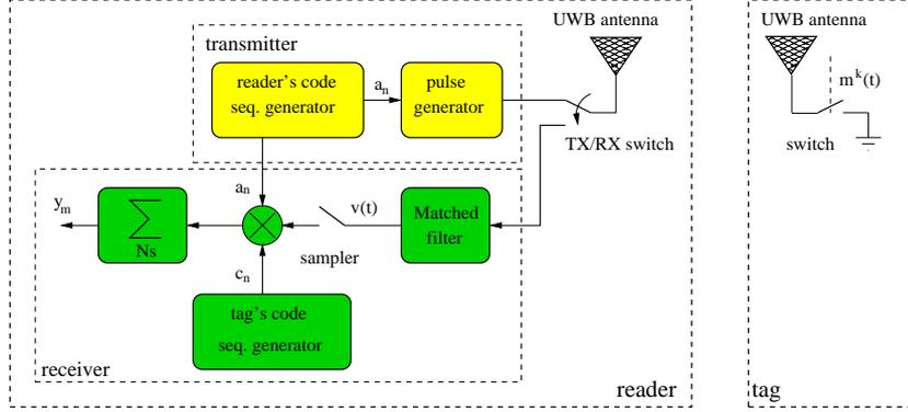
Figure 7.1: The considered scheme of the tag and the reader composed of a transmitter and a receiver section.
