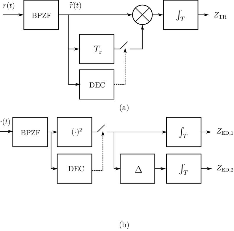
Figure 2.2: Stop-and-go receivers. (a) SaG-AcR. (b) SaG-EDR.
