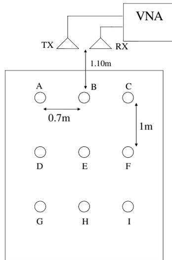
Figure 7.3: Indoor scenario considered for the measurement campaign at ENSTA-ParisTech.
