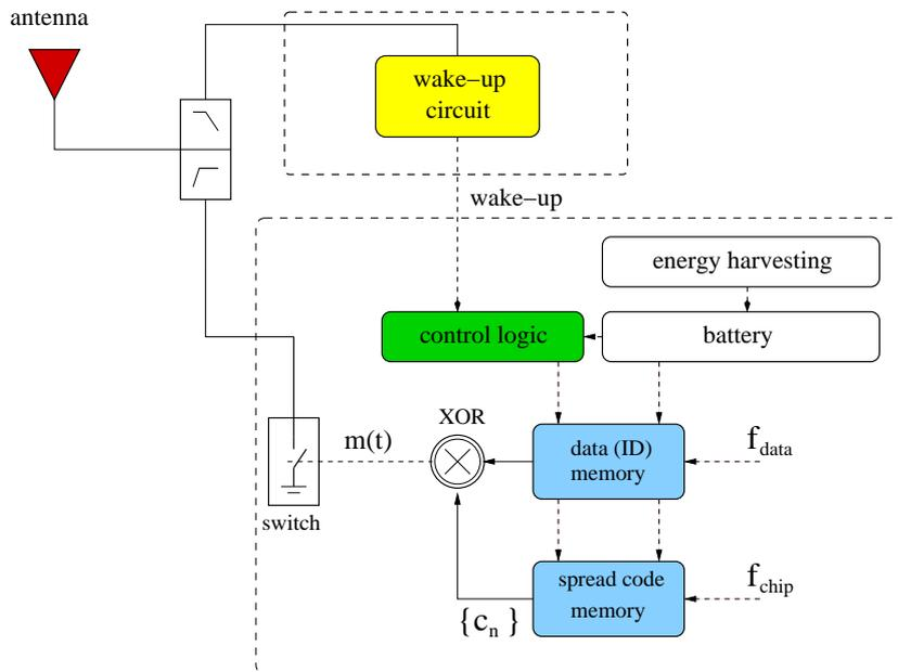
Figure 6.7: UWB tag architecture in backscattering schemes [271].
