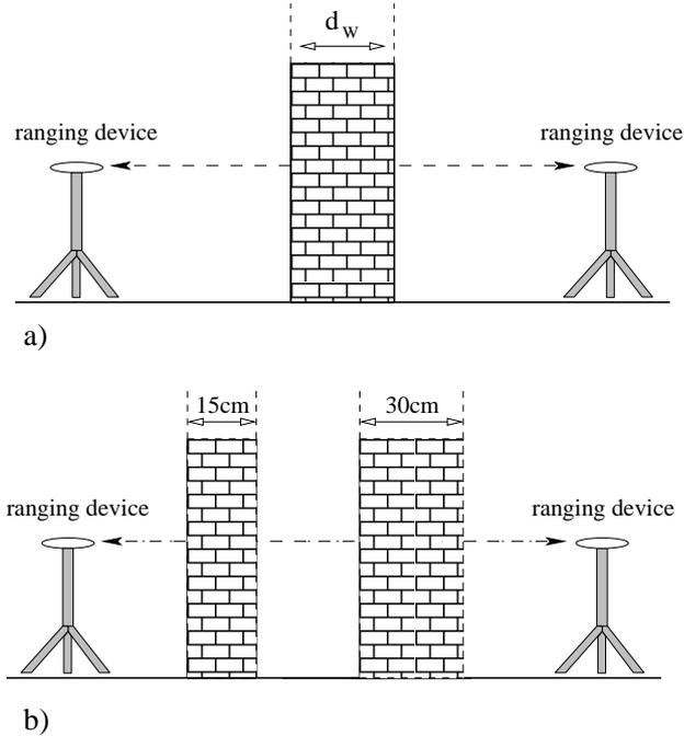
Figure 4.5: Obstacles characterization setup [228].
