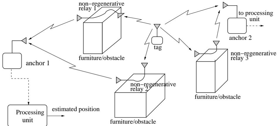
Figure 5.1: Example of localization system employing non-regenerative relays.
