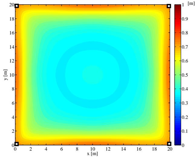
Figure 9.2: Configuration #1. PEB considering 4 reference nodes (transceivers) at the corners (monostatic).
