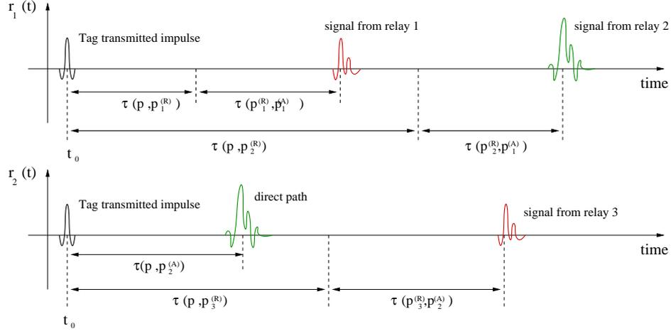
Figure 5.3: Example of signal structure in a scenario adopting active tags.  $\delta^{(R)} = 0$ .  $r_1(t)$  and  $r_2(t)$  are the signals received by anchors 1 and 2, respectively.
