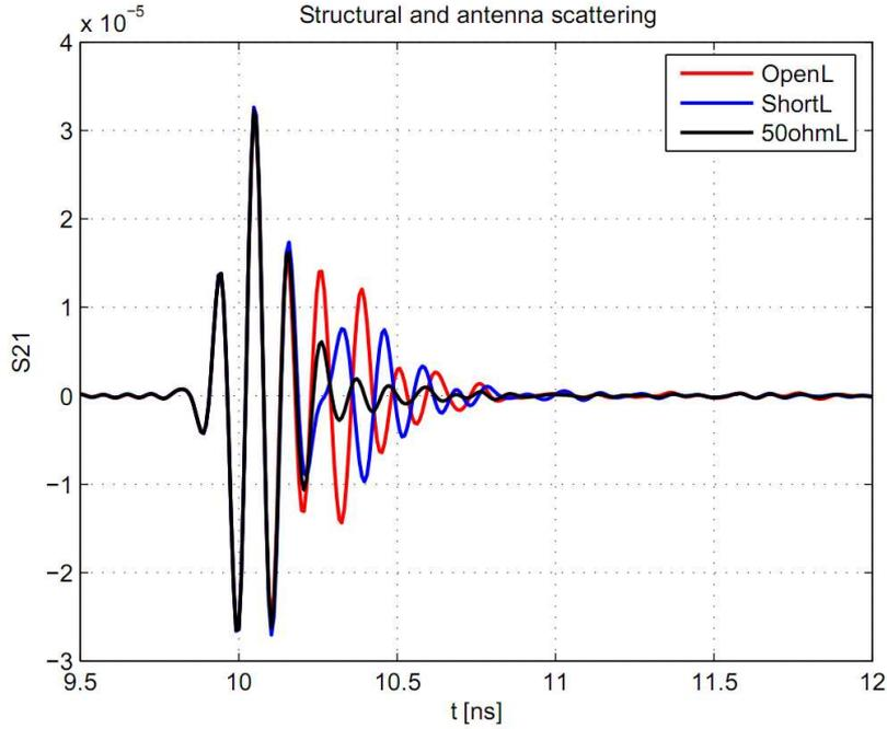
Figure 6.3: Example of backscattered signal, for three tag load impedance values (free space).
