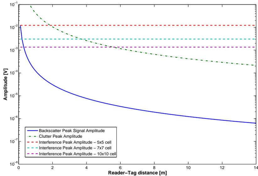
Figure 8.6: Typical dynamic range of a UWB-RFID system.
