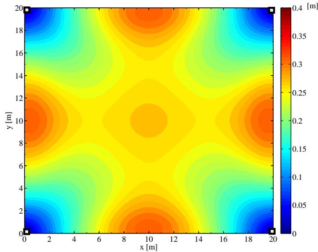
Figure 9.3: Configuration #2. PEB considering 4 reference nodes (transceivers) at the corners, each processing the signals of every transmitter (multistatic).
