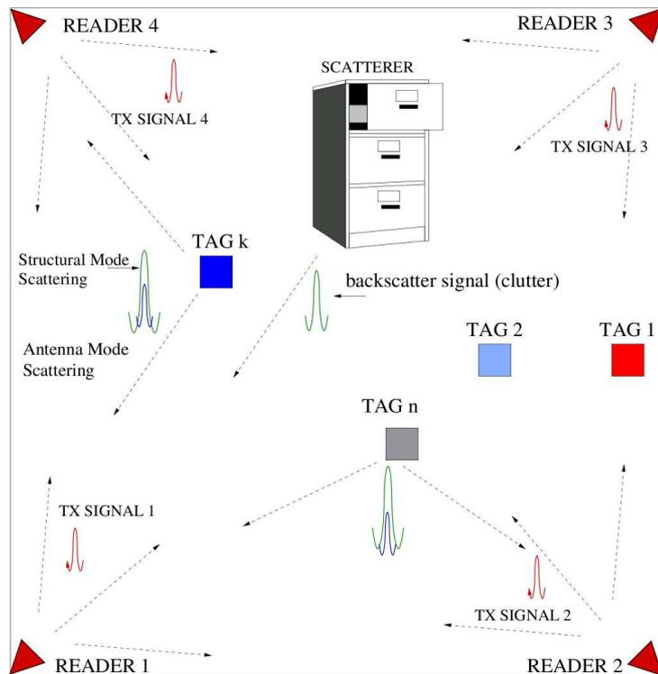
Figure 6.2: Example of a square cell monitored by four readers.
