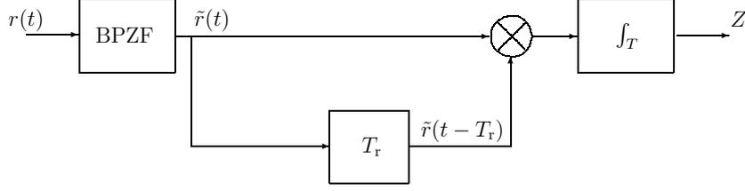
Figure 1.1: Conventional autocorrelation receiver.
