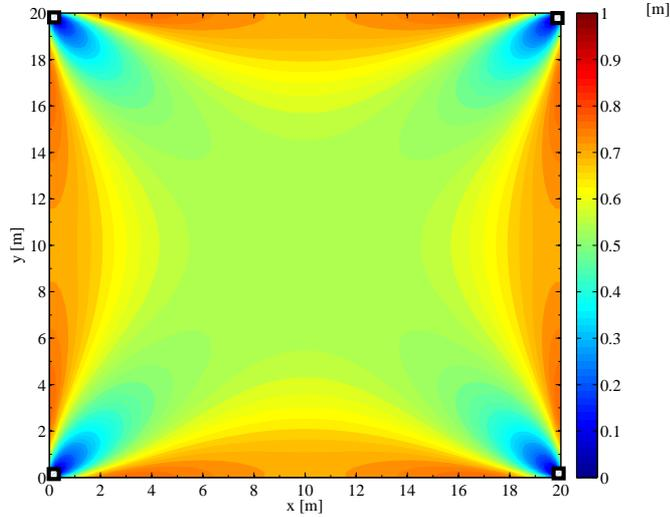
Figure 9.4: Configuration #3. PEB considering 2 transmitters in  $[0, 0]$ ,  $[20, 20]$ , and 2 receivers in  $[20, 0]$ ,  $[0, 20]$  (multistatic).
