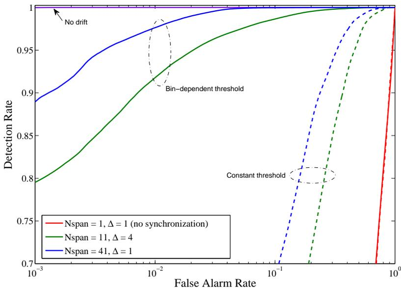
Figure 8.5: ROC for tag detection in presence of synchronization offset, clock drift and near-far interference effects. Continuous lines (–) refer to the bin-dependent threshold, dashed lines (– –) refer to the constant threshold.
